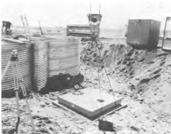
FIGURE 2.9a. Installation of In-Situ Monitoring Test Site. Background shows large buried caissons used for evaluating fluid and radionuclide flux. Foreground shows partial installation of a weighing lysimeter used to evaluate energy and mass balance parameters which control the rate of migration of radionuclides through the geologic media.
