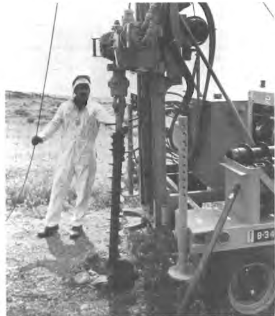
FIGURE 2.8. Core Drilling Apparatus Used for Taking Partially Disturbed Sediment Cores at Radioactively Contaminated Burial Trenches.
