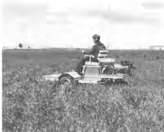
FIGURE 2.7a. Transducer Vehicle with Ground Penetrating Radar Unit and Telemetry System Used to Collect Data Concerning the Morphology and Contents of Waste Burial Structures.
