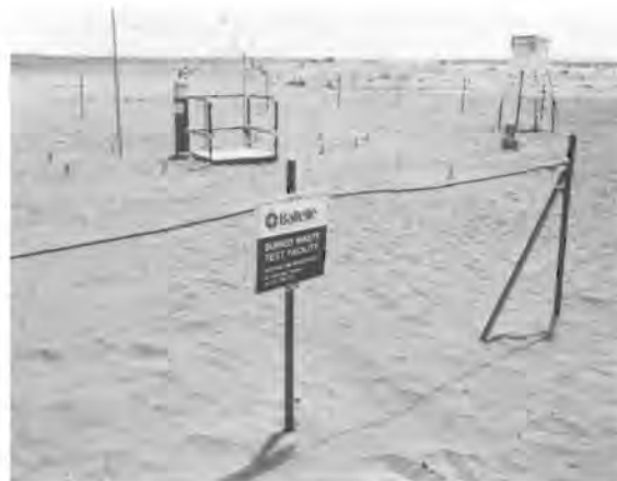
FIGURE 2.9b. Post Installation After Burial and Back-fill of Items Shown in Figure 2.9a. Neutron monitoring access wells and micrometeorological instruments are shown.
