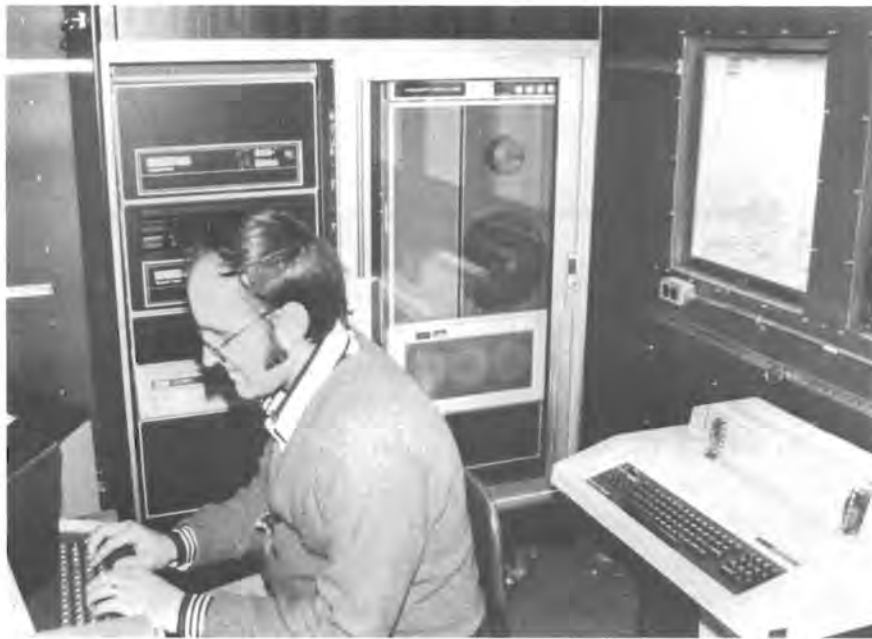
FIGURE 2.7b. Data Processing Vehicle with Computer and I/O Devices Used to Process and Analyze Data Telemetered from the Geophysical Transducer Vehicle.
