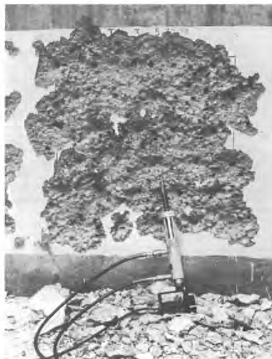
FIGURE 2.10. 3 ft x 3 ft Test Panel After Spalling with Hand-Held Hydraulically Actuated Split-Wedge Spalling Tool.
