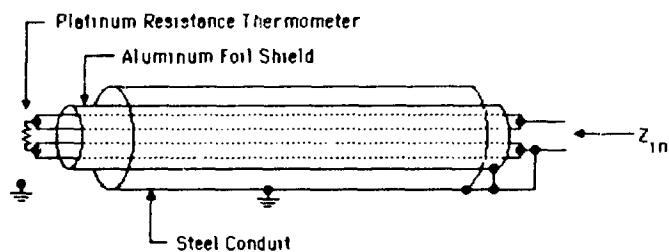
From the Model, the Transfer Function of the Cable can be calculated and the Cable Effects can be compensated for
