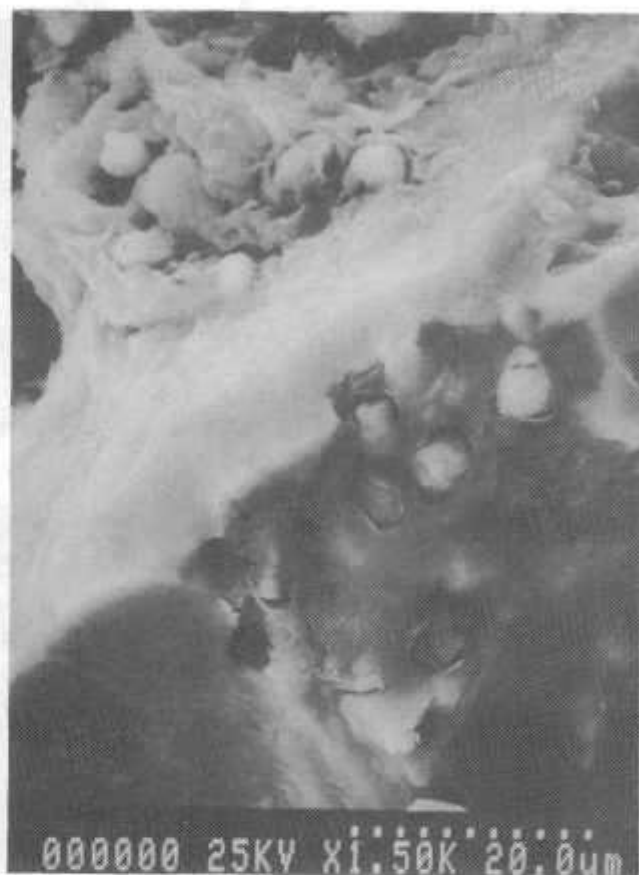
(b) Authigenic magnesite crystals growing in pits of surface of authigenic quartz crystal, suggesting that magnesite precipitation occurred after, or perhaps in conjunction with, corrosion of the quartz. (Scale bar = 20 \mu m)
