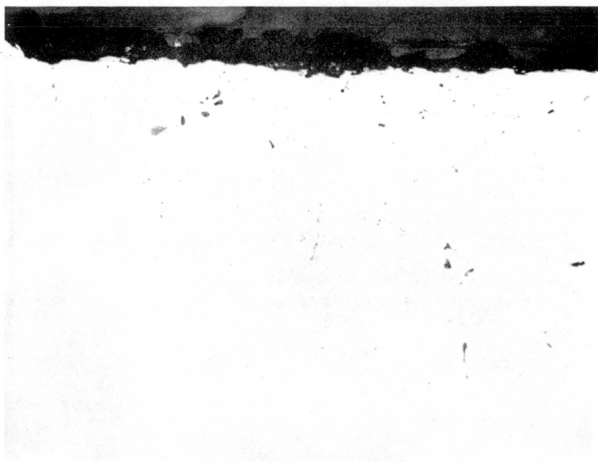
FIGURE 2 - A typical portion of the titanium edge after being in contact with ^{238}\text{PuO}_2 for 720 days at 800^\circ\text{C} showing the irregular edge and subsurface reaction product (as polished, 125X).
