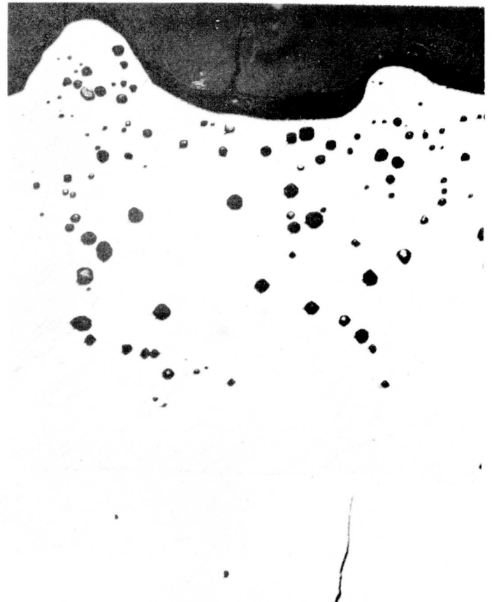
FIGURE 10 - Same as Figure 2 but etched to reveal acicular structure. Etchant: 5 to 7 ml Hf, 2 to 4 ml \text{HNO}_3 , 100 ml \text{H}_2\text{O} (250X).
