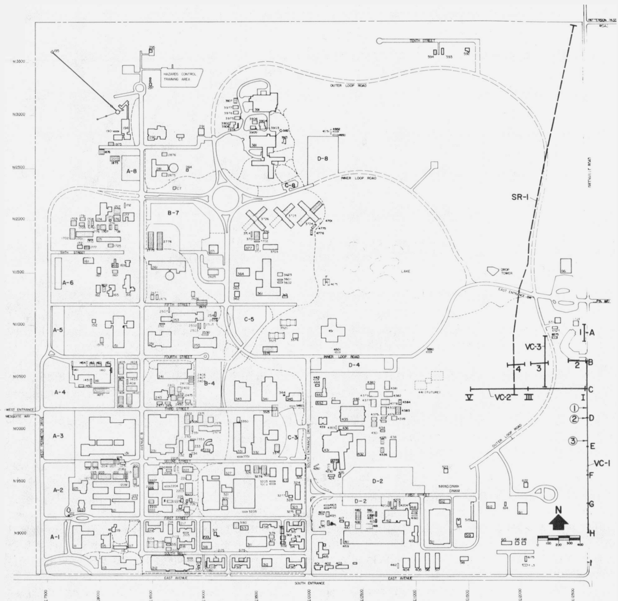
Fig. C-15. Locations of seismic refraction surveys near the east boundary of LLNL. Survey lines 1 through 4 are small-scale seismic lines using a sledge hammer as the source. A Dinoseis source was used for the large-scale seismic lines, VC-1 through VC-3.
