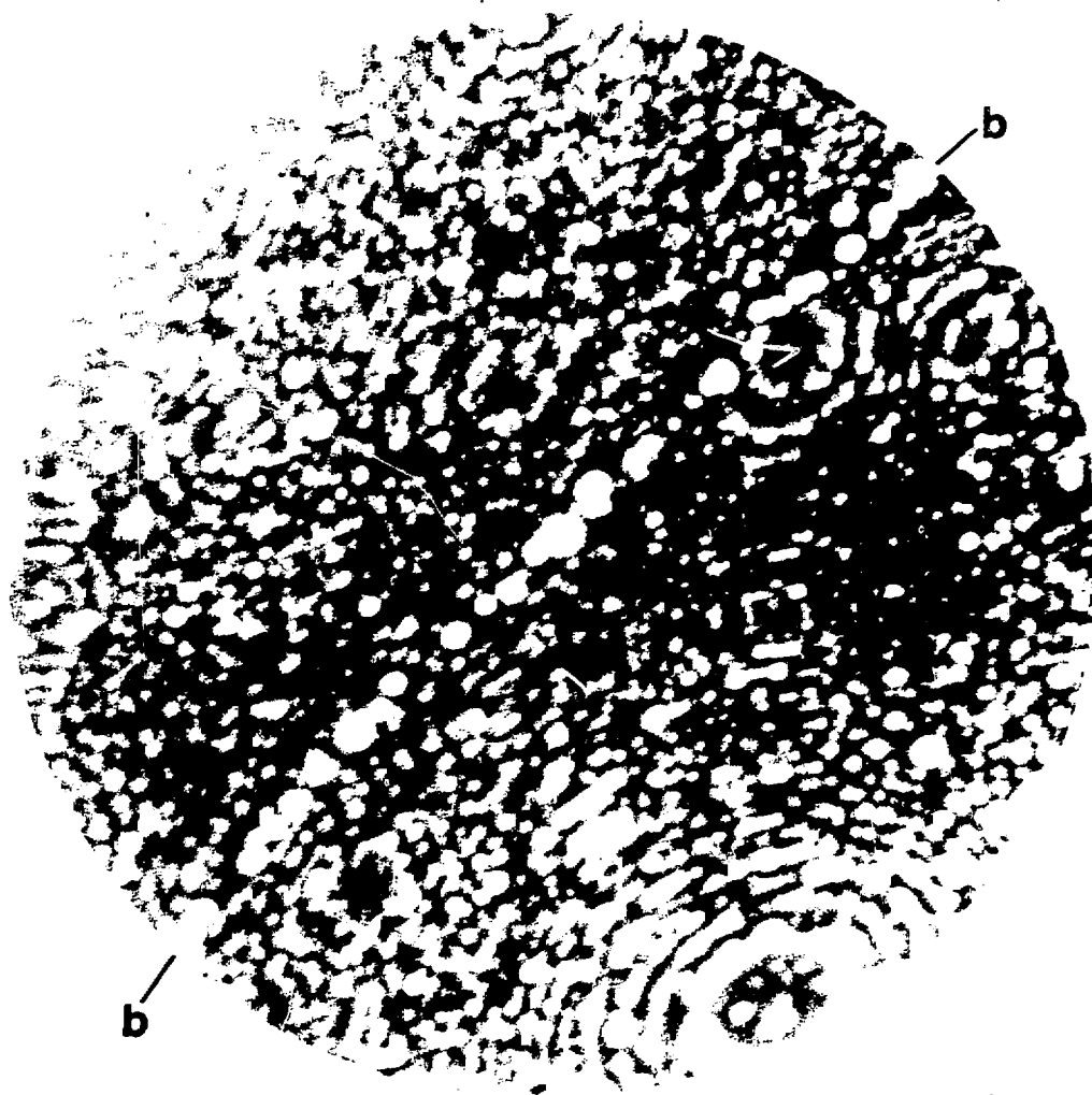
Fig. 2 FIM micrograph of a boron decorated boundary in rapidly solidified Ni - 24.0 at. % Al - 0.24 at. % B. Each bright spot is an individual boron atom.
