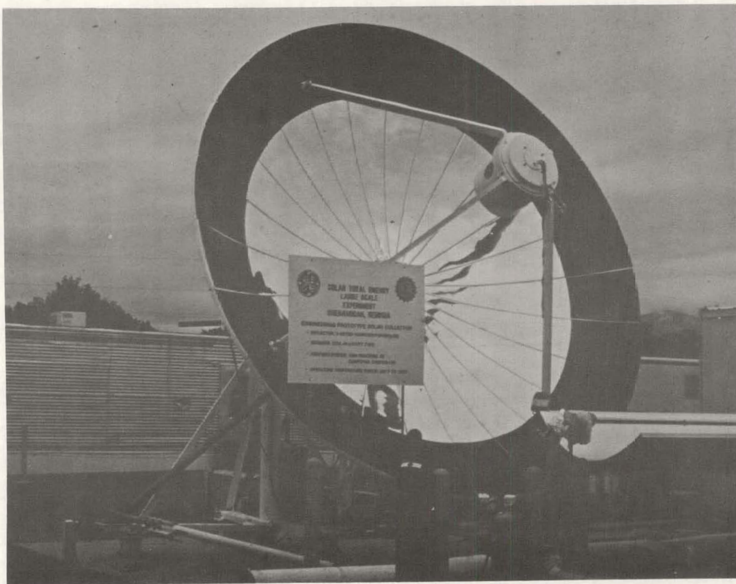
Figure 1.3-6. Prototype Parabolic Solar Collector
