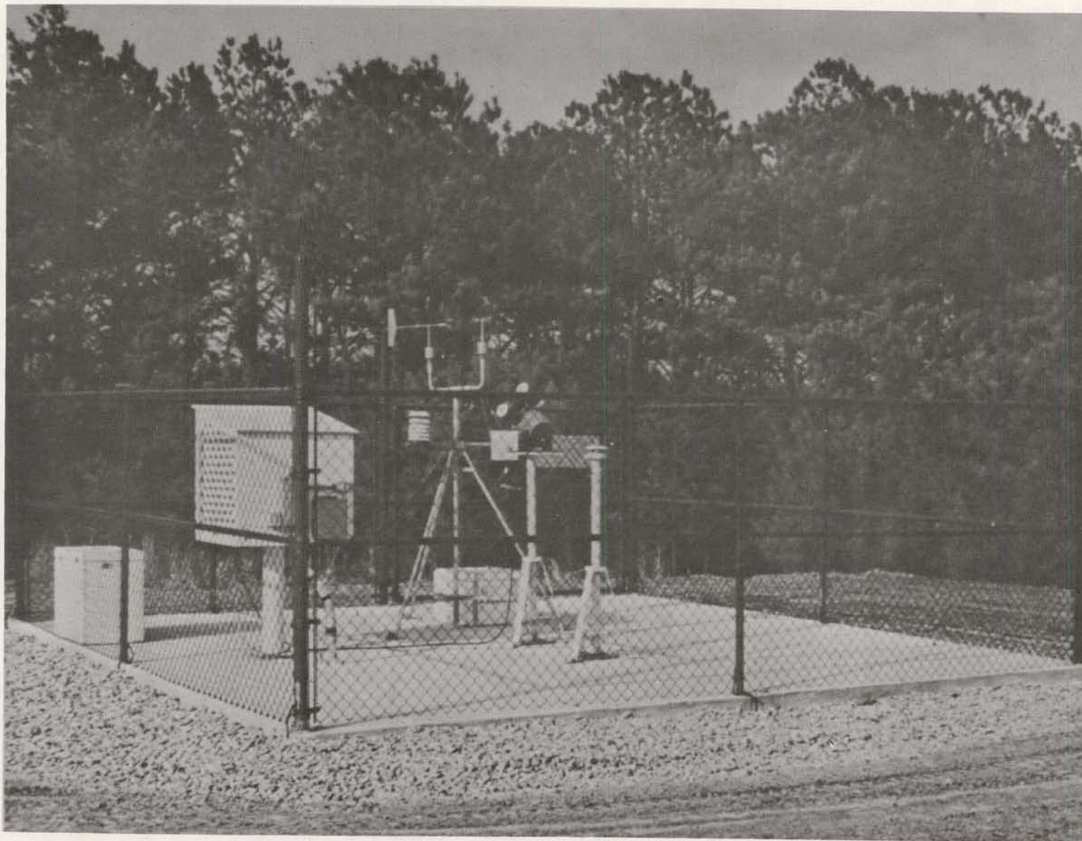
Figure 2.3-1. Government-Supplied Weather Station
