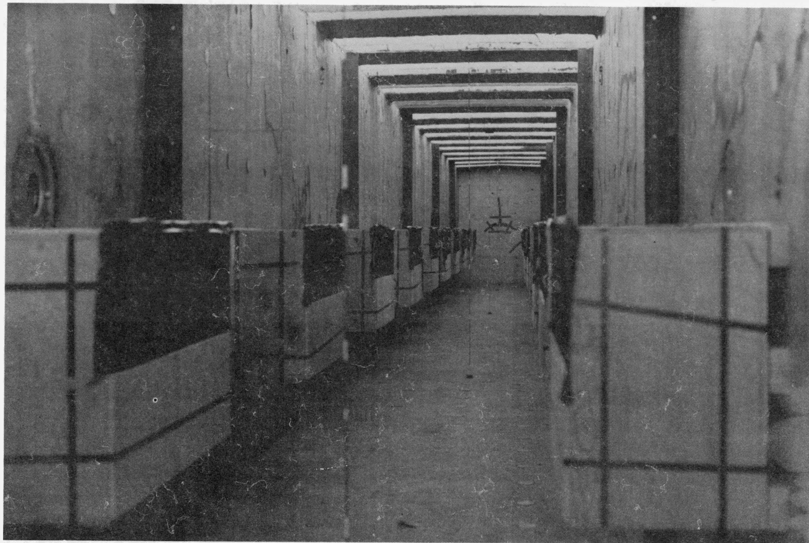
Figure 2.5. Interior of FLAME Channel With Plywood Boxes Simulating Half-Scale Model of the Ice Condenser Upper Plenum Region. Blockage ratio is 11%.
