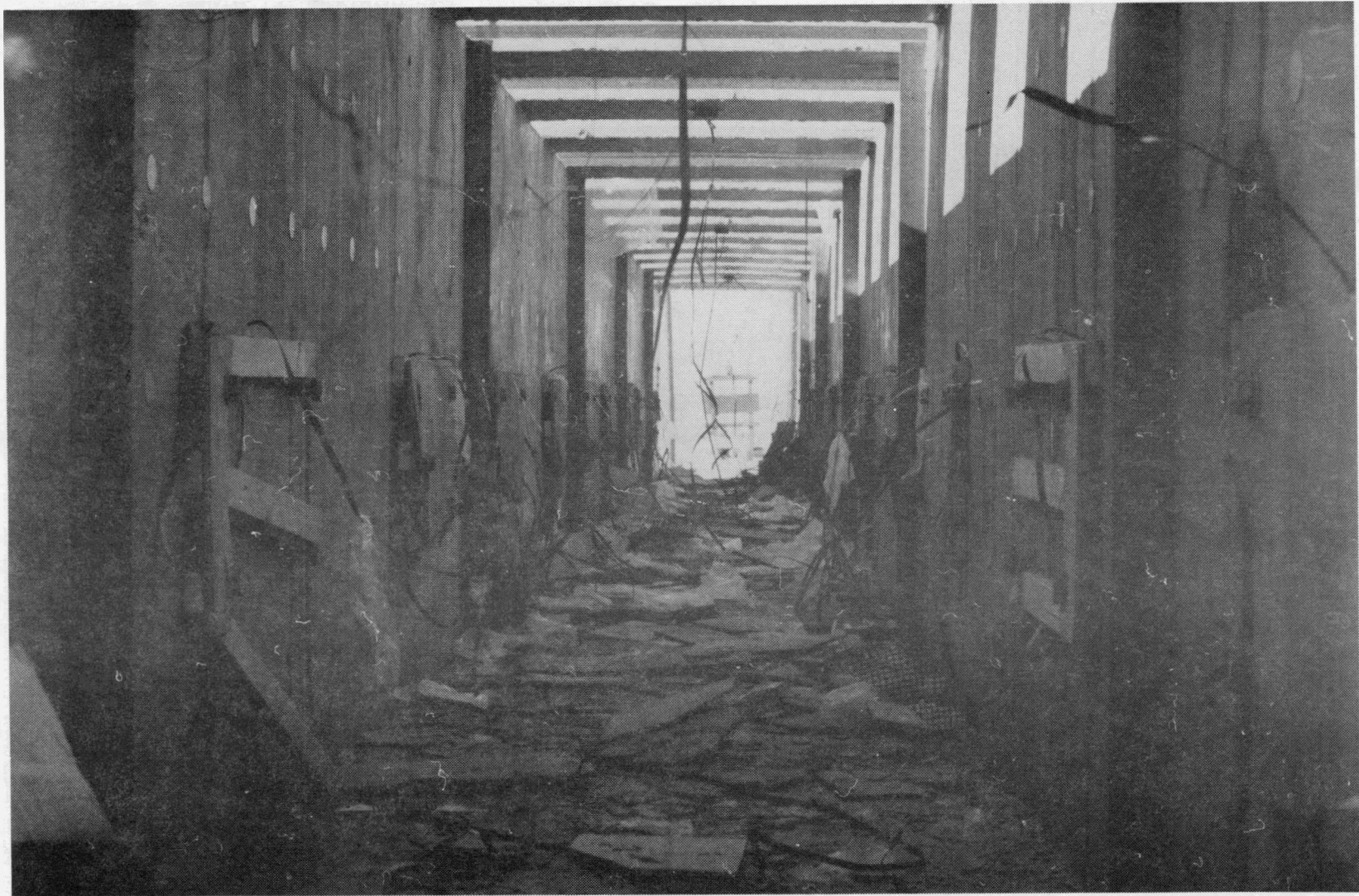
Figure 2.6. Interior of FLAME Channel After Test F-26. Detonation has destroyed boxes shown in Figure 2.5.
