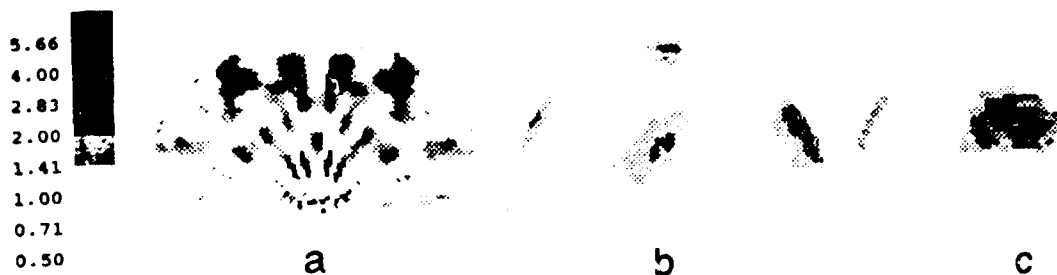
Fig. 4. {111} pole figures (in equal area projection) for Al-1Mg, a) initial texture, b) tested in torsion to \gamma=3.5 and c) in torsion to \gamma=3.5 followed by reverse torsion to \gamma=0 .
