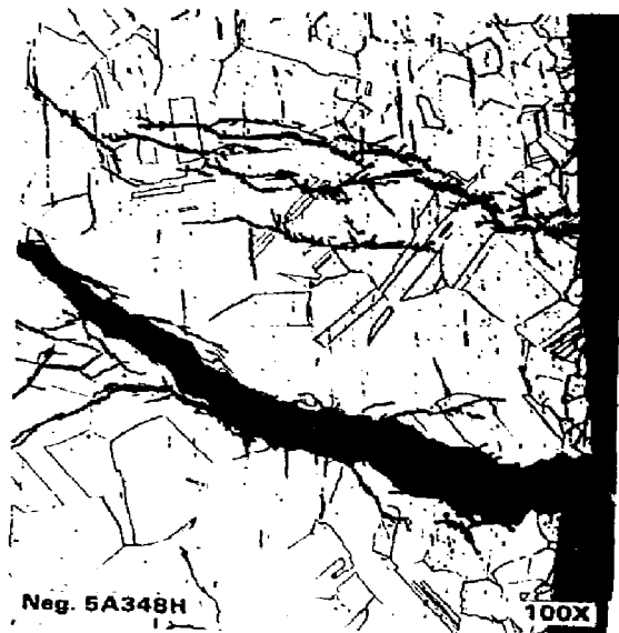
FIGURE 5.3. Transgranular Cracking of Solution-Annealed-and-Sensitized 304L SS (Specimen P434). The specimen was exposed for 14 months to the vapor-only region of the 90°C autoclave test system.
