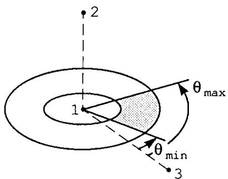
Point 1 is the center of the disk and point 2 is on the normal to the disk passing through the center of the disk.  $r_o$  is the outer radius of the disk. If desired,  $r_{in}$  may be specified, thus restricting the source to an annulus. Further restriction may be obtained by giving point 3 on the plane of the disk to define  $\theta = 0$  and then providing  $\theta_{min}$  and  $\theta_{max}$  (in degrees) between which the source will occur.
