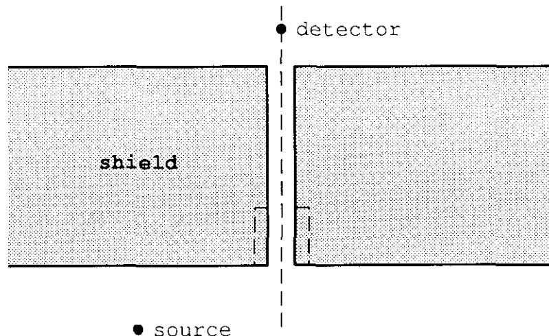
The first collision scatterings in the small cylindrical annulus around the hole on the source side of the shield produces particles that contribute almost all the response of the detector.
