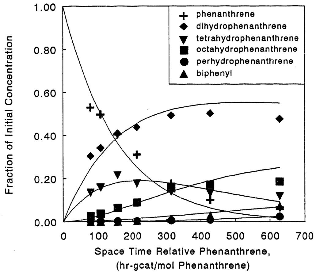
Figure 7 Space time plot of the hydrogenation of phenanthrene with no added ammonia. Solid lines represent first order kinetics.
