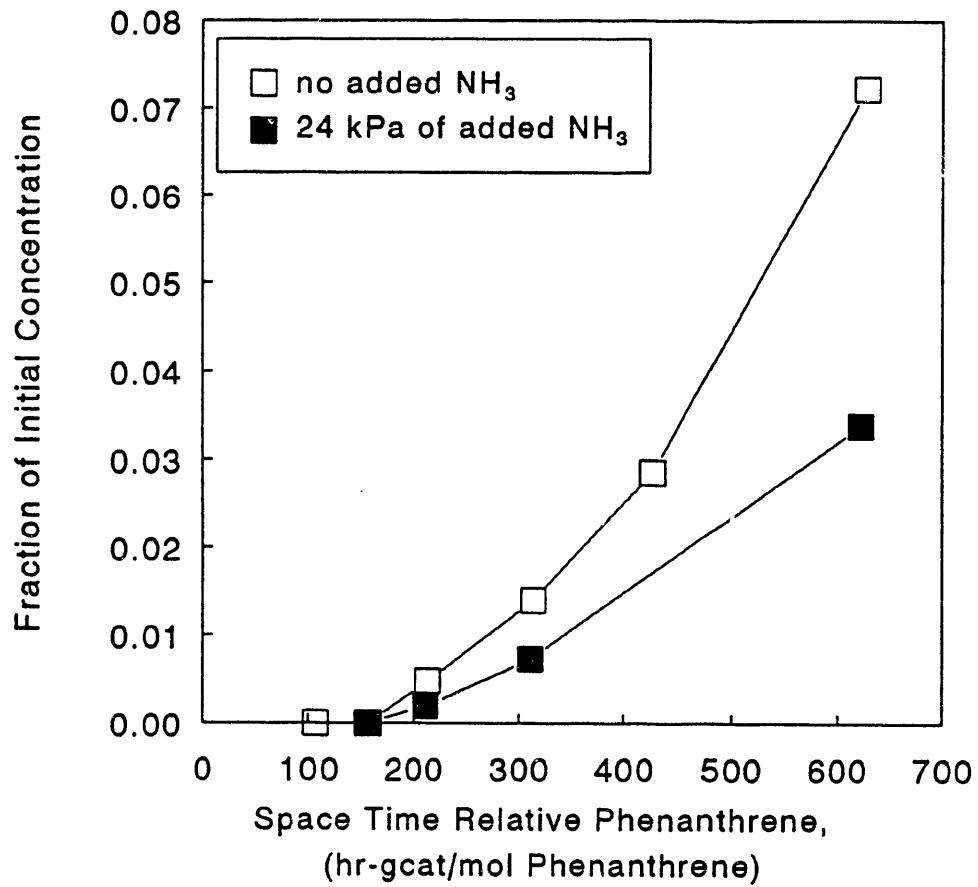
Figure 5 Ammonia reduces the amount of hydrocracking of 9,10-dihydrophenanthrene to biphenyl.
