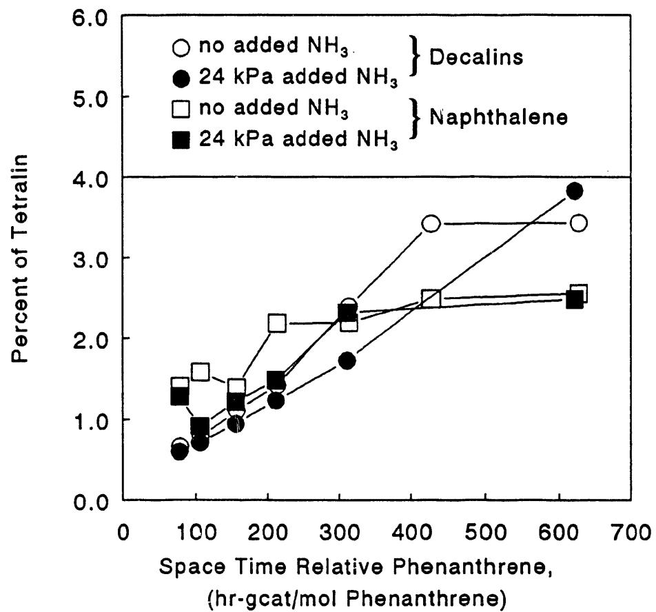
Figure 1 Ammonia had little effect on the hydrogenation of tetralin to decalins or the dehydrogenation of tetralin to naphthalene.
