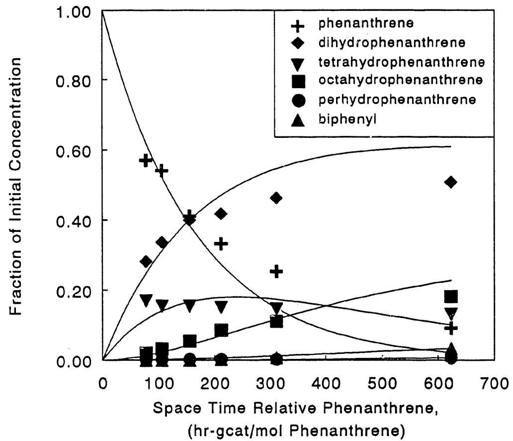
Figure 8 Space time plot of the hydrogenation of phenanthrene with 24 kPa of ammonia. Solid lines represent first order kinetics.
