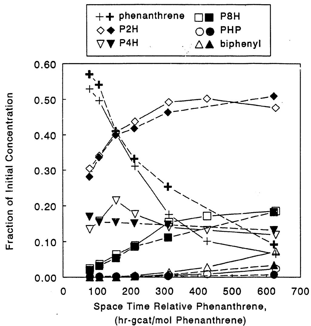
Figure 2 Effect of ammonia on the hydrogenation of phenanthrene during the HDN of quinoline. Open symbols represent no added ammonia; filled symbols represent 24 kPa of added ammonia.
