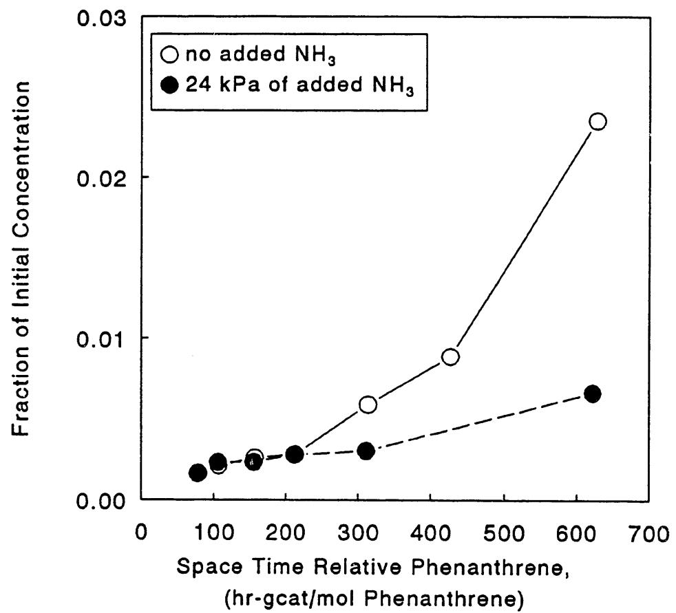
Figure 4 Ammonia inhibits the formation of perhydrophenanthrene.
