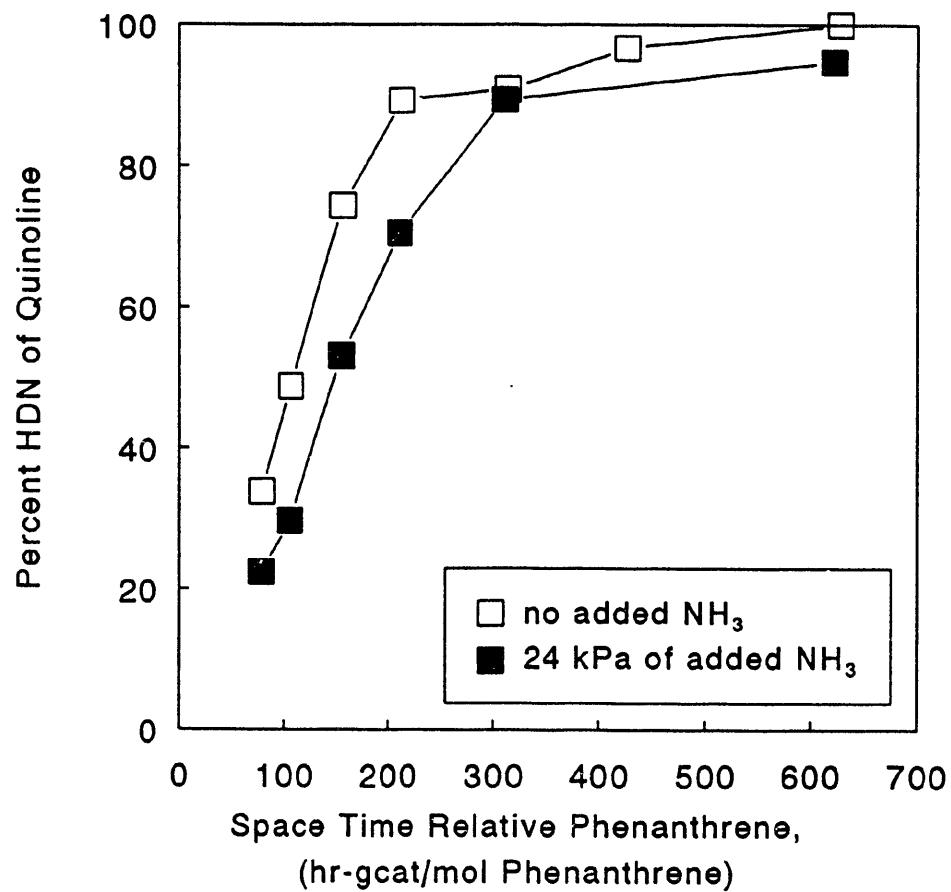
Figure 3 Hydrodenitrogenation of quinoline without added  $\text{NH}_3$  and in the presence of 24 kPa of  $\text{NH}_3$ .
