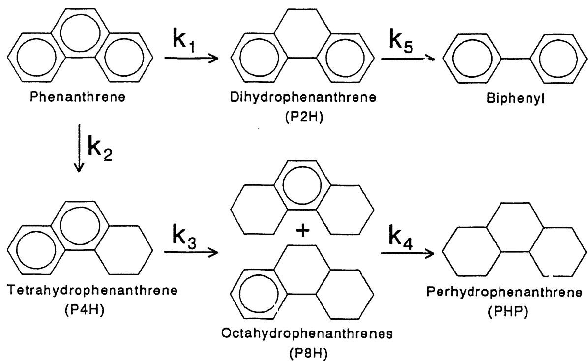
Figure 6 Kinetic model of the hydrogenation of phenanthrene assuming first order reactions.
