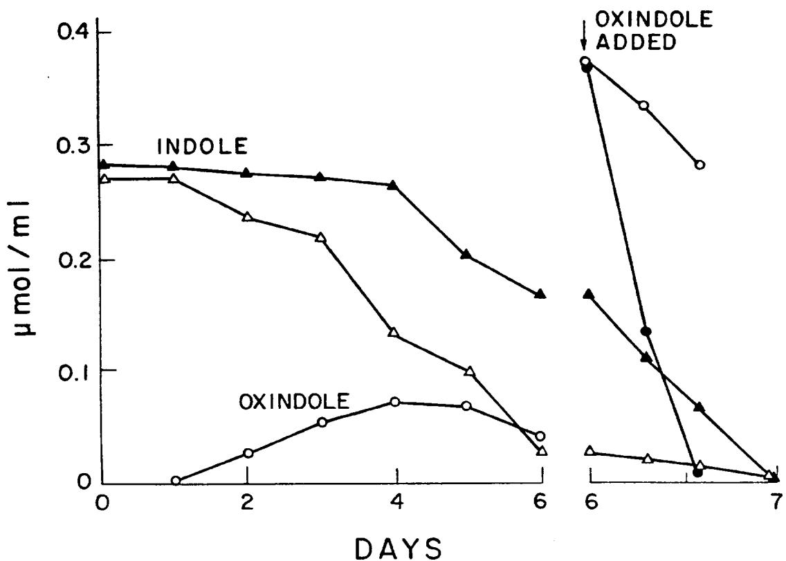
Fig. 1. Transformation of indole and oxindole by 9% digested sludge under methanogenic ( $\textcircled{O}$ ,  $\triangle$ ) and denitrifying ( $\textbullet$ ,  $\blacktriangle$ ) conditions.
