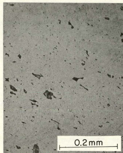
d. Example of the agglomerated metallic structure
