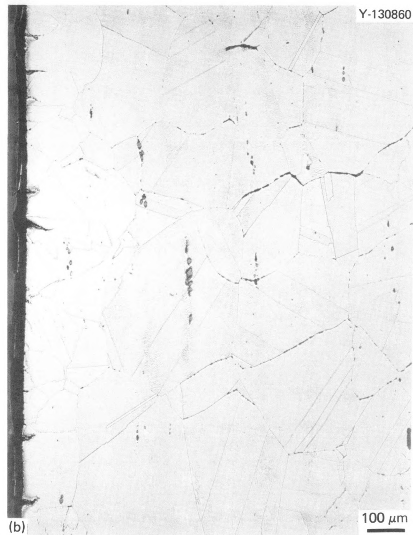
Fig. 20. Ruptured Specimens Showing (a) Wedge Cracking and (b) Microvoid Formation.
