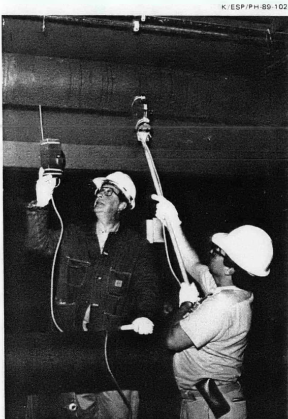
Fig. 2 - Scanning and incremental measurements of process piping with sodium iodide detectors
