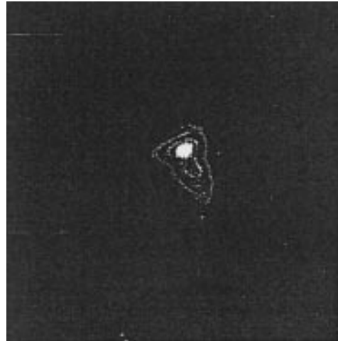
Fig.8: The far field irradiance distribution obtained at the output of the compressor.
