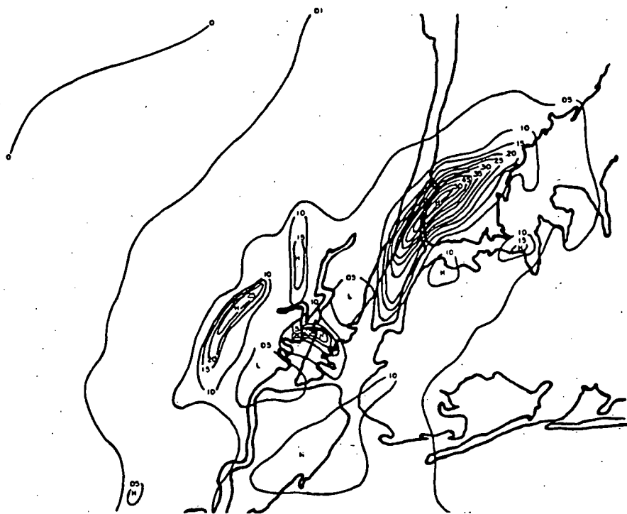
Figure 12. Predicted \text{SO}_2 concentration field (ppm), 1800 March 9, 1966, 1.0 mile x 1.0 mile computational grid. (From Shieh et al., 1970)
