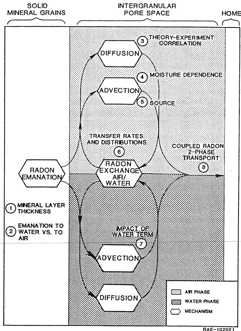
FIGURE 1-1. PHYSICAL MECHANISMS OF RADON GENERATION AND TRANSPORT.
