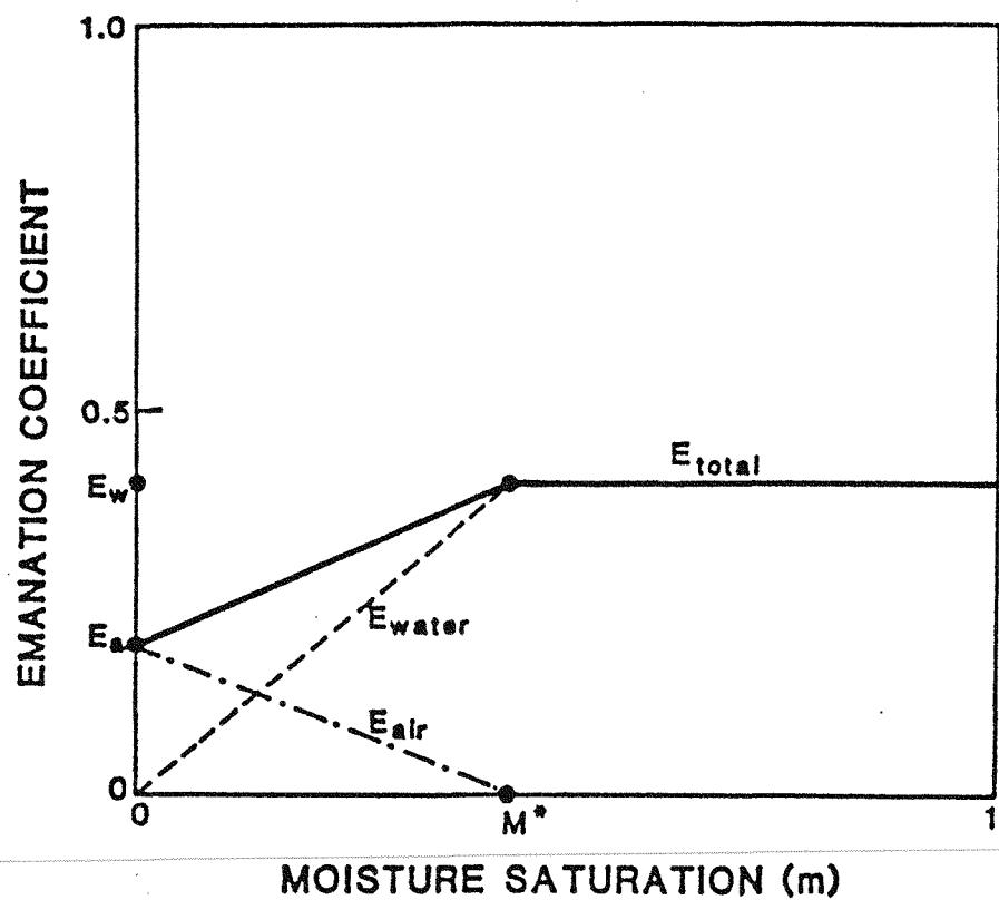
FIGURE 2-2. COMPONENTS OF THE EMANATION COEFFICIENT AS A FUNCTION OF MOISTURE.
