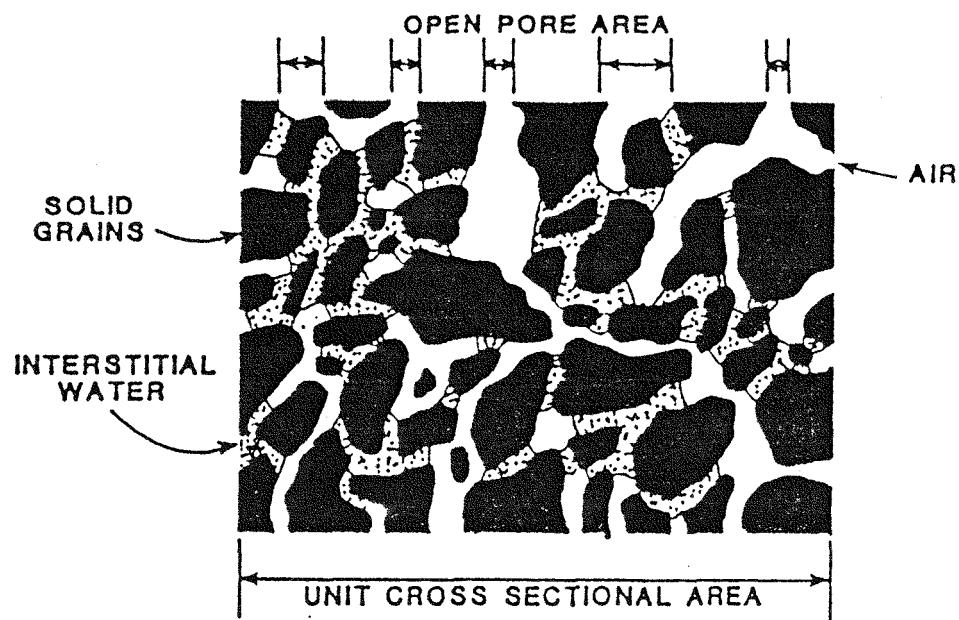
FIGURE 2-1. VOLUME OF UNSATURATED POROUS MATERIAL. RADIUM IS IN THE SOIL GRAINS AND INTERSTITIAL WATER.
