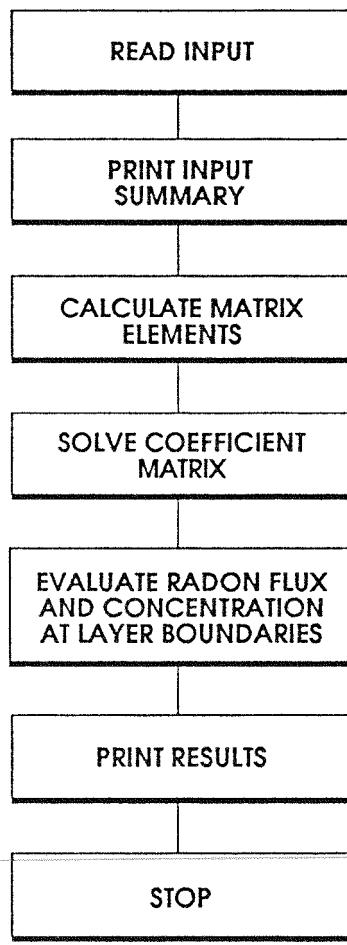
FIGURE 3-3. LOGIC FLOW FOR RAETRAN CODE.
