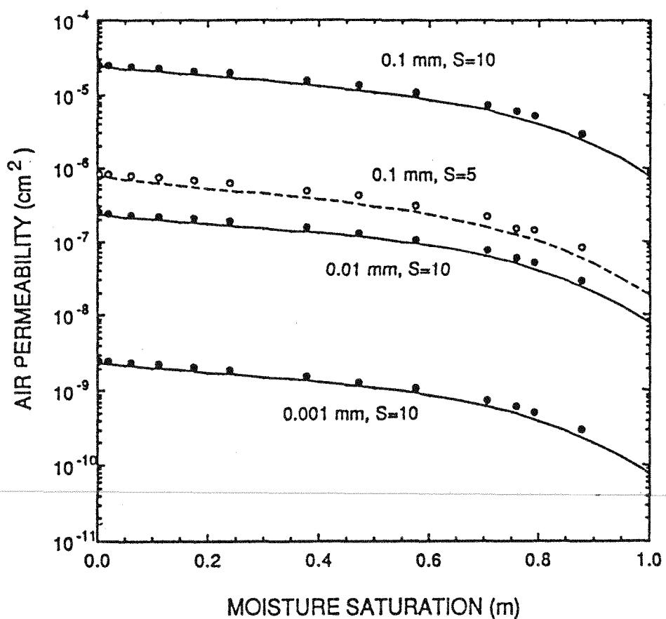
FIGURE 4-1. AIR PERMEABILITY FOR VARIOUS SOIL TYPES.
