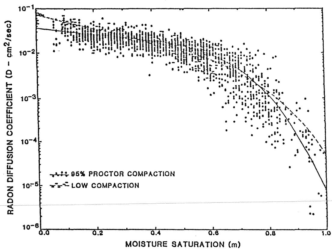
FIGURE 4-2. MEASURED RADON DIFFUSION COEFFICIENT AND CORRELATION PREDICTIONS.
