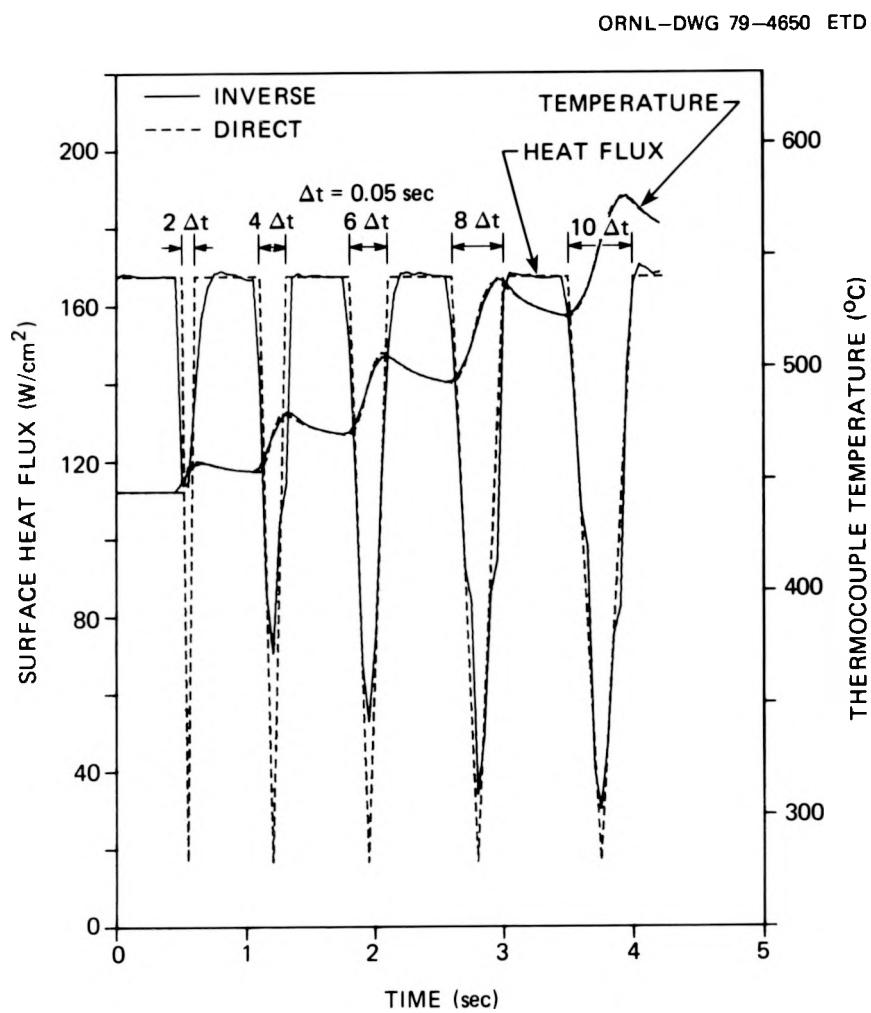
Figure 14. Second test case: Comparison of direct solution with inverse solution using one future temperature ( $J = 2$ )
