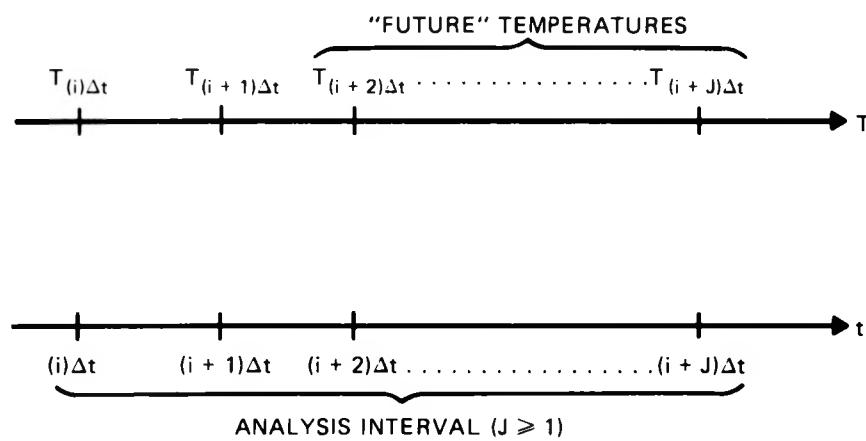
Figure 5. Analysis interval for computing surface heat flux  $q_{(i+1)\Delta t}$
