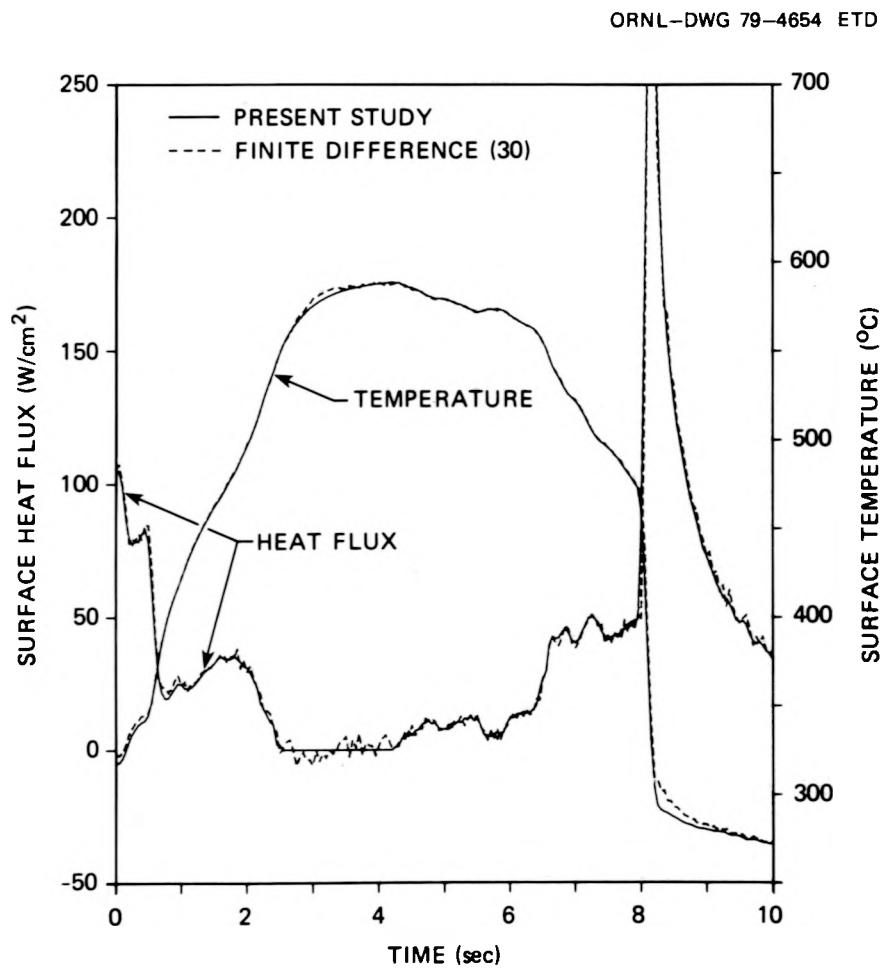
Figure 22. Thermocouple TE-325AD: Comparison of INCAP inverse solution using one future temperature ( $J = 2$ ) with ORINC solution
