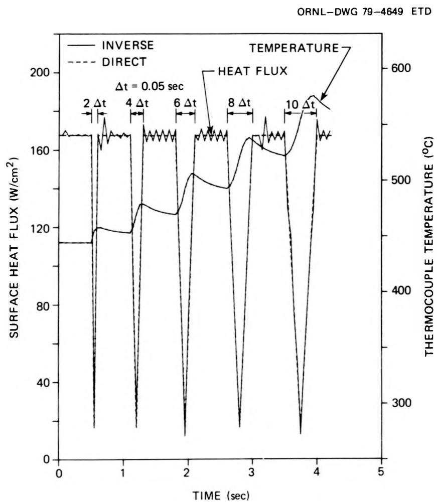
Figure 13. Second test case: Comparison of direct solution with inverse solution using no future temperatures ( $J = 1$ )
