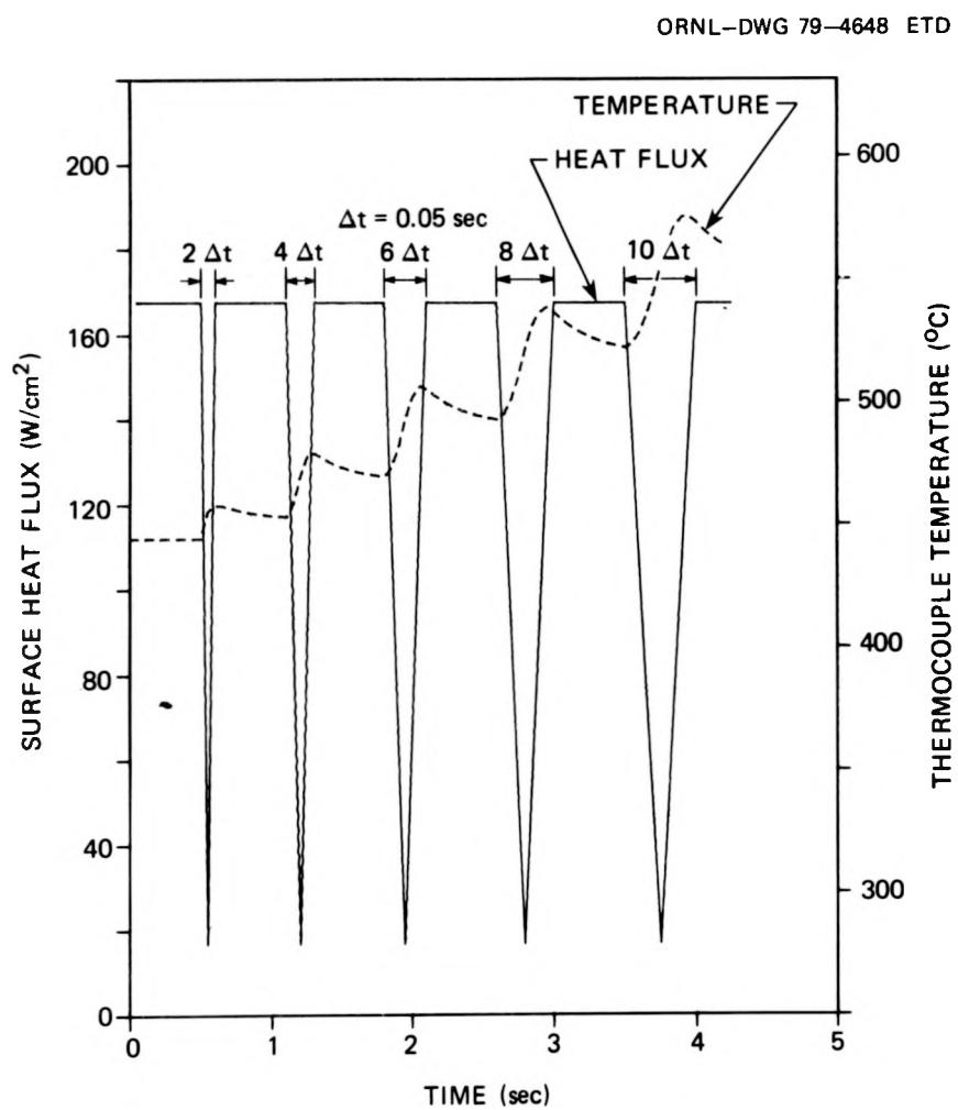
Figure 12. Second test case: Imposed surface heat flux and calculated thermocouple temperature of direct solution
