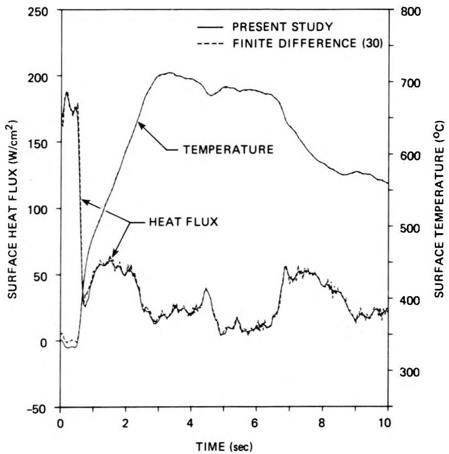
Figure 18. Thermocouple TE-325BG: Comparison of INCAP inverse solution using one future temperature ( $J = 2$ ) with ORINC solution
