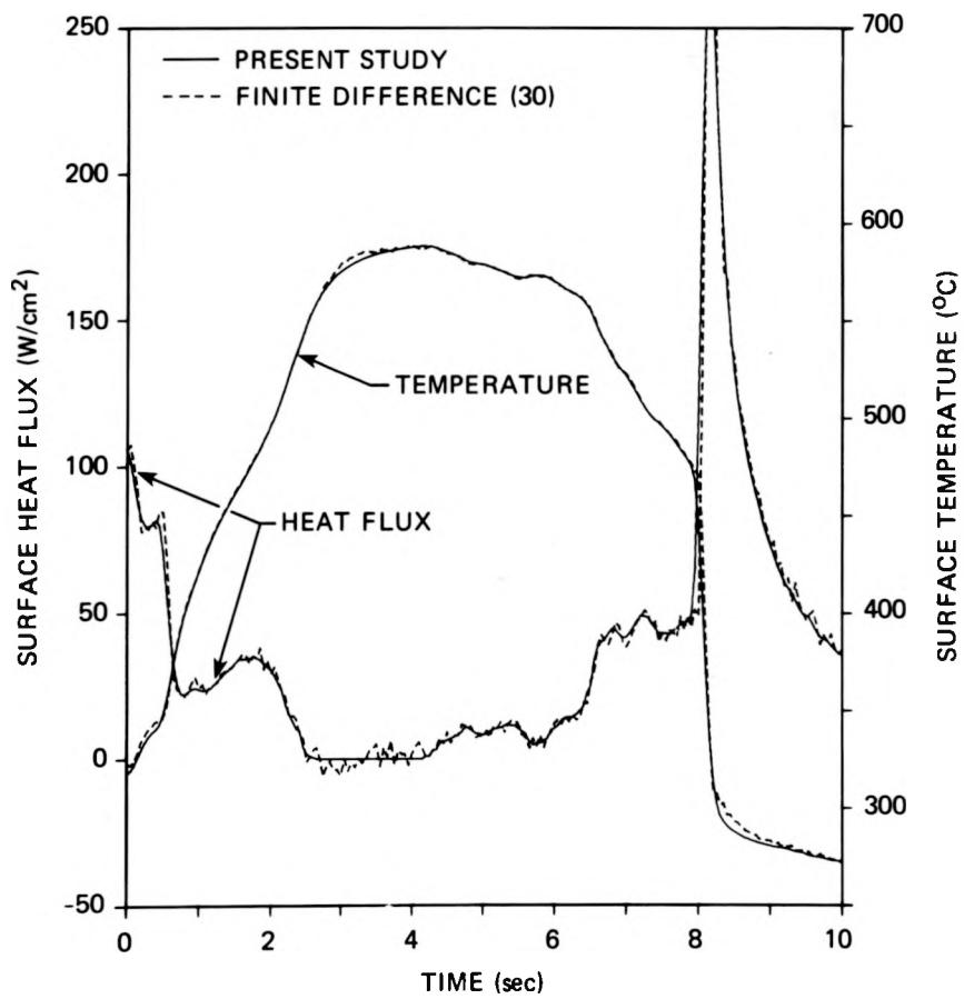
Figure 23. Thermocouple TE-325AD: Comparison of INCAP inverse solution using two future temperatures ( $J = 3$ ) with ORINC solution
