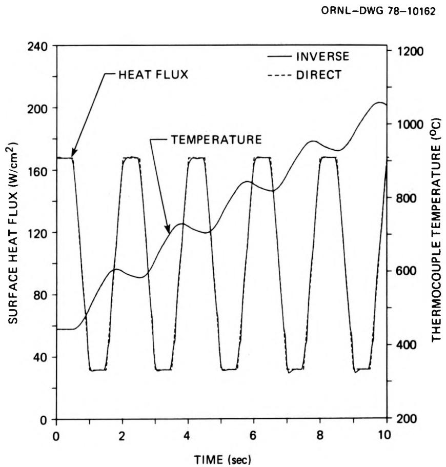
Figure 10. First test case: Comparison of direct solution with inverse solution using one future temperature ( $J = 2$ )
