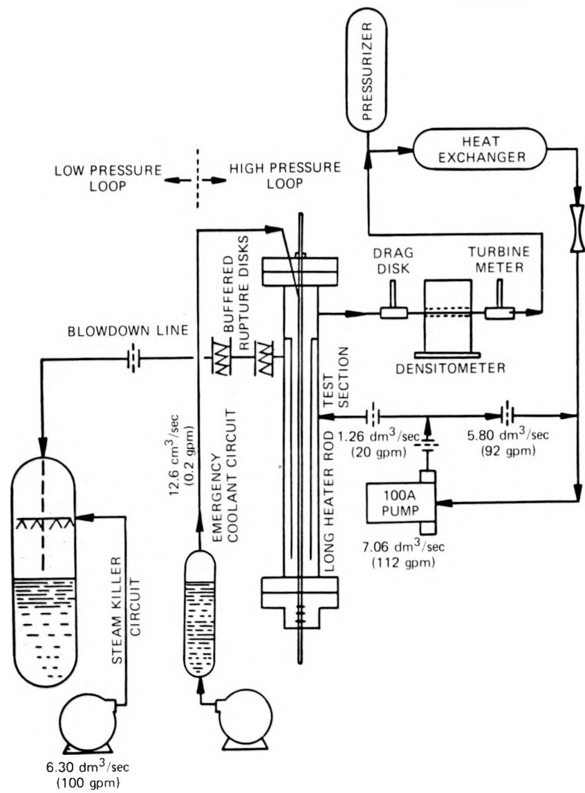
Figure 2. Forced Convection Depressurization Loop
