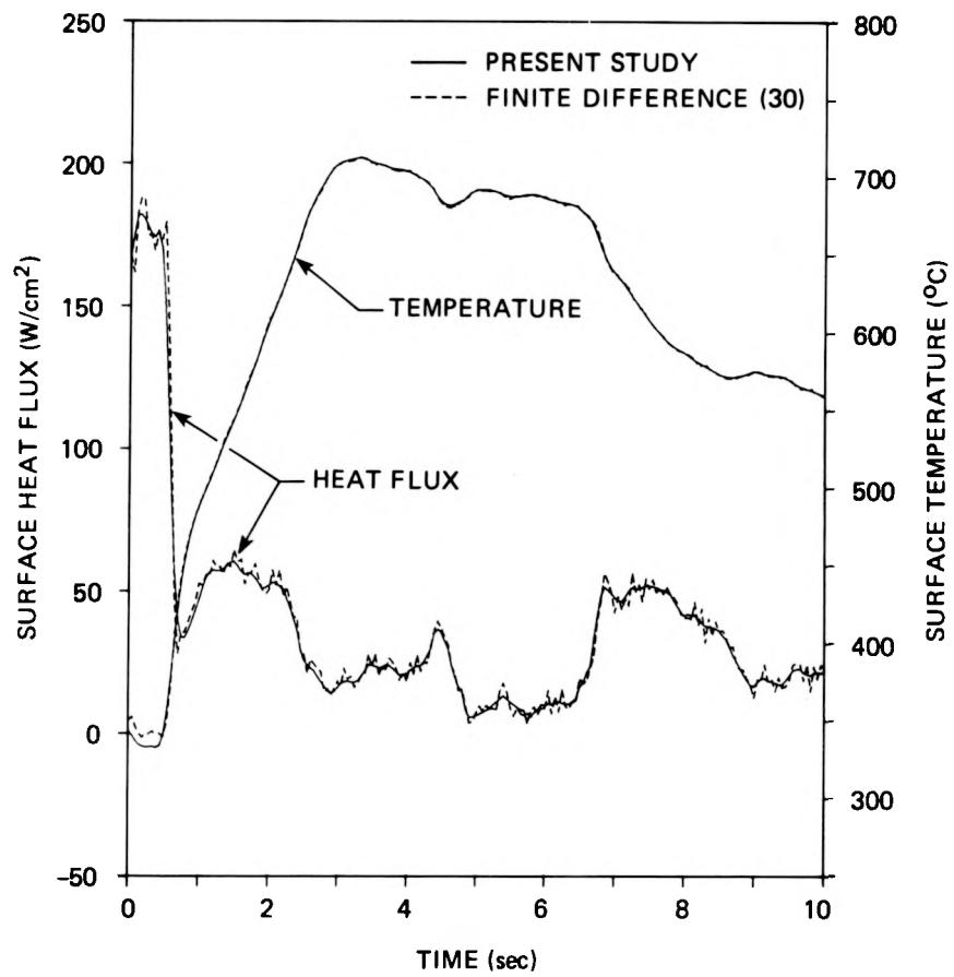
Figure 19. Thermocouple TE-325BG: Comparison of INCAP inverse solution using two future temperatures ( $J = 3$ ) with ORINC solution
