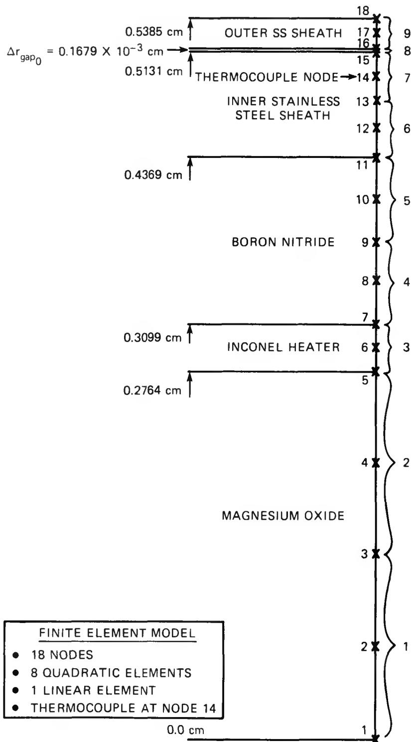
Figure 7. One-dimensional finite element model of heater rod cross section
