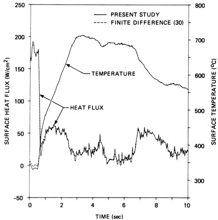
Figure 17. Thermocouple TE-325BG: Comparison of INCAP inverse solution using no future temperatures ( $J = 1$ ) with ORINC solution
