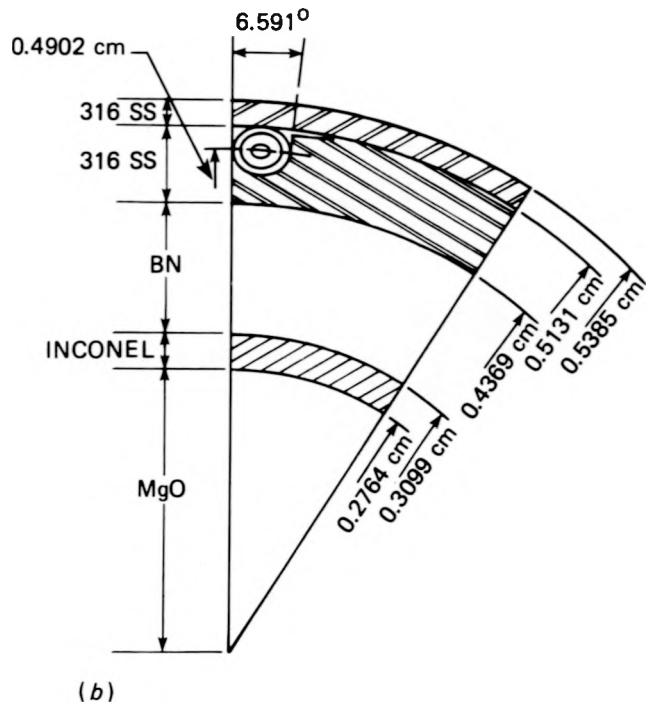
Figure 6. Electrically-heated rod containing thermocouple sensors
