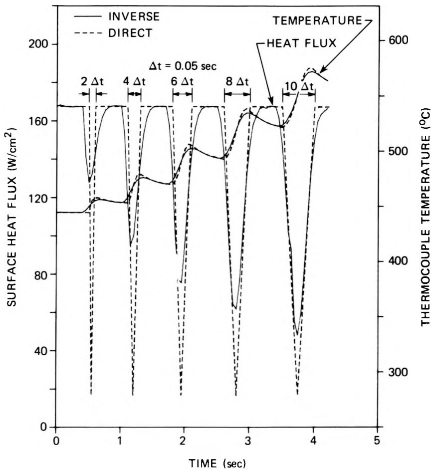
Figure 15. Second test case: Comparison of direct solution with inverse solution using two future temperatures ( $J = 3$ )
