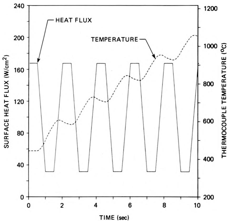
Figure 8. First test case: Imposed surface heat flux and calculated thermocouple temperature of direct solution
