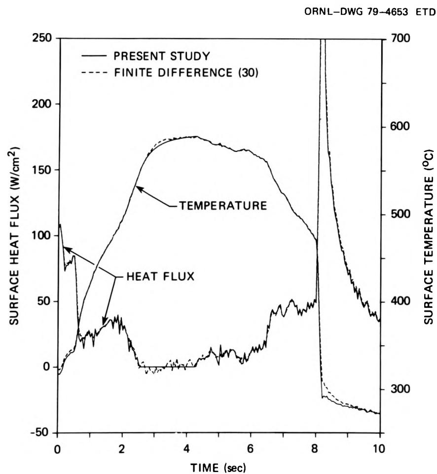
Figure 21. Thermocouple TE-325AD: Comparison of INCAP inverse solution using no future temperatures ( $J = 1$ ) with ORINC solution
