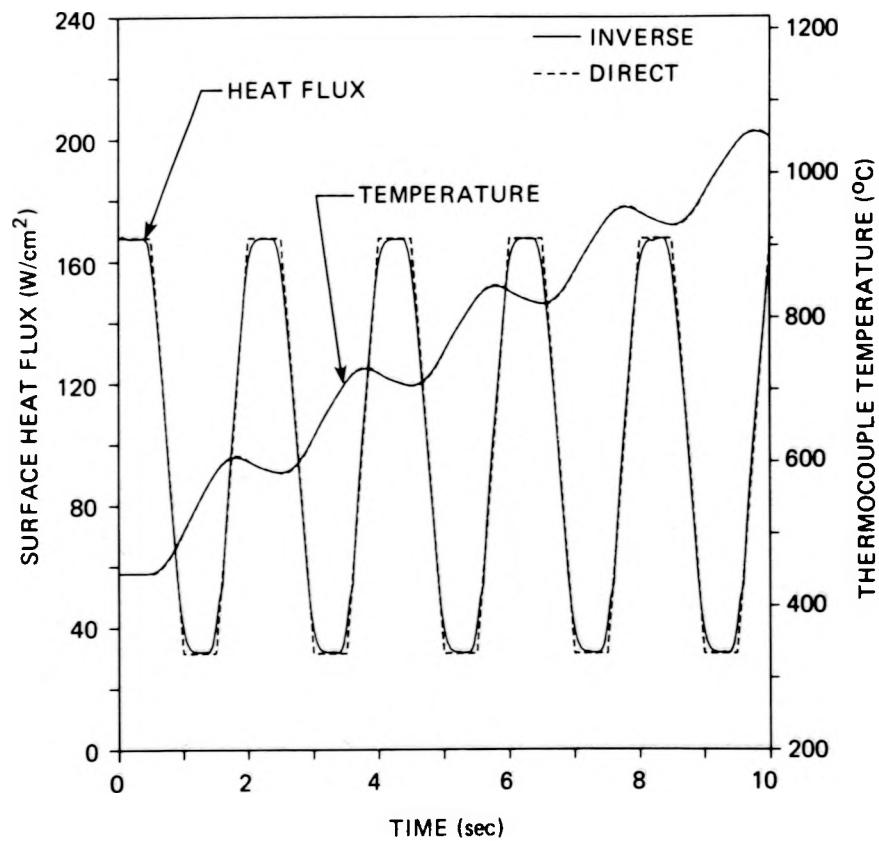
Figure 11. First test case: Comparison of direct solution with inverse solution using two future temperatures ( $J = 3$ )
