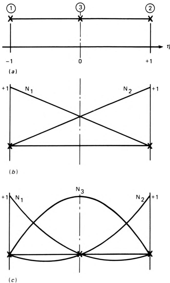
Figure 3. Interpolation functions for one-dimensional element
