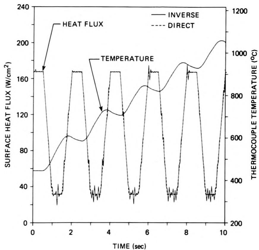
Figure 9. First test case: Comparison of direct solution with inverse solution using no future temperatures ( $J = 1$ )
