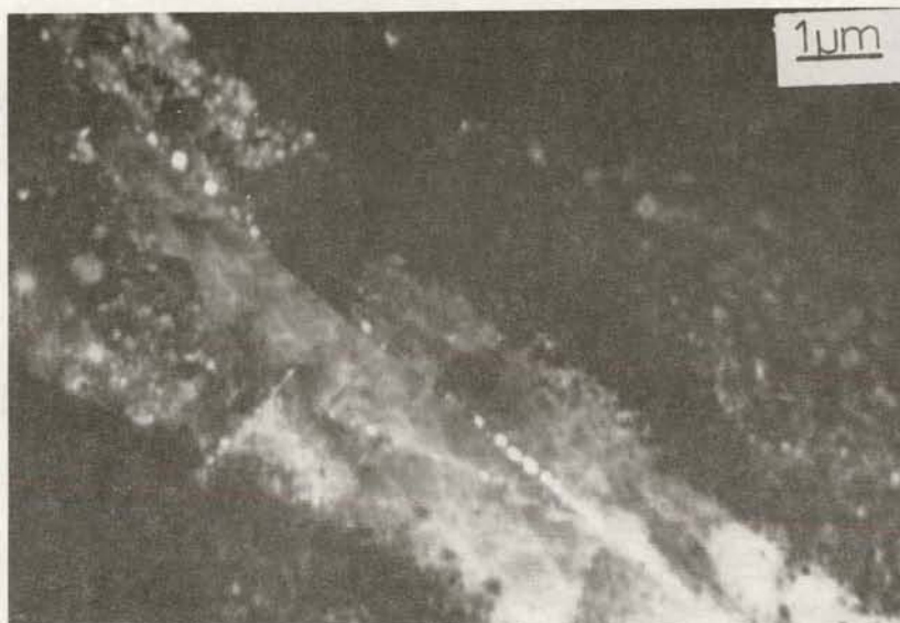
Fig. 7 HVEM micrograph (exp 17) of a helium ion irradiated sample fractured at 25°C. Note the bubble free band adjacent to the grain boundary and the bubble-decorated incoherent twin boundaries as well as a bubble-decorated grain boundary. The lower left grain has a (110) orientation (free surfaces). The upper right grain is (103).
