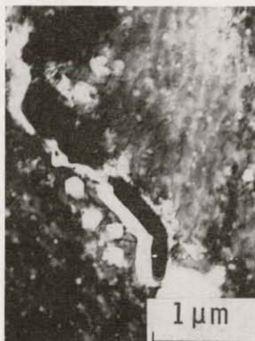
(b) Carbide Formation After 650°C Irradiation To 10 dpa
