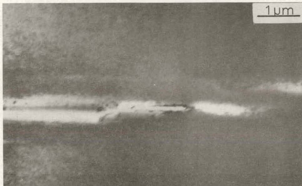
Fig. 3 HVEM micrograph (exp 25) of a neutron irradiated sample fractured at 400°C. Note that the crack is following a narrow slip band.
