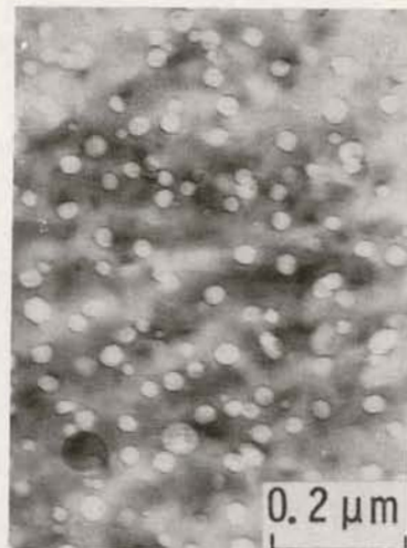
(a) Void Microstructure At 550°C, 9 dpa
