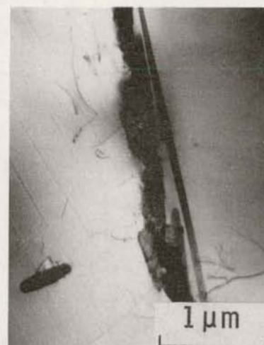
(c) Carbide Formation In Unirradiated, Aged 316 SS Specimen
