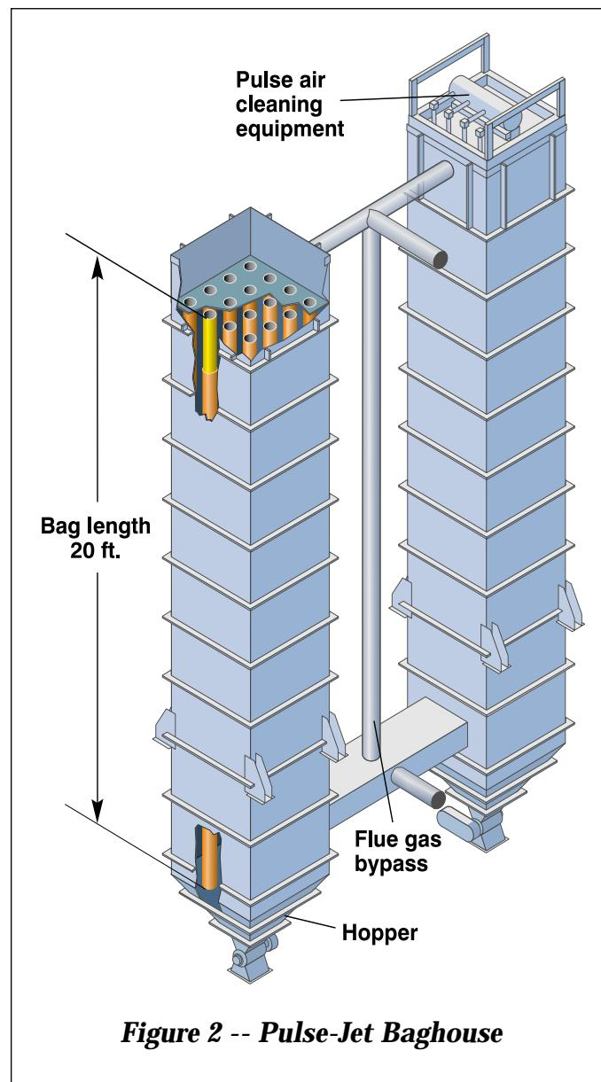
The baghouse is designed to process 6,000 lb/hr of flue gas with a particulate loading of 94 lb/hr. The baghouse will reduce particulate emissions to less than the New Source Performance Standard of 0.03 lb/ $10^6$  Btu. The primary design characteristics for the baghouse are summarized below:
