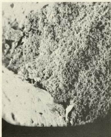
5601 + 0.5 mol % \text{CaCl}_2 Calcined 1h 850°C 638X
