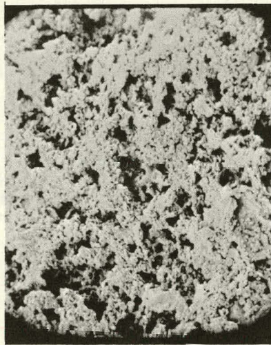
5401 + 3 mol % \text{CaCl}_2 Calcined 1h 850°C 1276X
