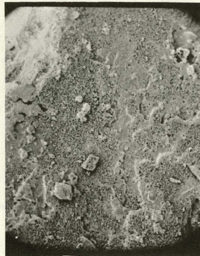
5401 + 0.1 mol % \text{CaCl}_2 Calcined 1h 850°C 1276X
