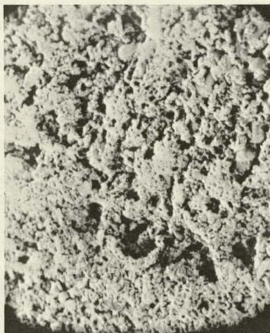
5601 + 1.0 mol % \text{CaCl}_2 Calcined 1h 850°C 638X
