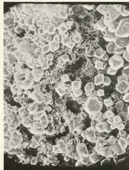
9501 Calcined 1 h Sulfated 2 h Reheated with NaCl 2 h 770X
