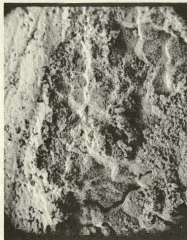
5601 + 0.1 mol % \text{CaCl}_2 Calcined 1h 850°C 638X
