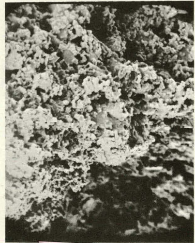
5401 + 5 mol % \text{CaCl}_2 Calcined 1h 850°C 1276X
