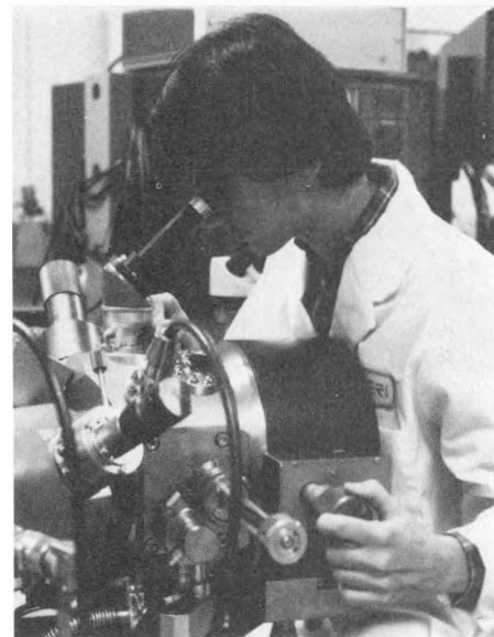
SERI researcher positions sample prior to volume-indexed SIMS analysis.
