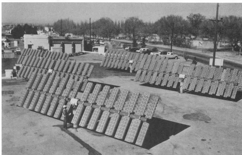
In FY 1985, Sandia showed that solar arrays, such as this one at the Photovoltaic Advanced Systems Test Facility in Albuquerque, can achieve peak efficiencies of 15%.
