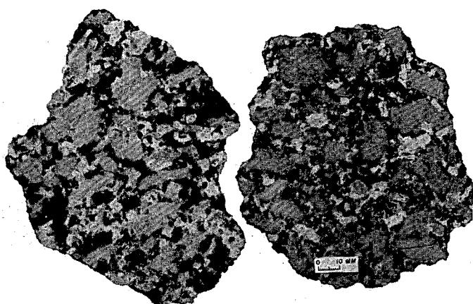
FIGURE 9.—Representative specimens of zone 2 (textural facies 2). Potassium feldspar phenocrysts in specimen to right are stained and appear gray. Quartz is smoky and appears black.
