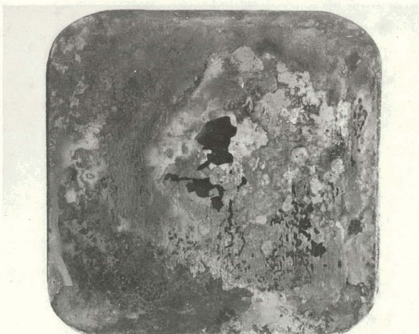
Figure 5.7 -- Top: CRD049 Stainless Steel Current Collector, Inlet Side Up (7.5X); Bottom: CRD049 Stainless Steel Insert (1.35X).
