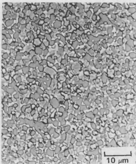
1130°C-99.9% Dense 48 HRC W Particle ~2 μm
