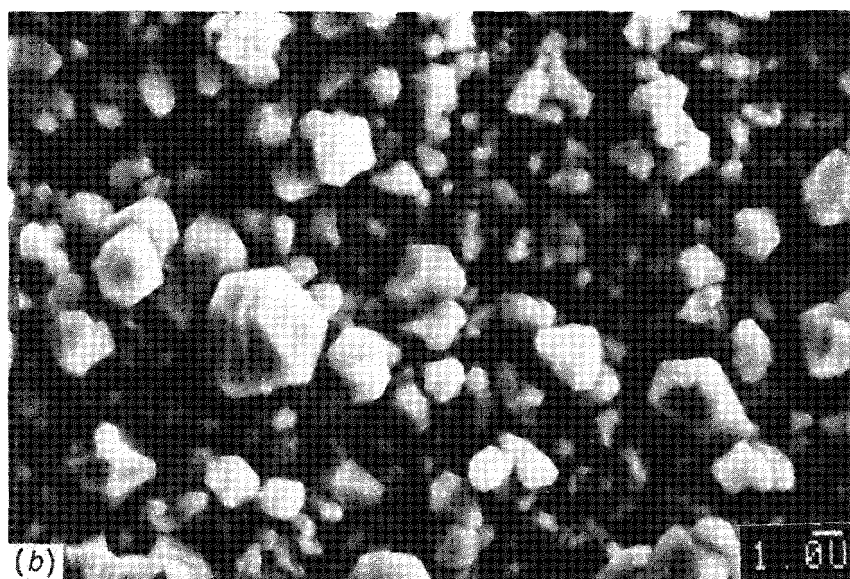
Fig. 3. Surface topographies of PS2 (Fe-18Cr-6Al) exposed to the gas mixture 2 with P_{S_2} = 10^{-6} and P_{O_2} = 10^{-20} atm at 800°C. (a) 5 min. (b) 10 min.
