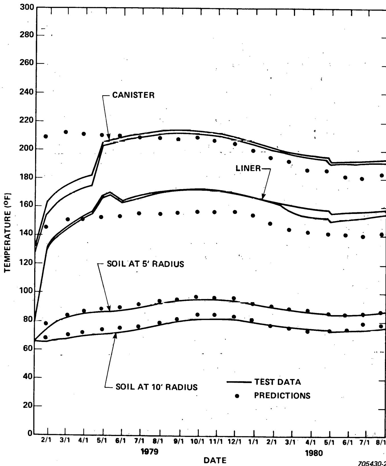
Figure 38. Drywell 5 Test Data and Predictions Comparison at About 205 Inches Below Ground Level
