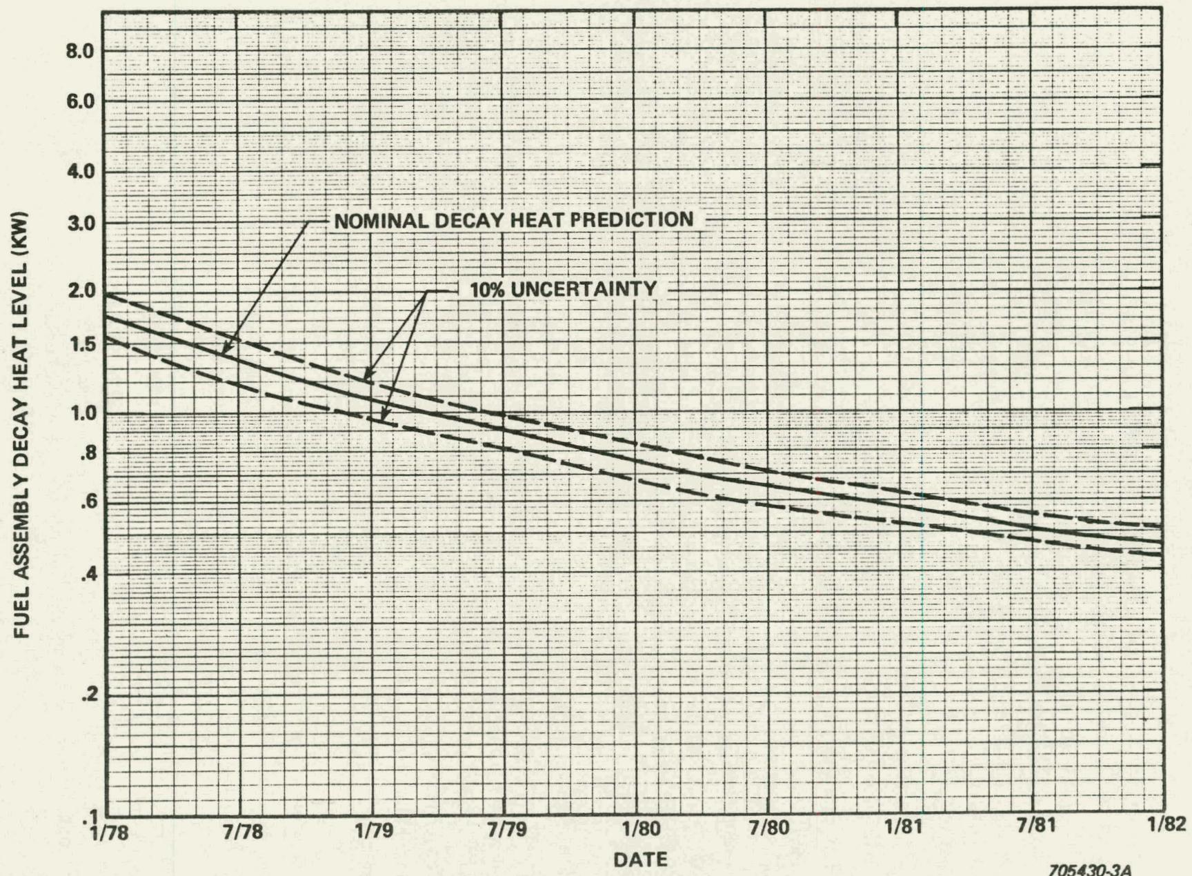
Figure 12. PWR Spent Fuel Assembly Predicted Nominal Decay Heat Curve
