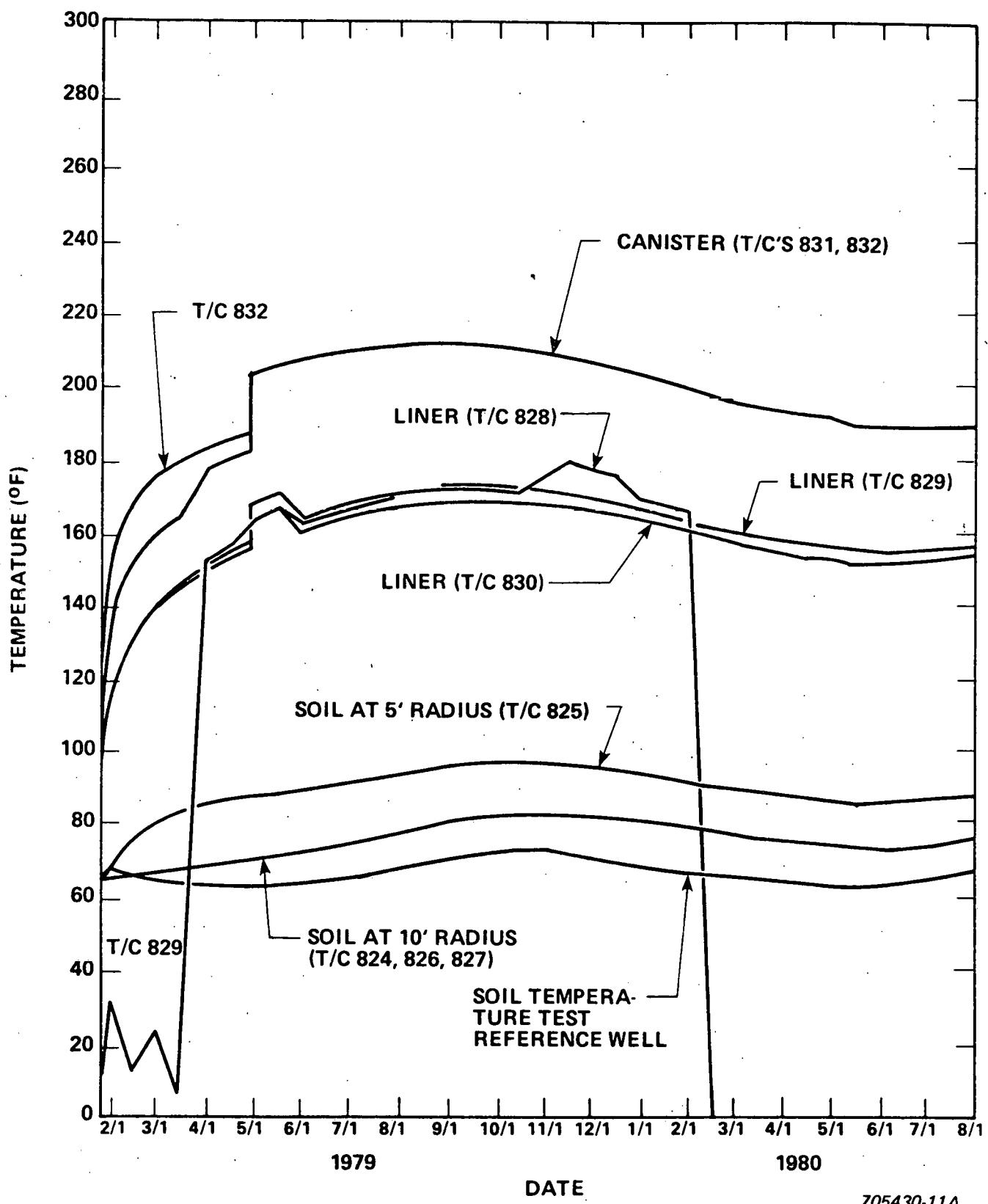
Figure C-3. Drywell 3 Canister, Liner, and Soil Temperature Distributions at About 205 Inches Below Ground Level
