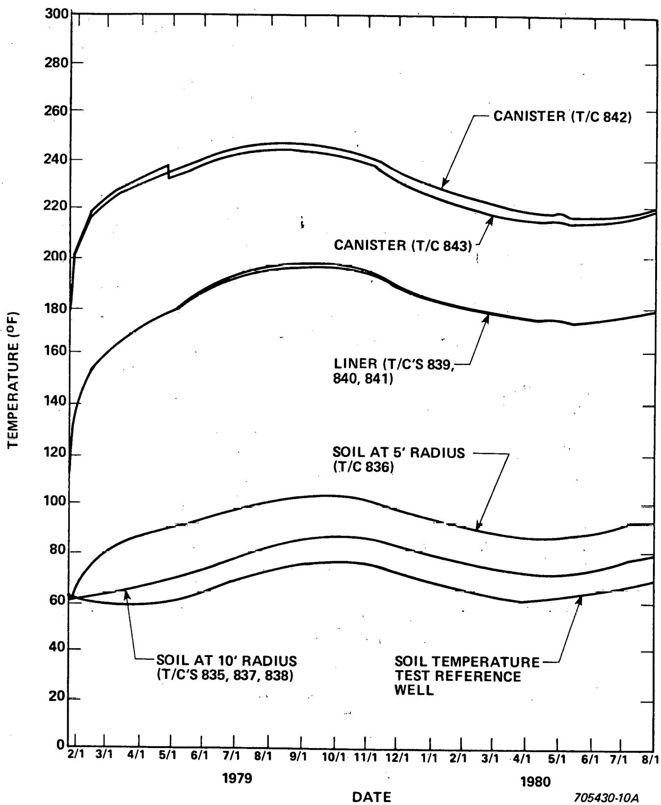
Figure C-2. Drywell-3 Canister, Liner, and Soil Temperature Distributions at About 145 Inches Below Ground Level
