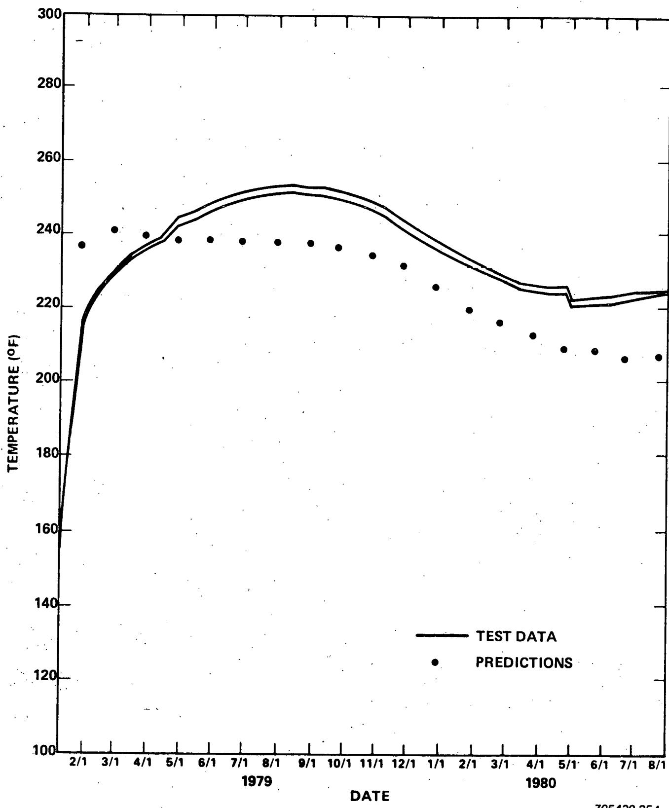
Figure 37. Drywell 5 Canister Test Data and Predictions Comparison at 176 Inches Below Ground Level
