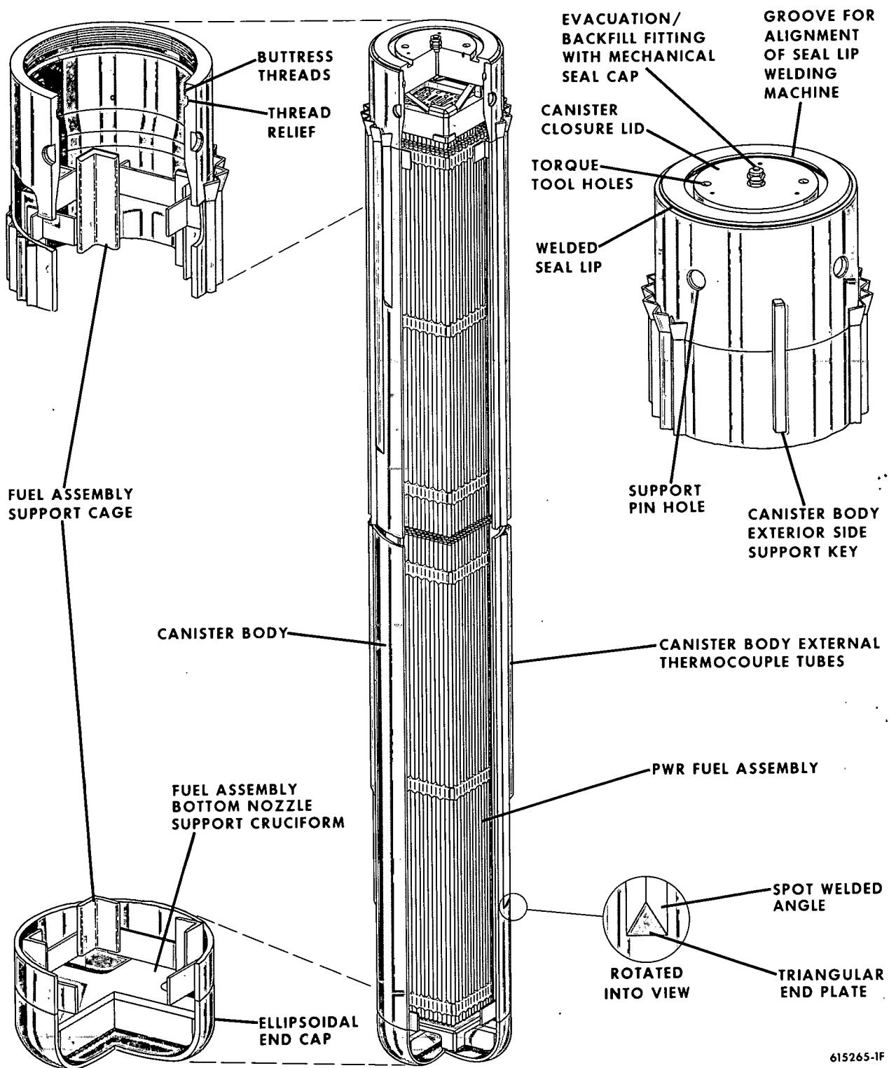
Figure 8. Canister Configuration
