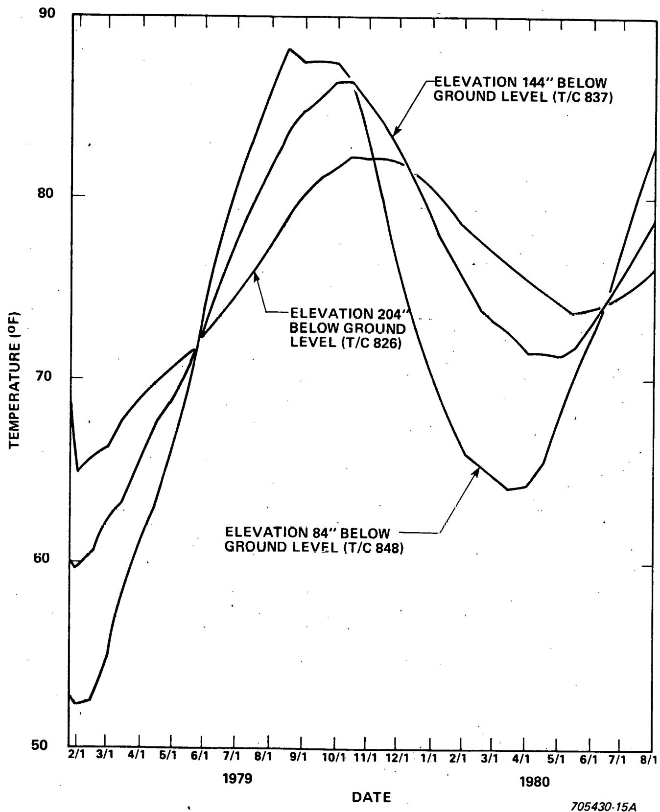
Figure 25. Drywell 3 Soil Temperature Distributions
