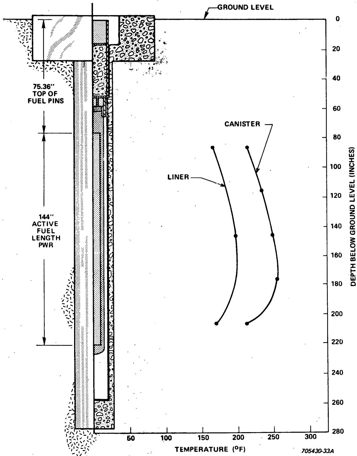
Figure 21. Drywell 3 Peak Canister and Liner Axial Temperature Profiles
