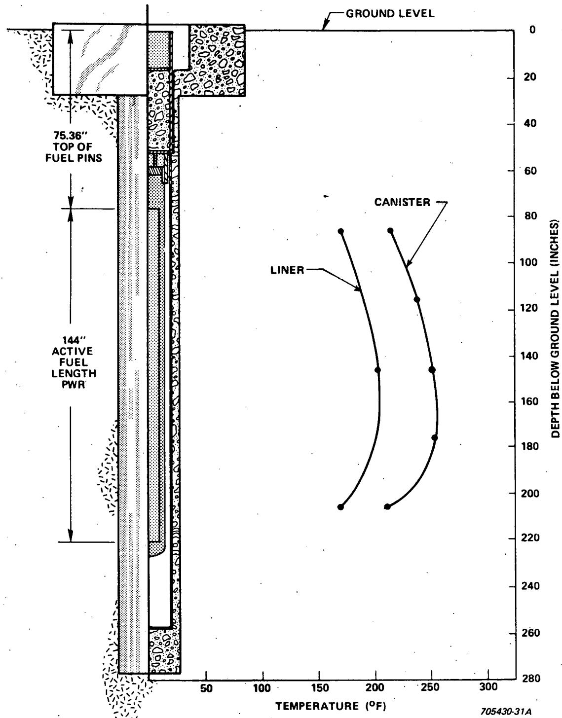
Figure 23. Drywell 5 Peak Canister and Liner Axial Temperature Profiles
