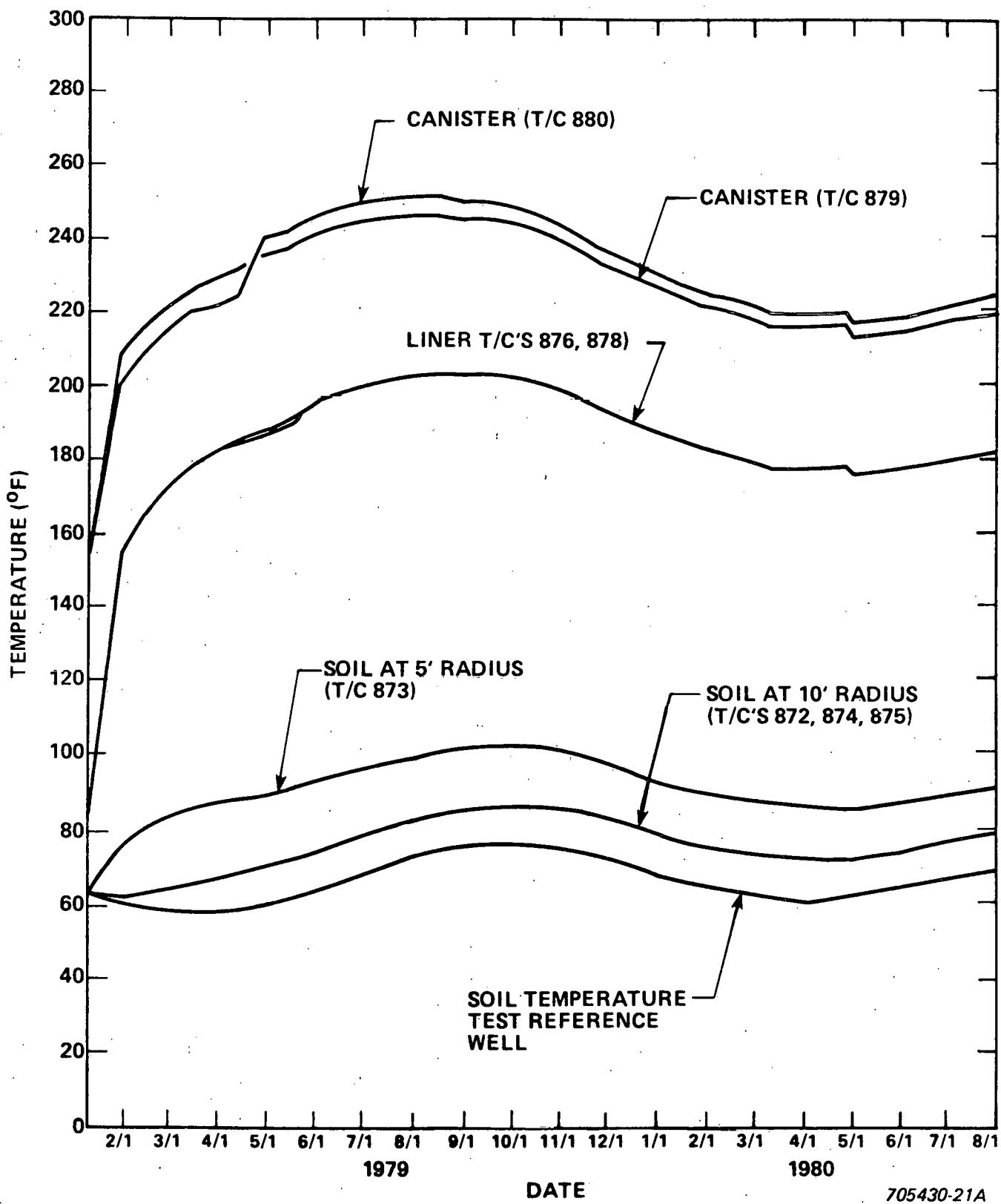
Figure C-7. Drywell 5 Canister, Liner, and Soil Temperature Distribution at About 145 Inches Below Ground Level
