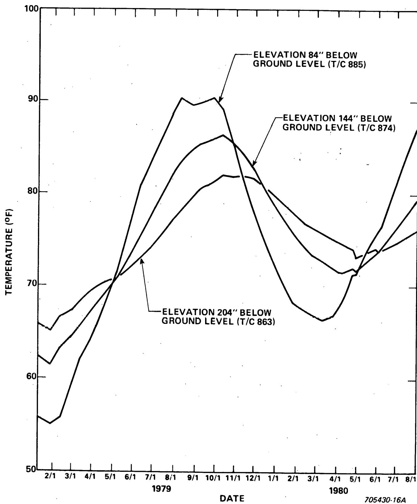
Figure 27. Drywell 5 Soil Temperature Distributions
