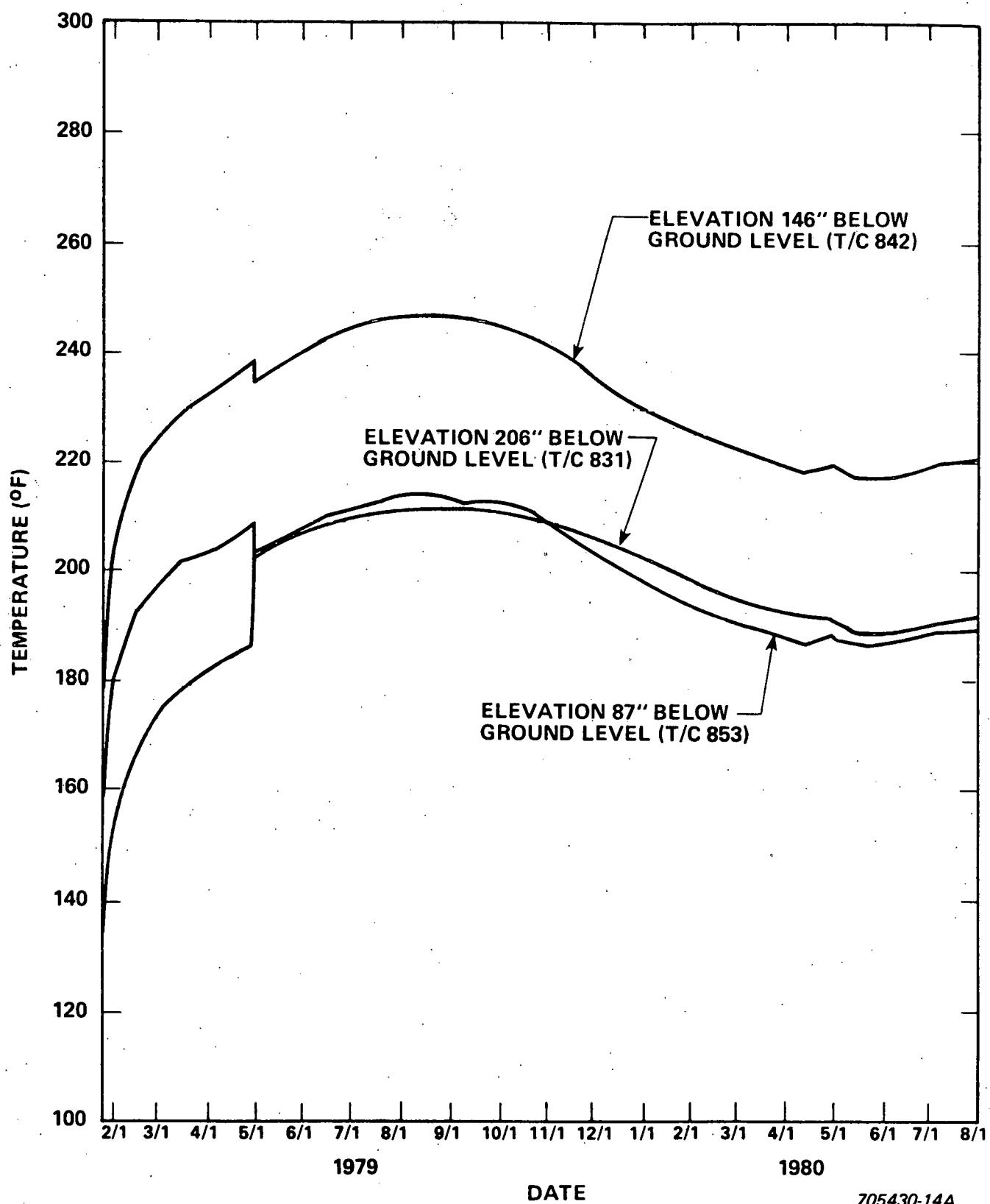
Figure 24. Drywell 3 Canister Temperature Distributions
