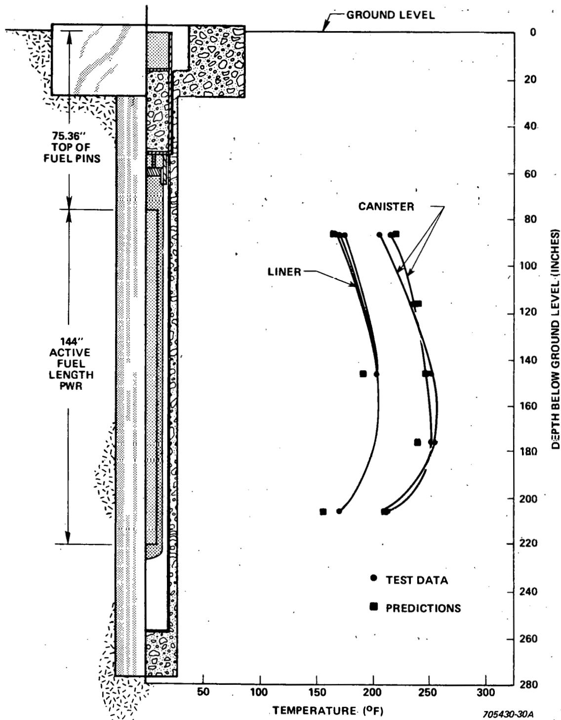
Figure 33. Drywell 5 Test Data and Predictions Comparison of Canister and Liner Axial Temperature Profiles
