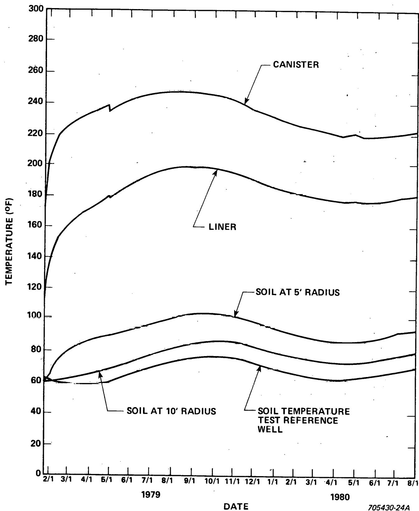
Figure 20. Drywell 3 Peak Canister, Liner and Soil Temperature Distributions
