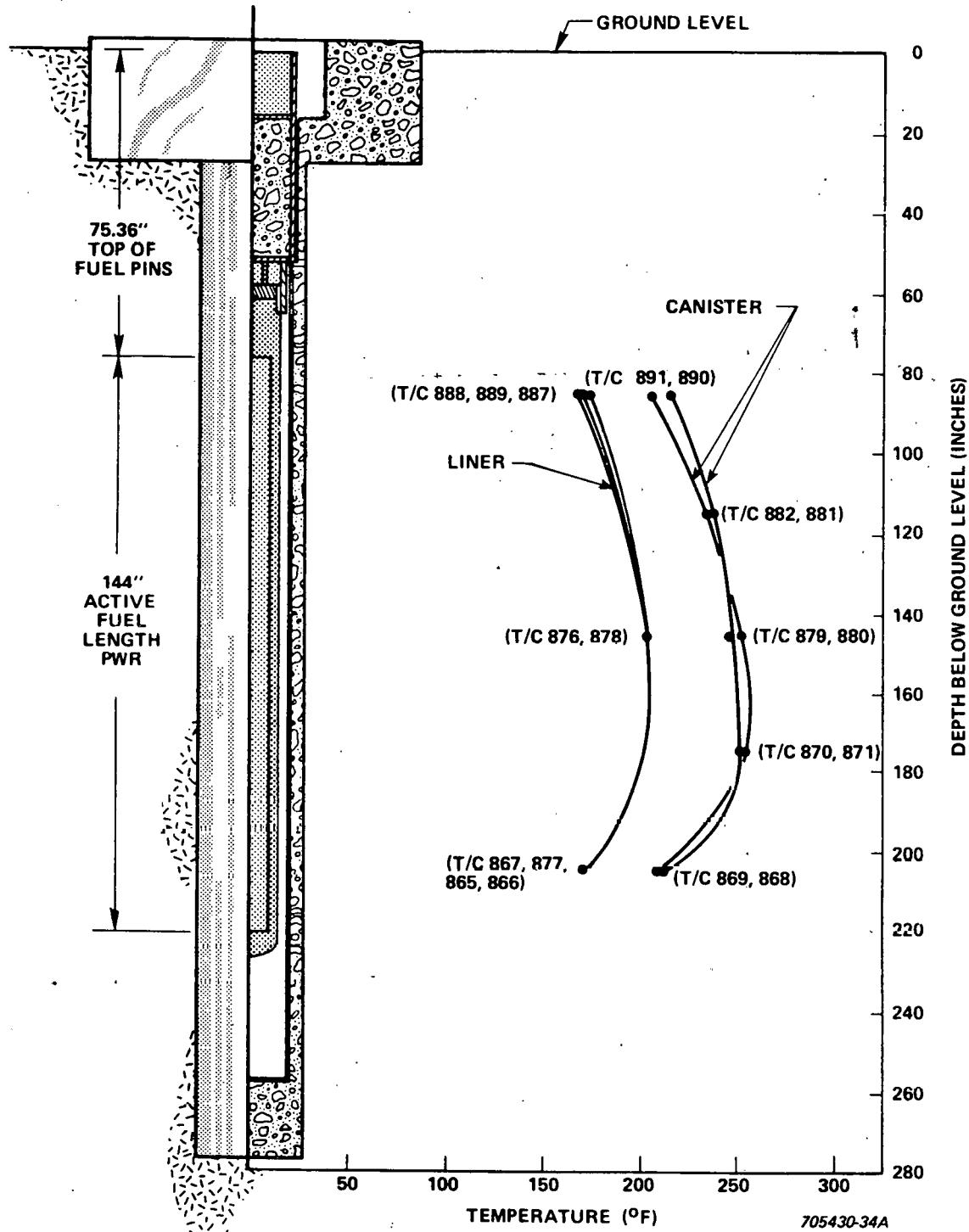
Figure C-12. Drywell 5 Axial Canister and Liner Temperature Profiles, August 15, 1979
