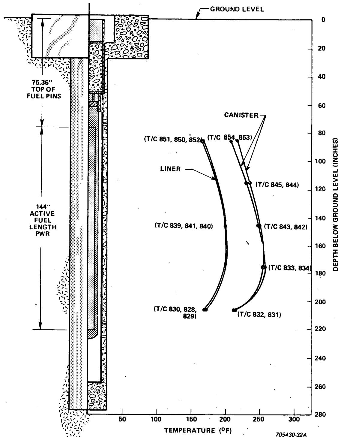
Figure C-11. Drywell 3 Axial Canister and Liner Temperature Profiles, August 15, 1979
