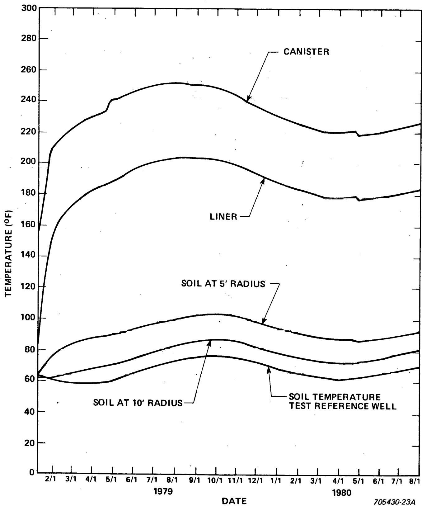
Figure 22. Drywell 5 Peak Canister, Liner and Soil Temperature Distributions
