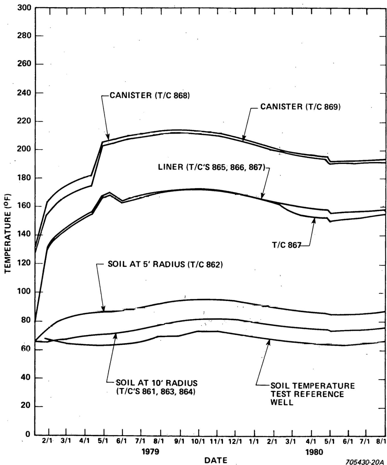
Figure C-8. Drywell 5 Canister, Liner, and Soil Temperature Distributions at About 205 Inches Below Ground Level
