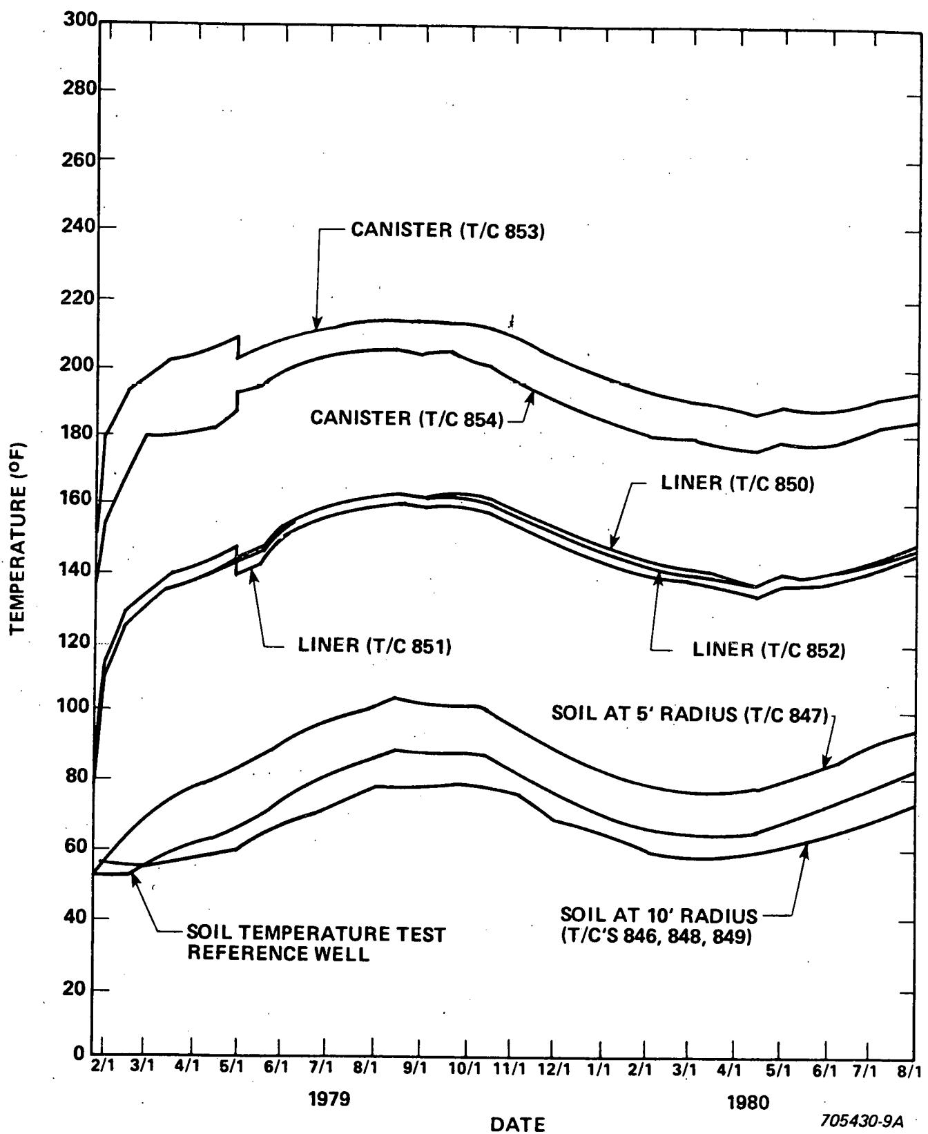
Figure C-1. Drywell 3 Canister, Liner, and Soil Temperature Distributions at About 85 Inches Below Ground Level
