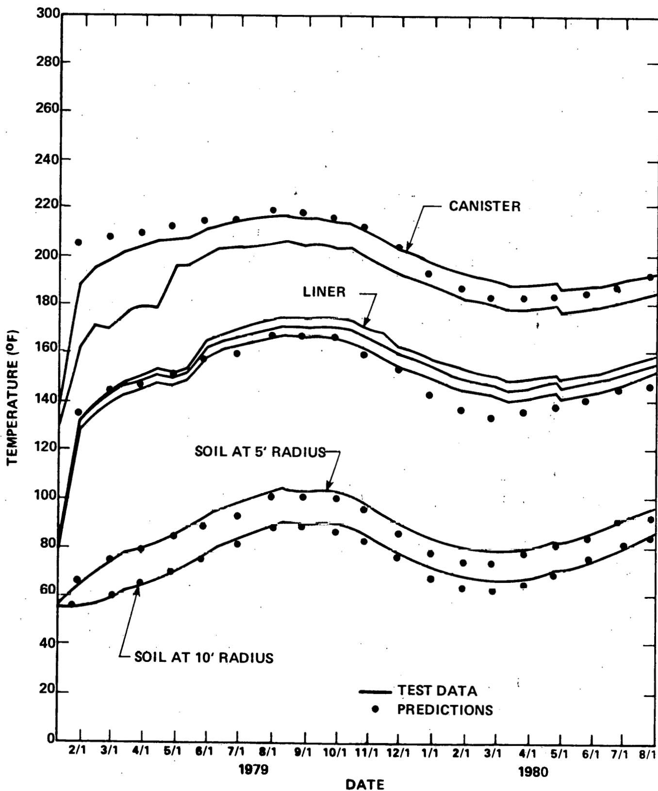
Figure 34. Drywell 5 Test Data and Predictions Comparison at About 85 Inches Below Ground Level
