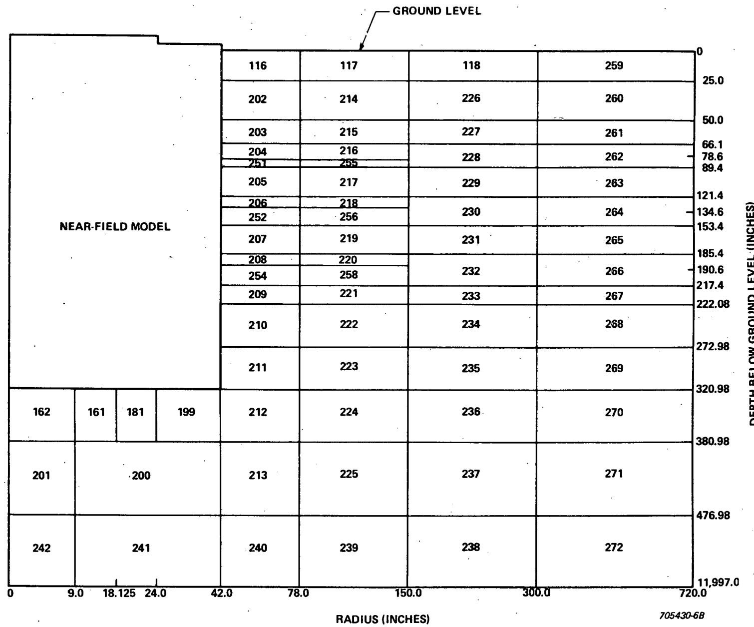
Figure 29. Far-Field Isolated Drywell Thermal Model
