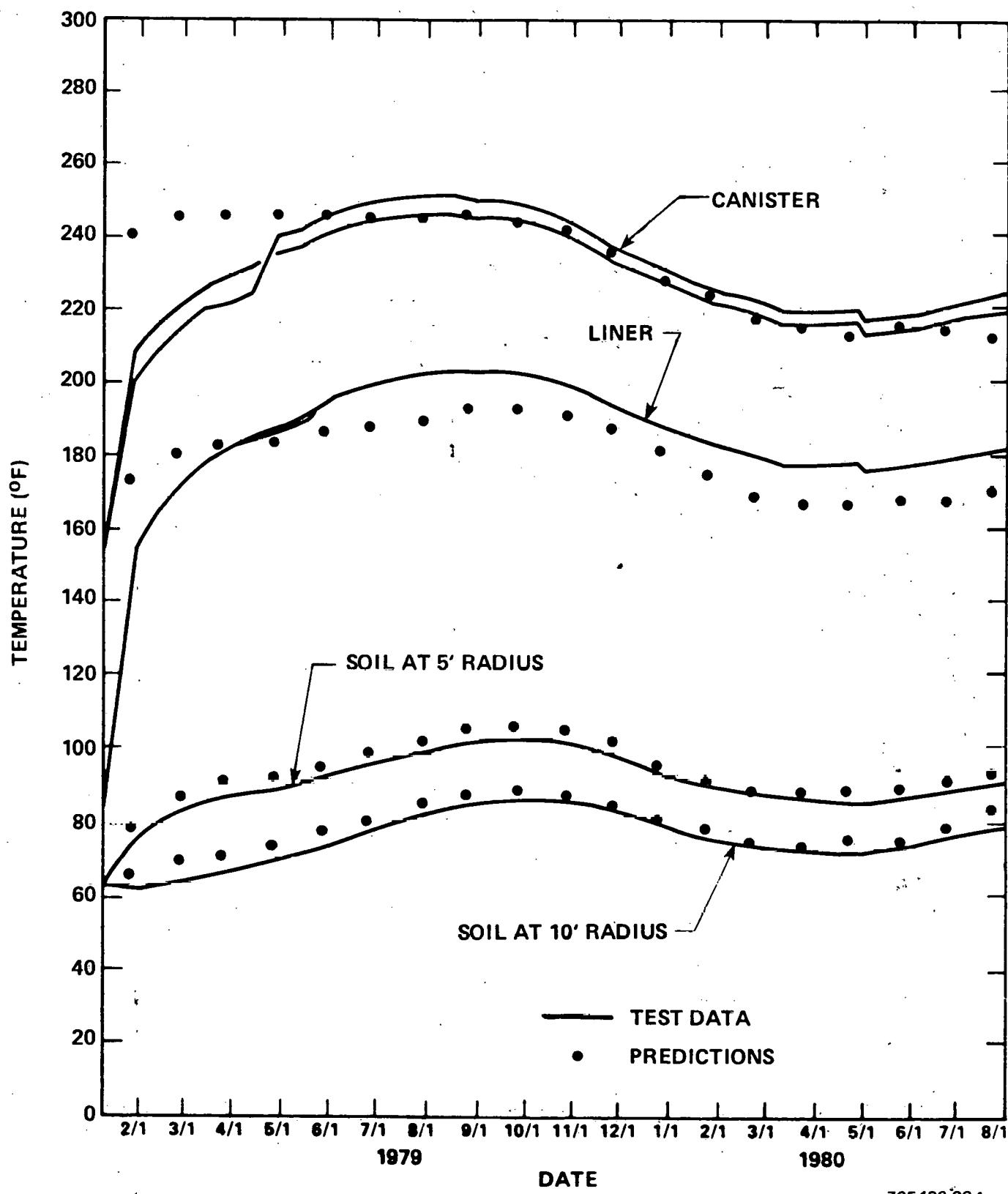
Figure 36. Drywell 5 Test Data and Predictions Comparison at About 145 Inches Below Ground Level
