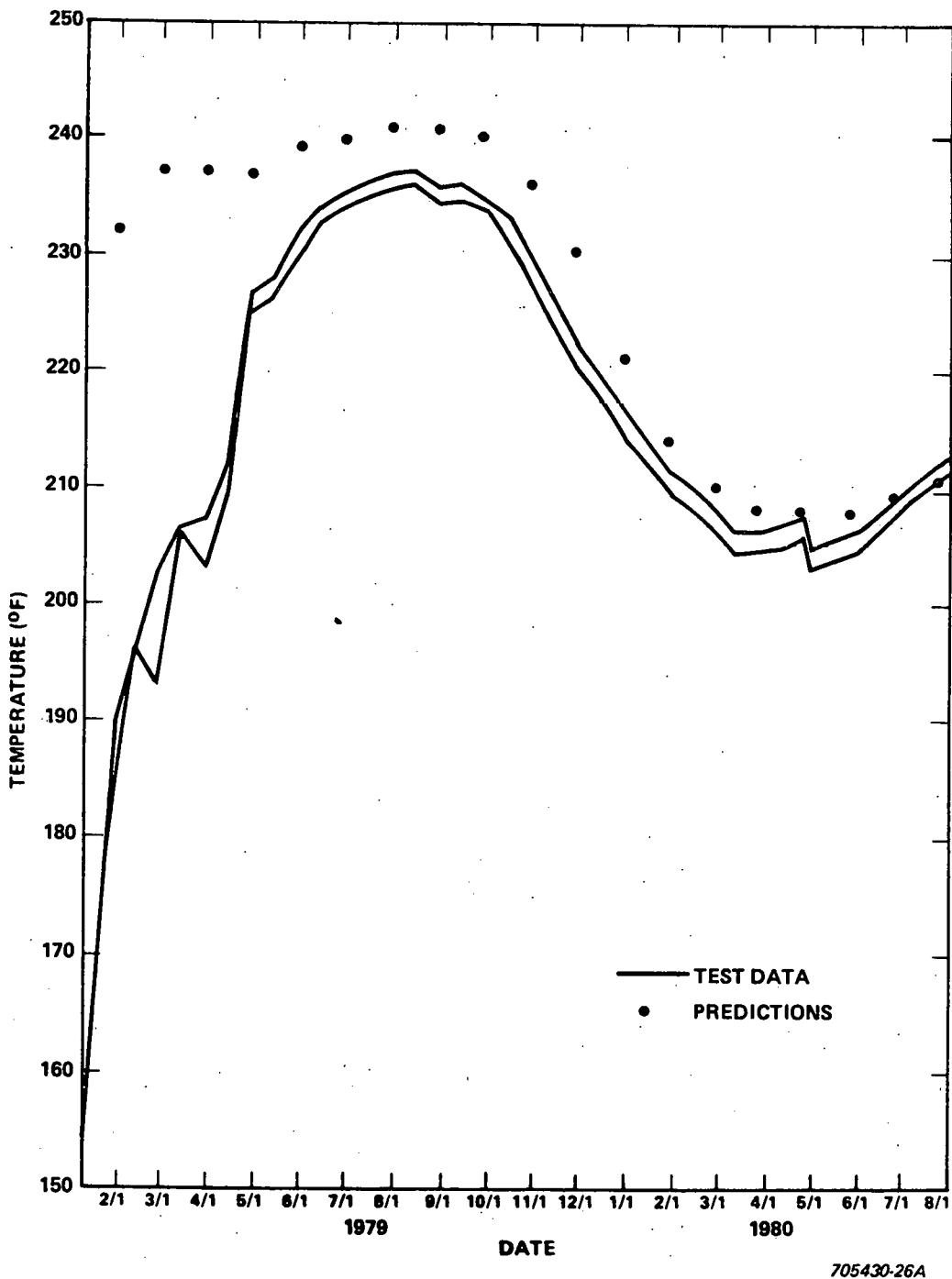
Figure 35. Drywell 5 Canister Test Data and Predictions Comparison at 116 Inches Below Ground Level
