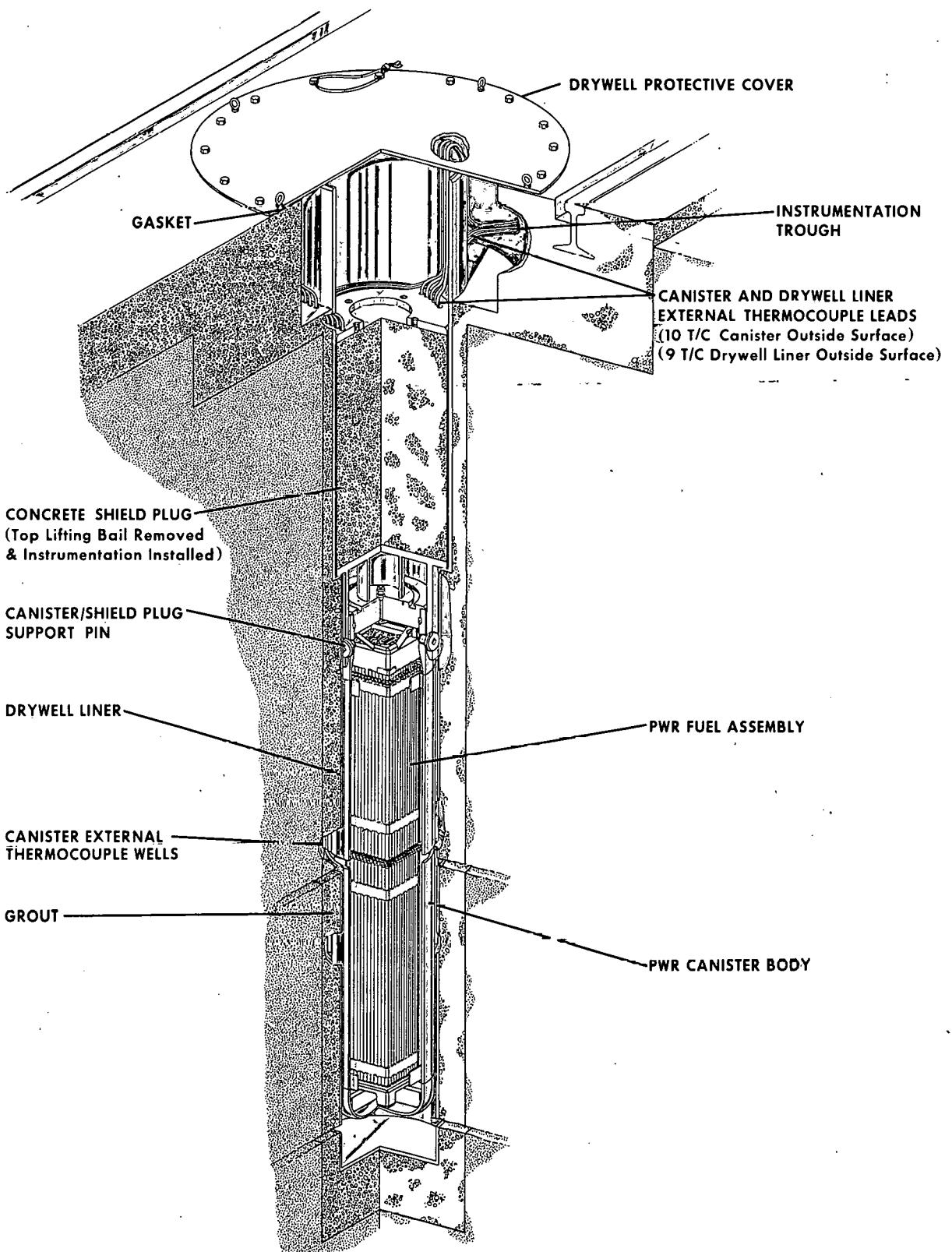
Figure 1. Drywell Configuration
