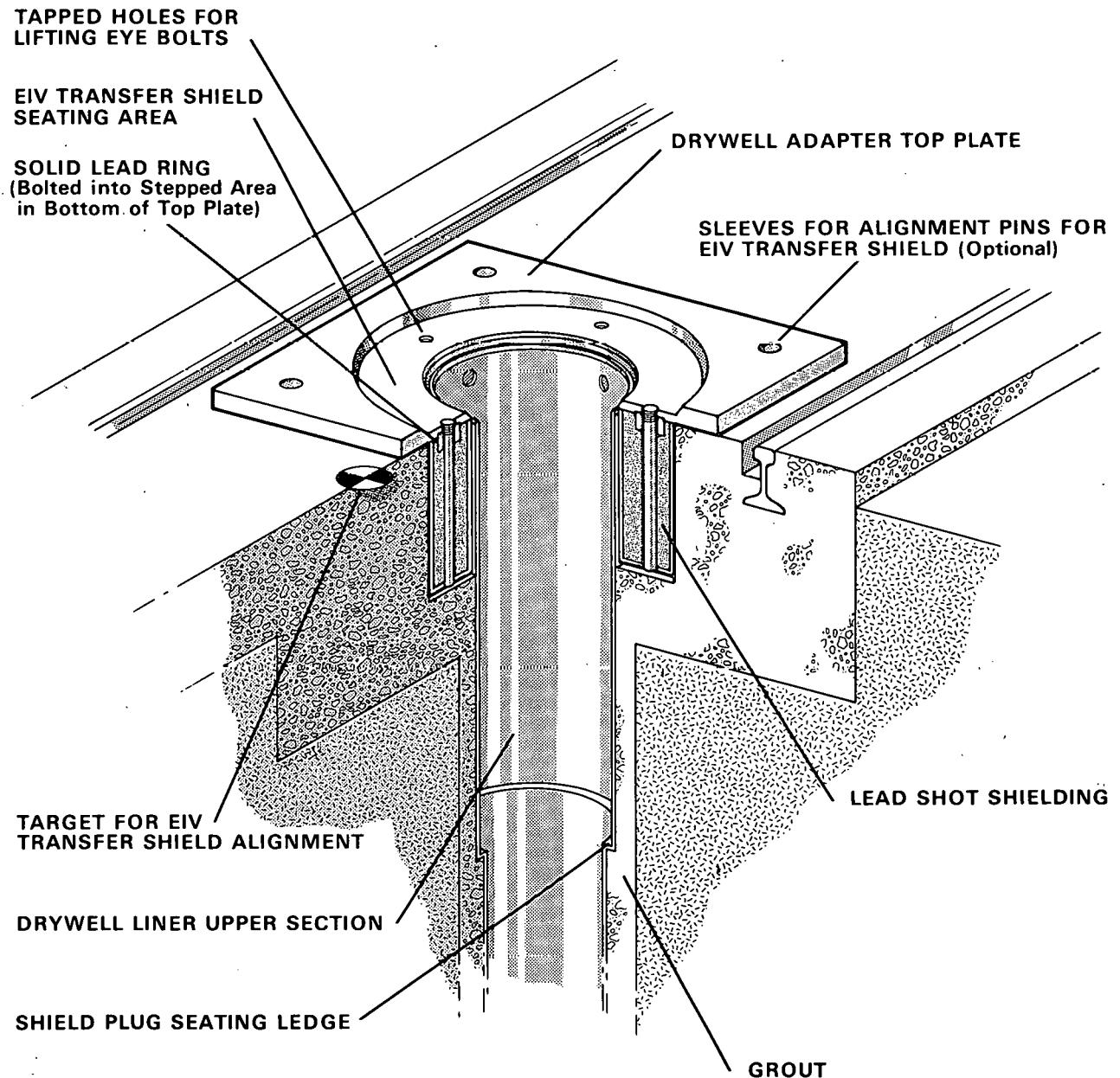
Figure 19. Drywell Shield Adapter Configuration (Shown Installed in Drywell)
