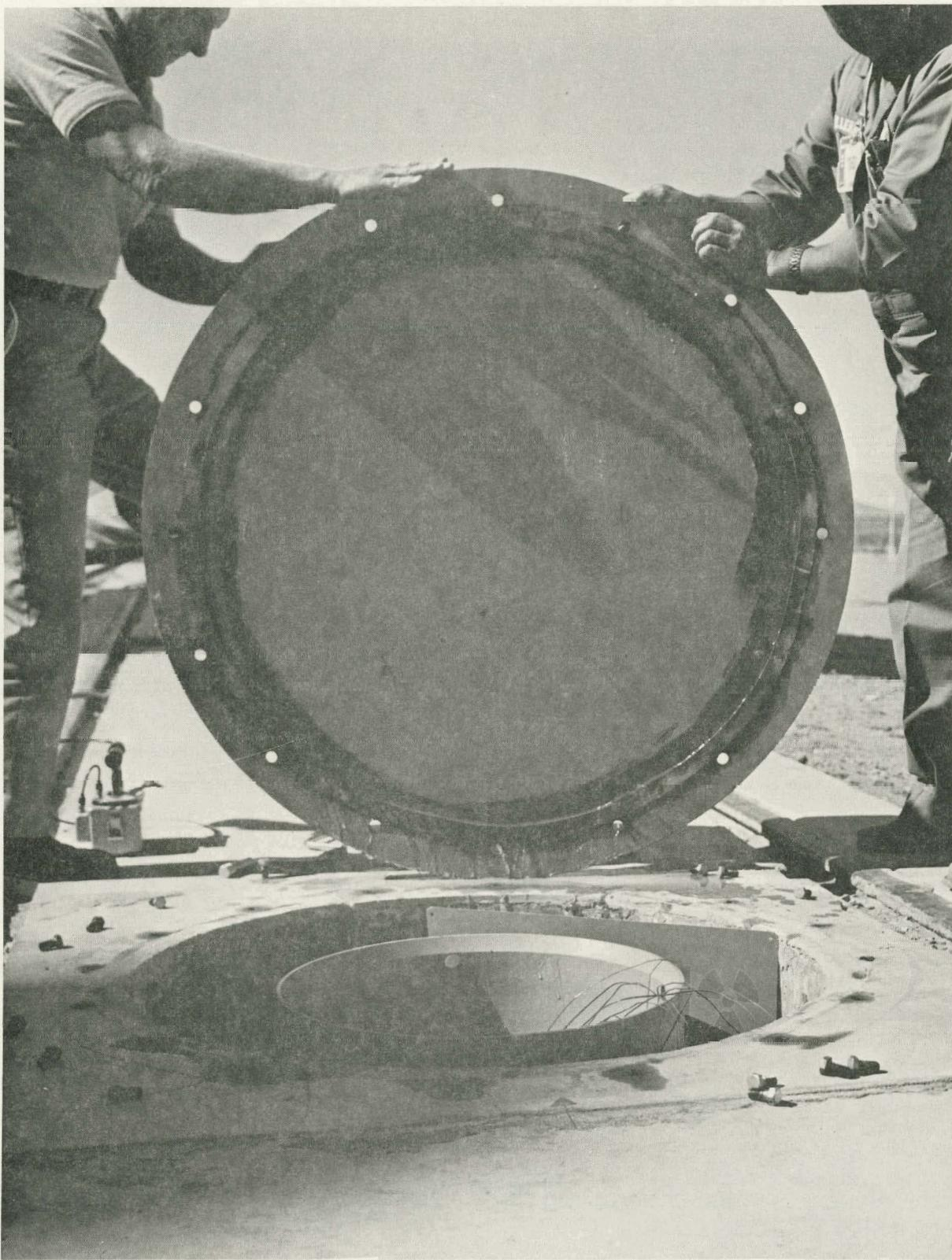
Figure A-18. Drywell 3 Cover Plate Removed After Isolated Drywell Test
