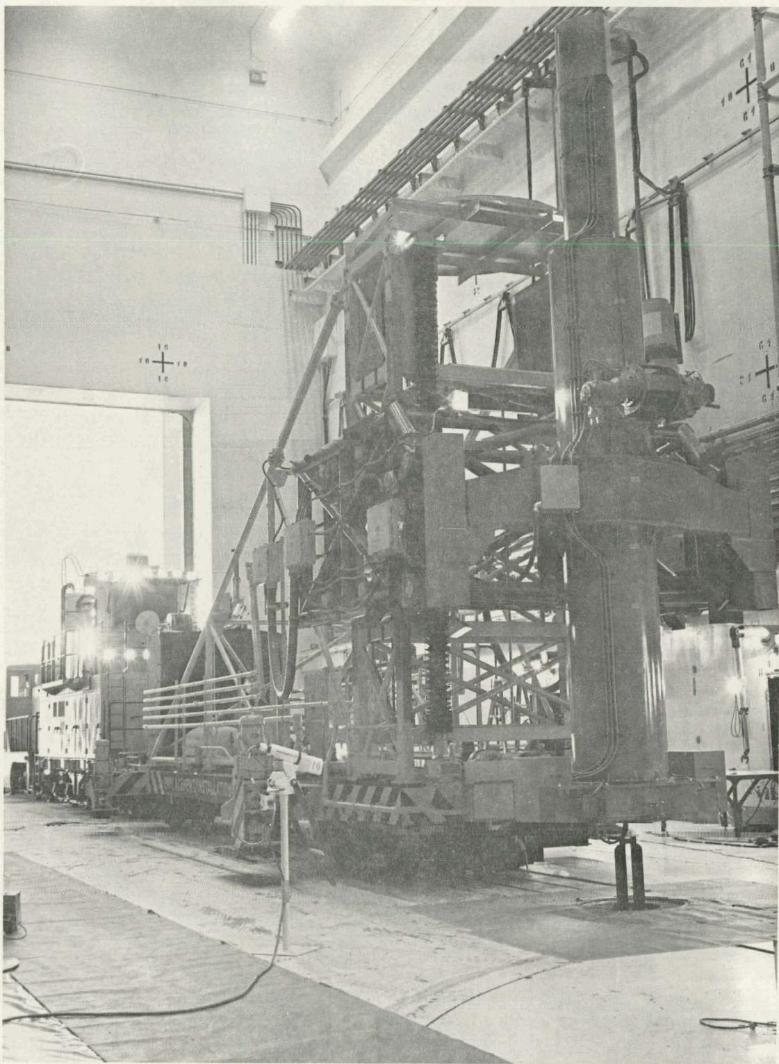
Figure A-10. Positioning Transfer Cask Over Hot Bay Transfer
