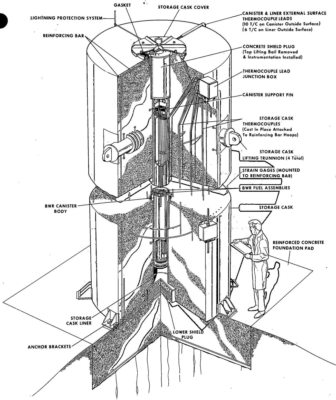
Figure 2. Surface Storage Cask Configuration
