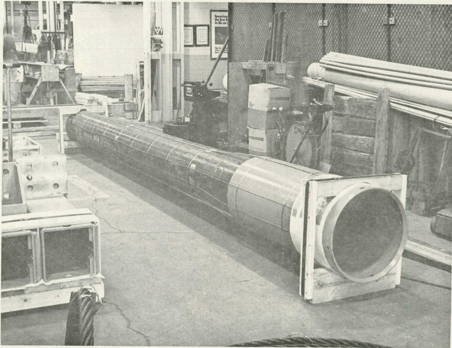
Figure A-1. Drywell Liner Prior to Shipment
