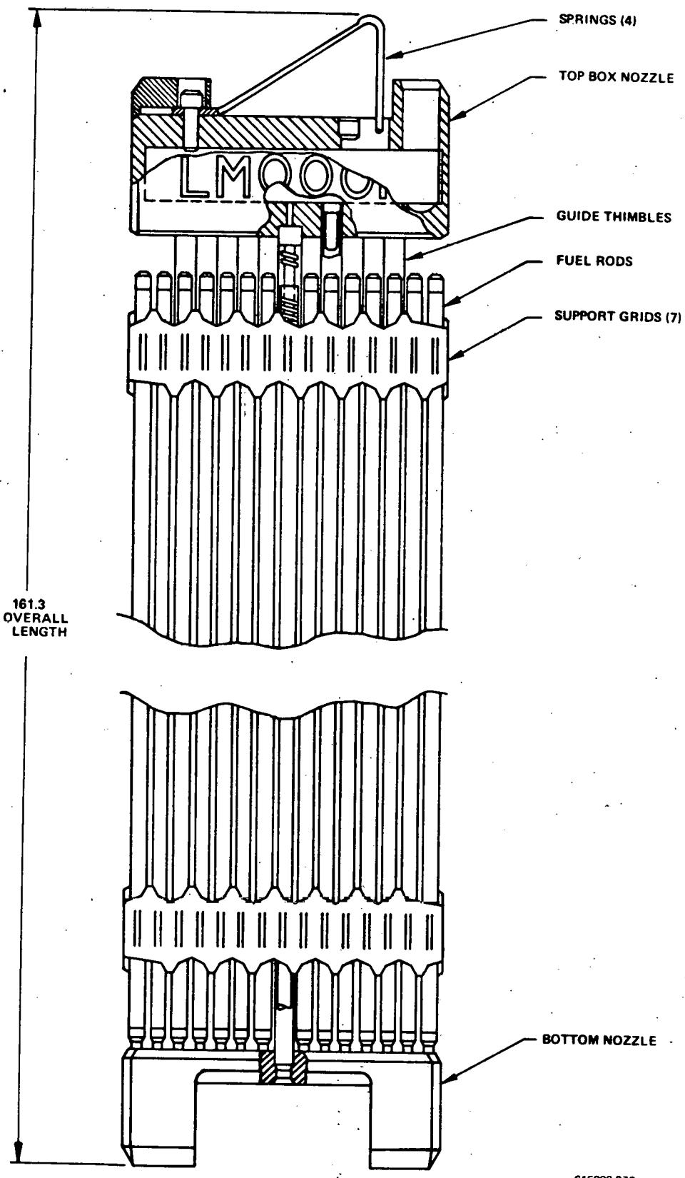
Figure 11. PWR Fuel Assembly Configuration
