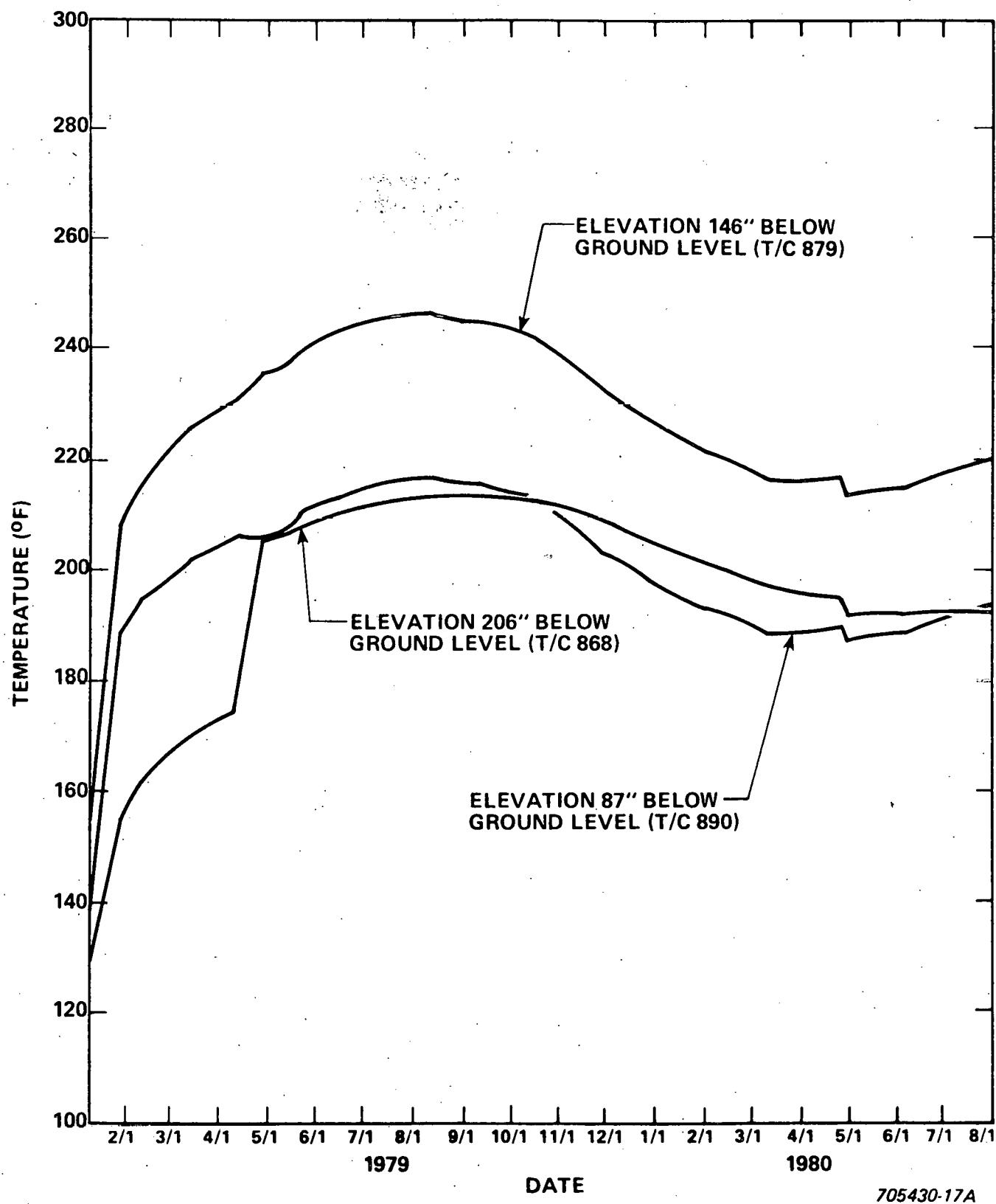
Figure 26. Drywell 5 Canister Temperature Distributions
