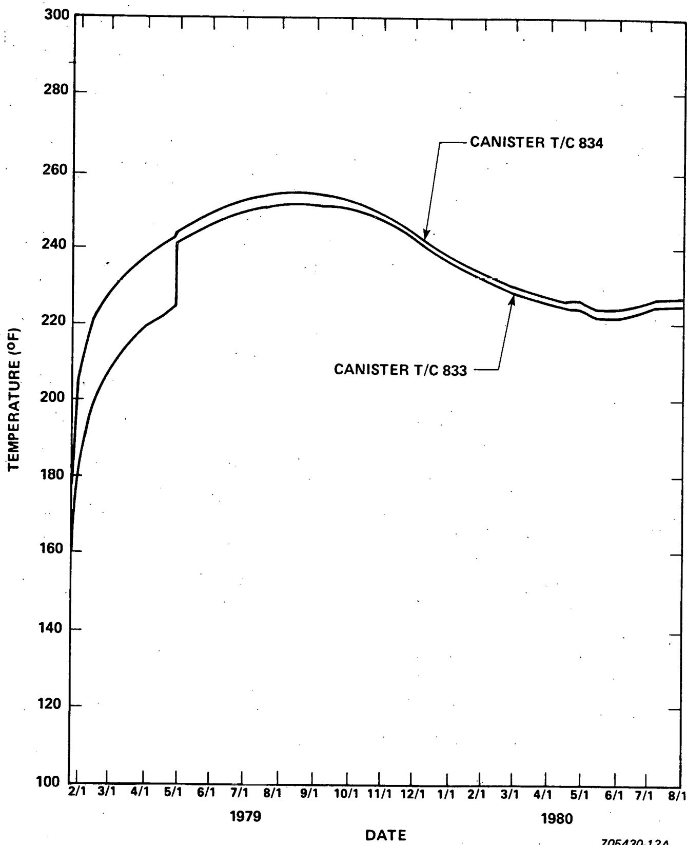
Figure C-5. Drywell 3 Canister Temperature Distribution at 176 Inches Below Ground Level
