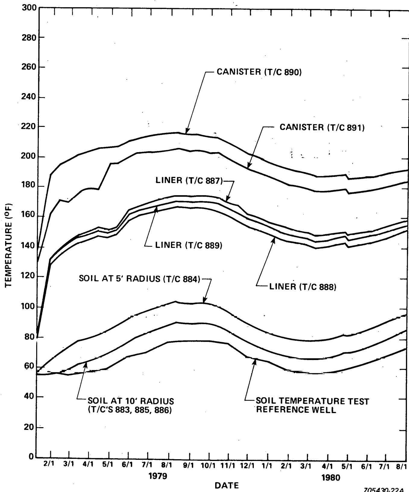
Figure C-6. Drywell 5 Canister, Liner, and Soil Temperature Distributions at About 85 Inches Below Ground Level
