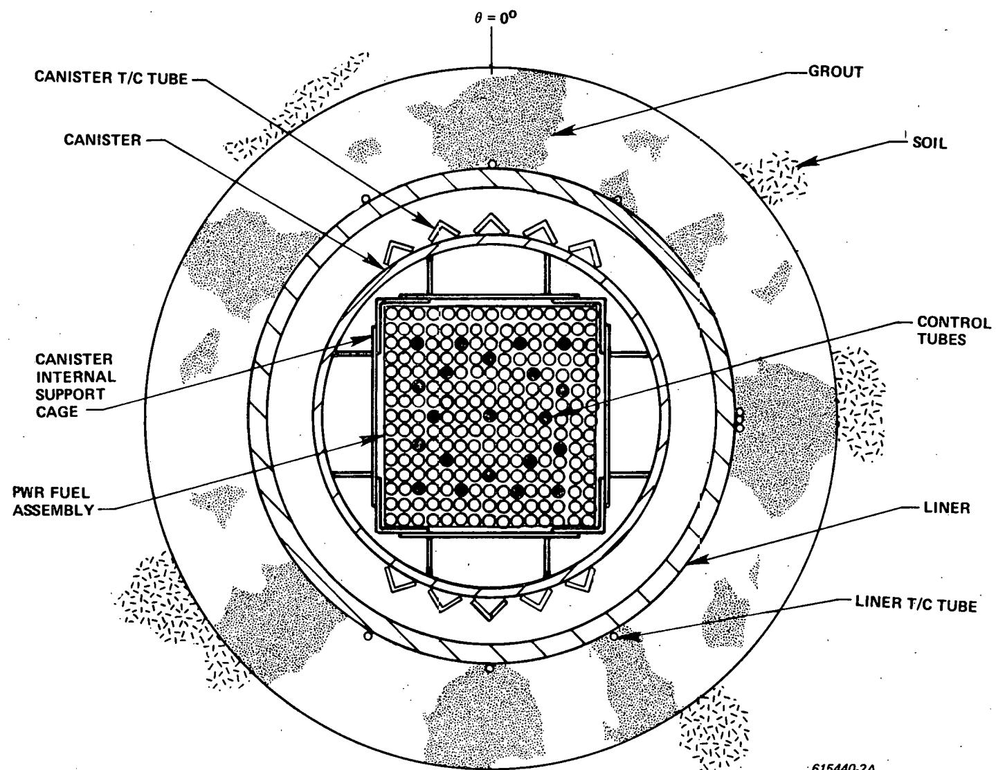
Figure 6. Drywell Section View
