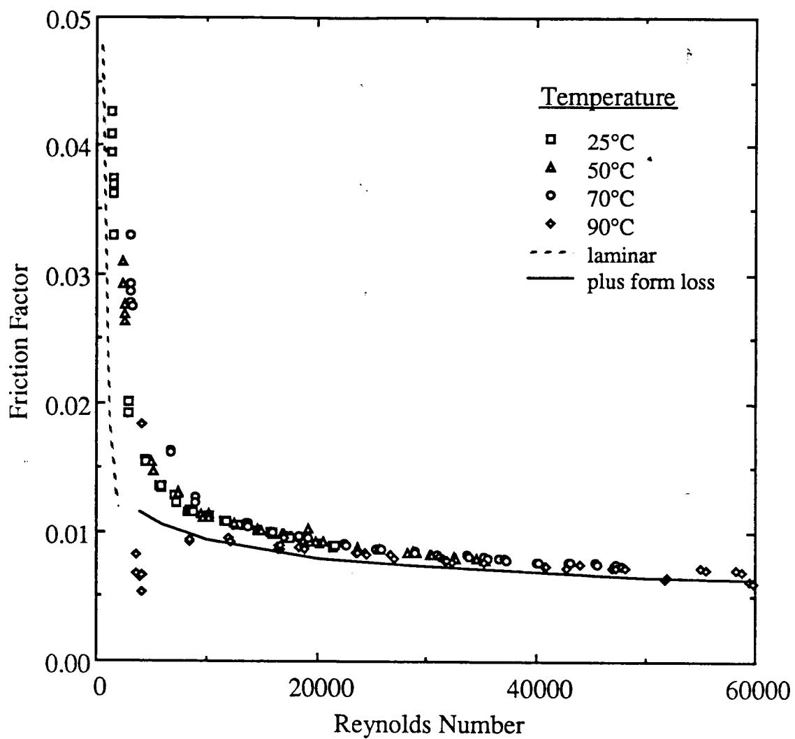
**Fig. 2 Test section friction factor for unheated experiments**
