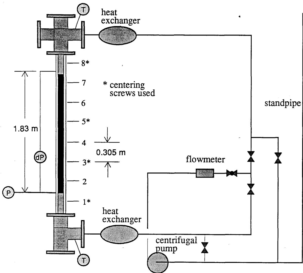
Fig. 1 Schematic of flow loop showing instrumentation and location of centering screws
