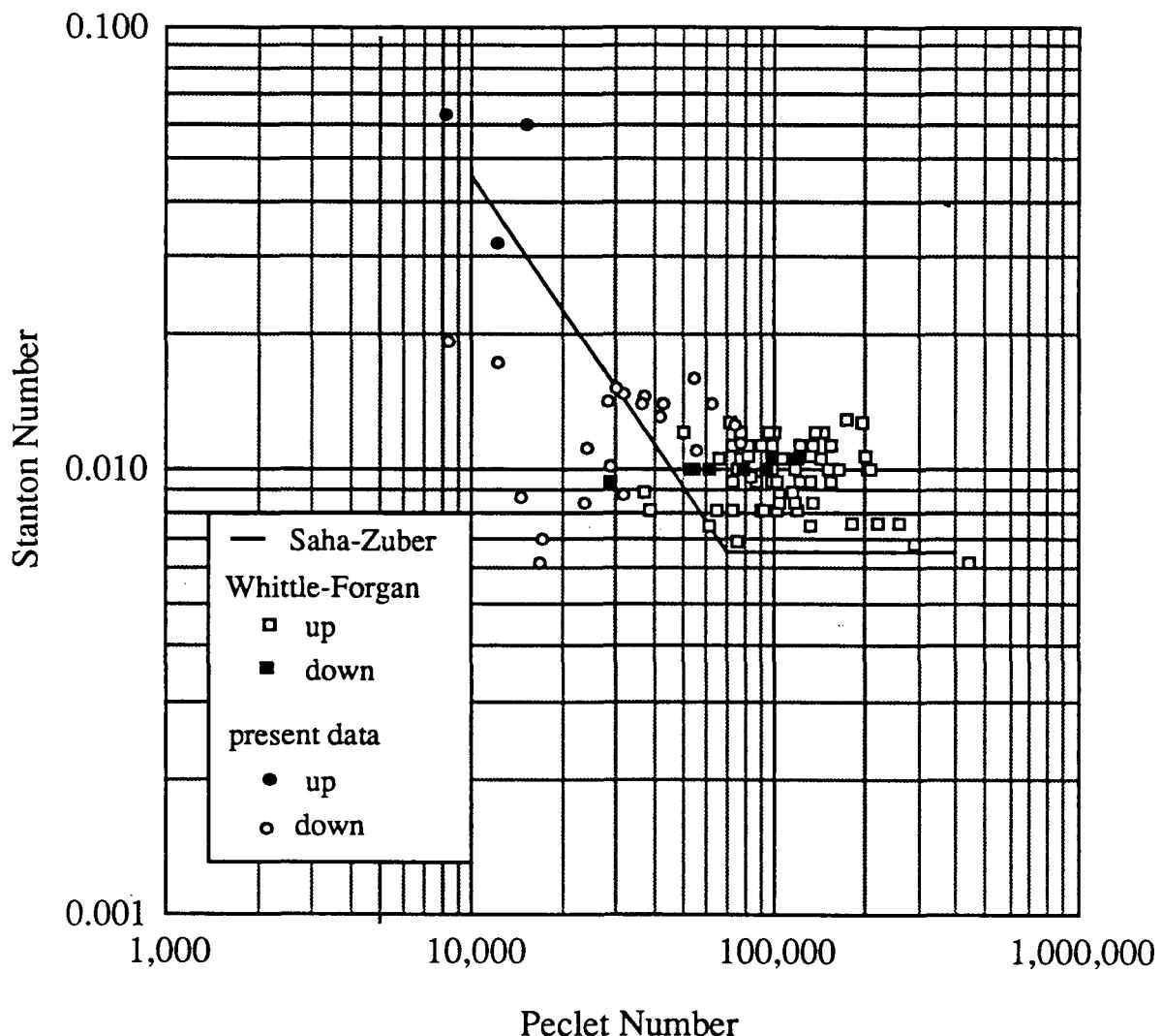
**Fig. 9** Minima of demand curves from experiments of Whittle and Forgan (1967) compared to present data and correlation of Saha and Zuber (1974)
