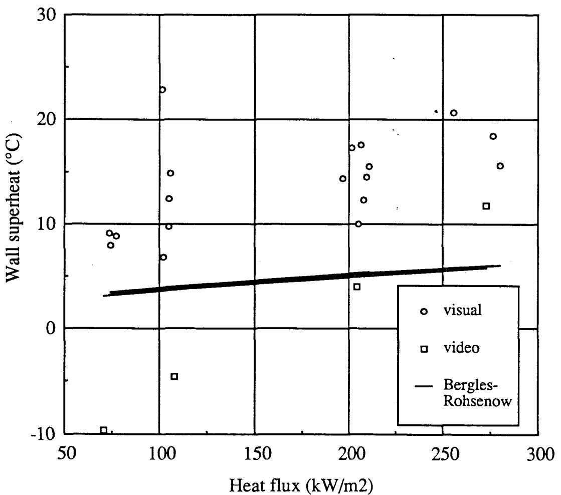
**Fig. 4** Wall temperature at first appearance of bubbles compared to the correlation of Bergles and Rohsenow (1964)
