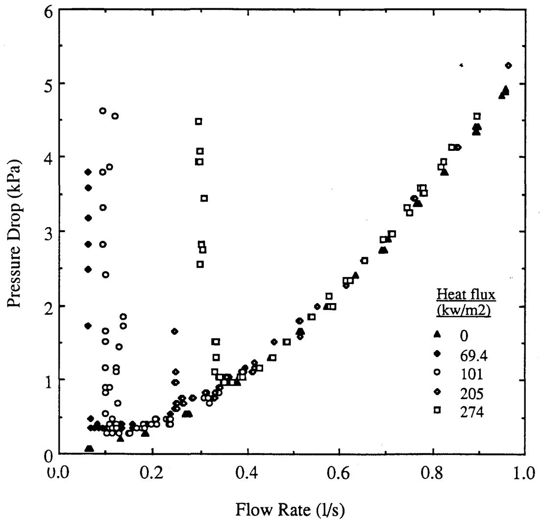
Fig. 6 Test section demand curves at 70 °C inlet temperature
