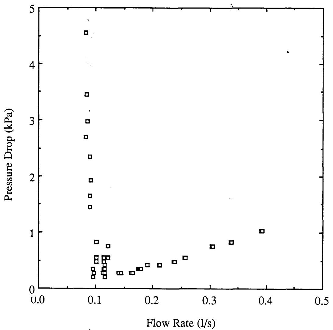
**Fig. 8 Demand curve showing multiple rise in pressure drop**
