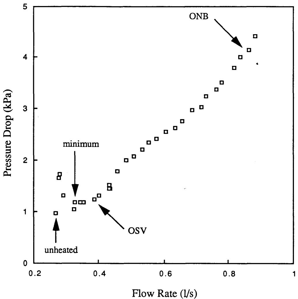
Fig. 3 Demand curve for 205 kW/m<sup>2</sup> and 80°C inlet temperature
