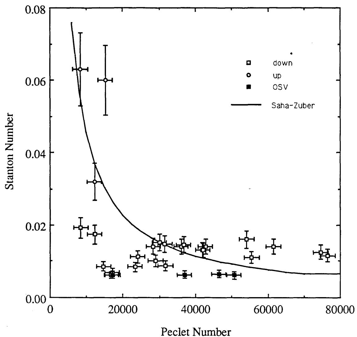
**Fig. 7** Demand curve minima plotted as Stanton and Peclet numbers, compared with OSV data and the correlation of Saha and Zuber (1974)
