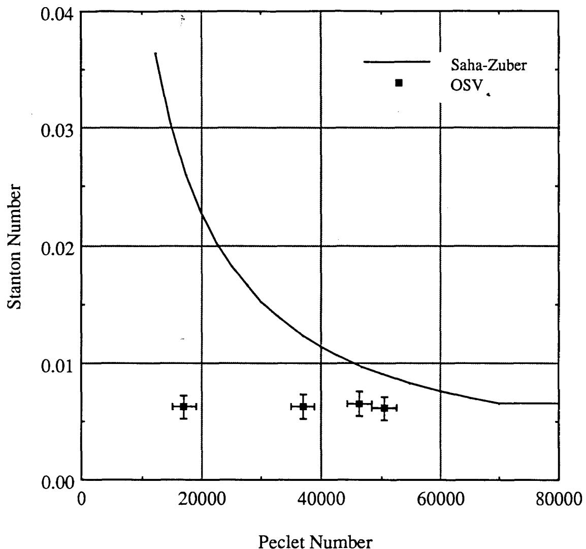
Fig. 5 Conditions at the onset of significant void (OSV) expressed as Stanton and Peclet numbers, compared to correlation of Saha and Zuber (1974)
