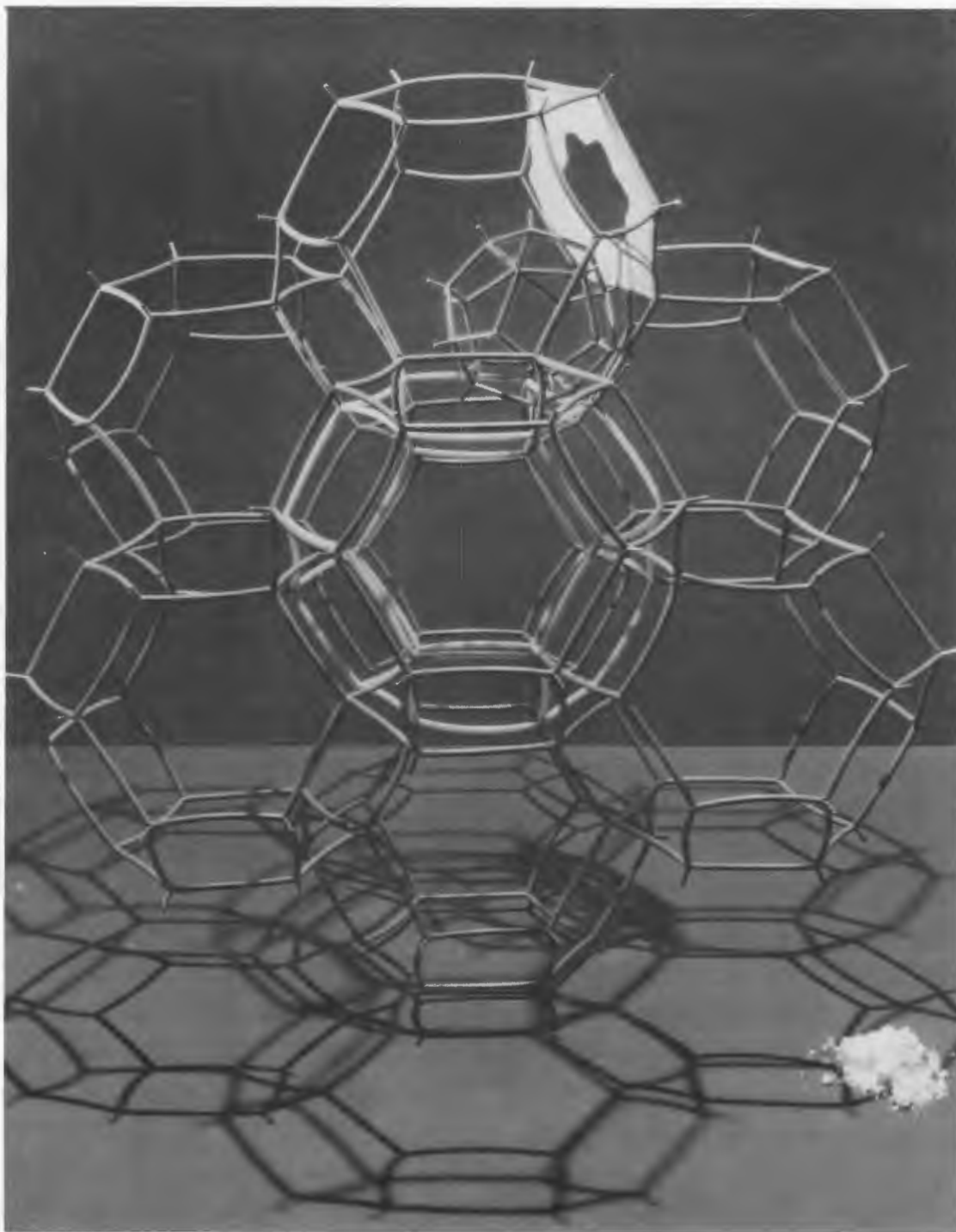
Figure B-1. Model of sodalite cages. Relative cage opening shown in upper right of cage containing model of krypton atom.
