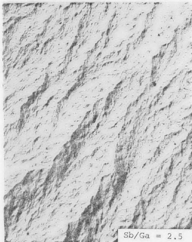
Fig. 13. Surface morphology of continuously graded AlGaAsSb/GaAs (111)A grown from solutions with different Sb concentrations. 110X
