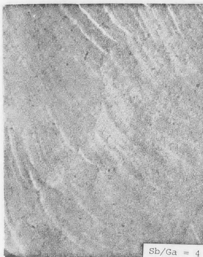
Fig. 13. Surface morphology of continuously graded AlGaAsSb/GaAs (111)A grown from solutions with different Sb concentrations. 110X
