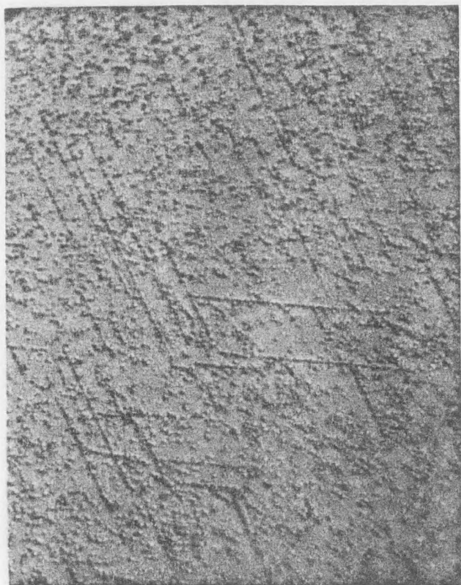
Fig. 16. Dislocation densities observed before and after growth of GaAsSb/AlGaAsSb (graded) layers Sb/Ga = 4. #42878A Substrate dislocation density: Column I 1.7 \times 10^4 \text{ cm}^{-2} Column II 9.7 \times 10^4 \text{ cm}^{-2}
