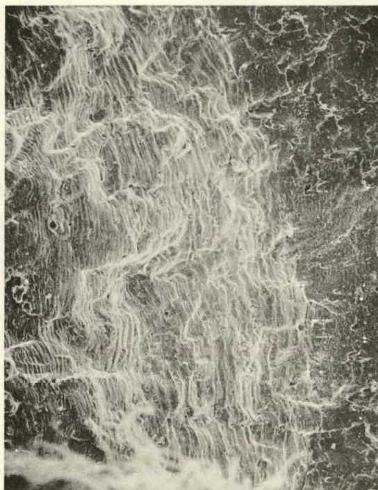
Fig. 33. Scanning Electron Micrograph of the Fractured Surface of Test No. 1044. Neg. No. MSD-66263.
