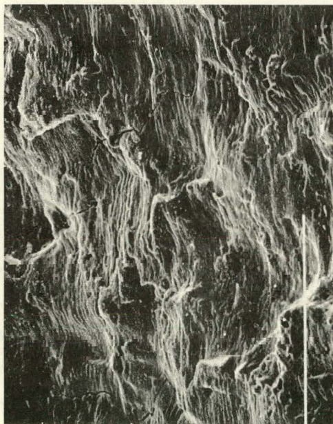
Fig. 34. Scanning Electron Micrograph of the Fractured Surface of Test No. 1033. Neg. No. MSD-66262.
