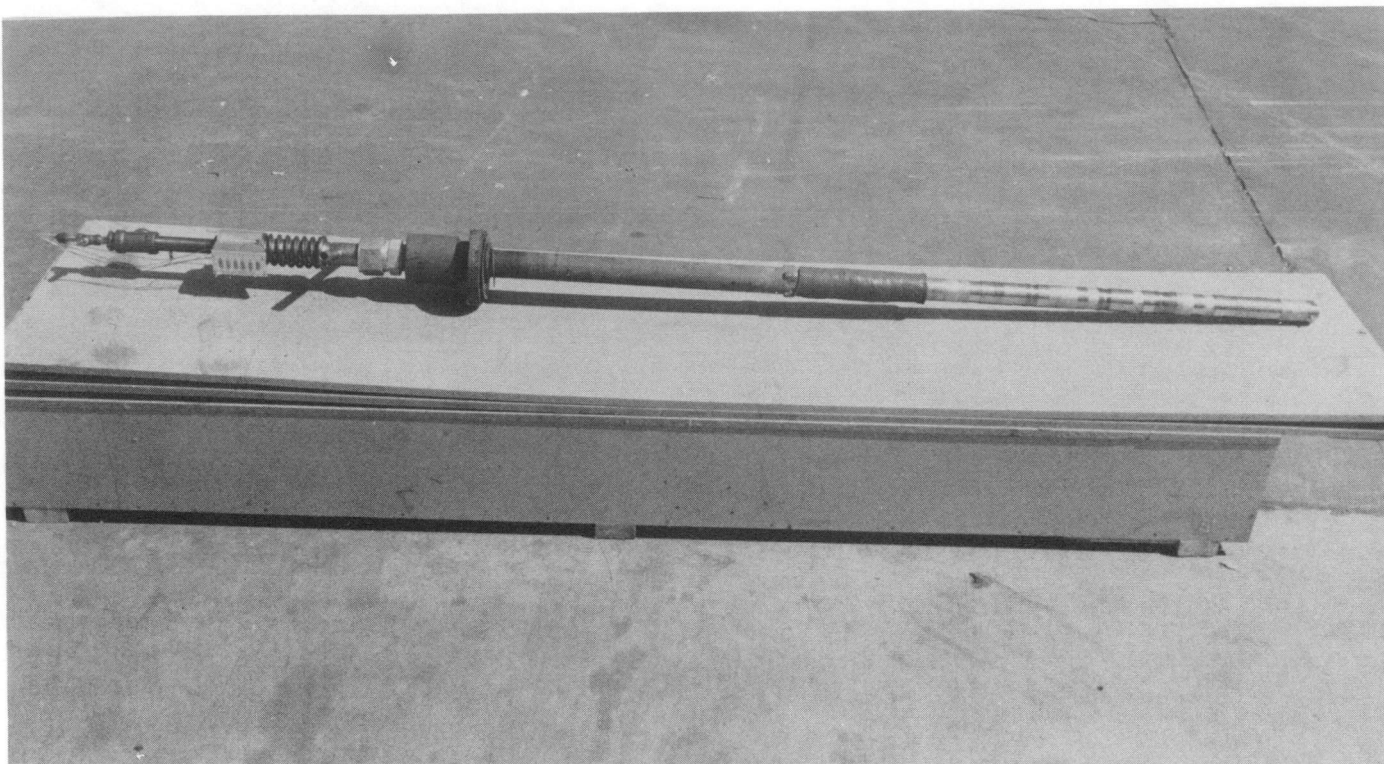
Figure C-23. Complete Material Specimen Probe Assembly
