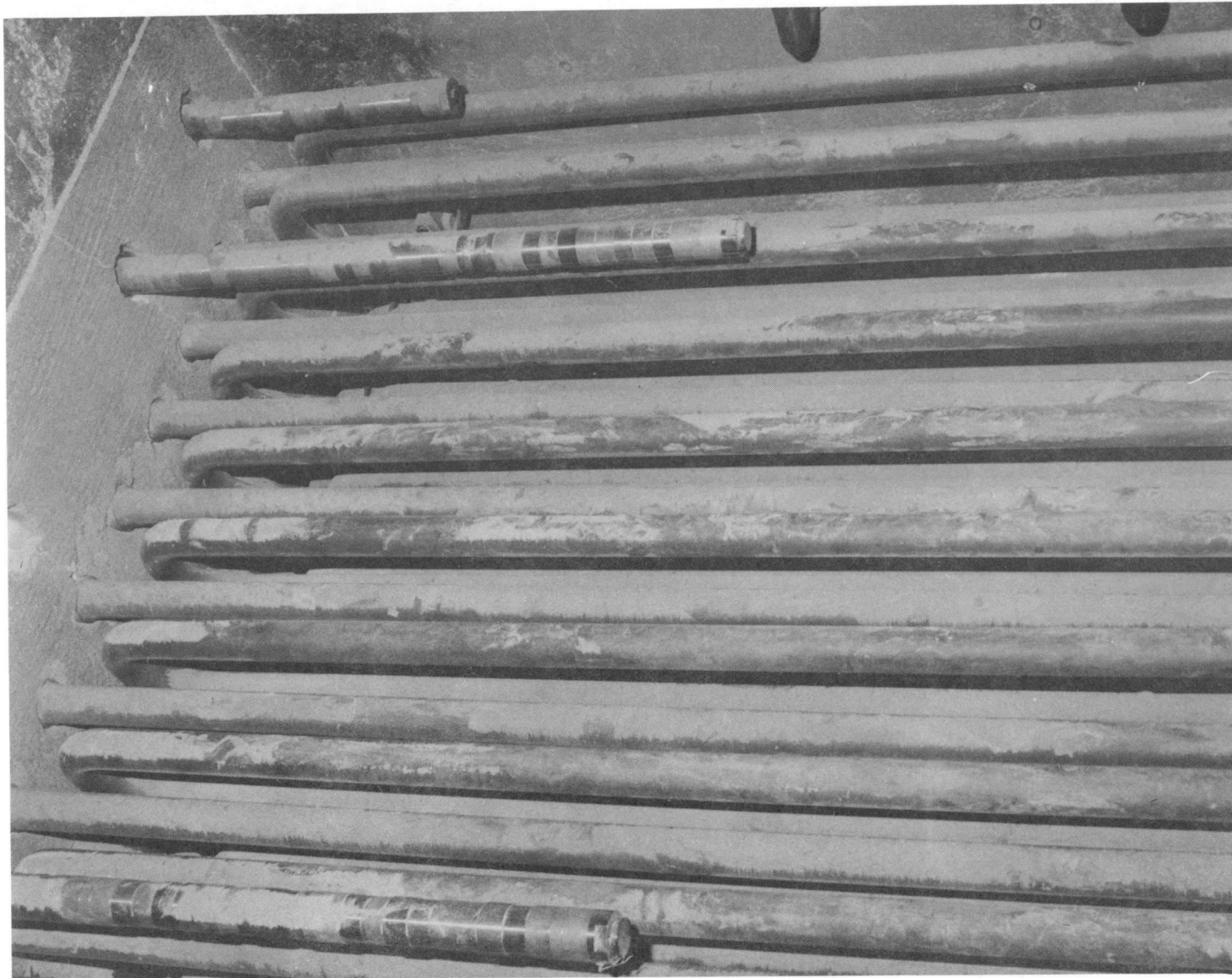
Figure C-30. Post-Run View of Material Specimen Probes Installed Above the Bed Heat Exchanger (uncooled surface penetration probes partially visible at top of photograph)
