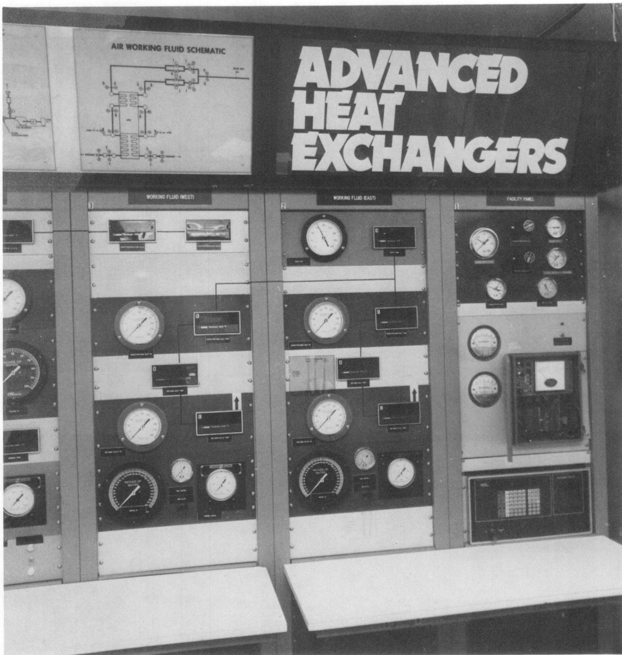
Figure C-35. Control Room Panels (left and center panels have the two working fluid systems; right panel has another in situ oxygen meter in the middle while the Autodata recorder is at the bottom.
