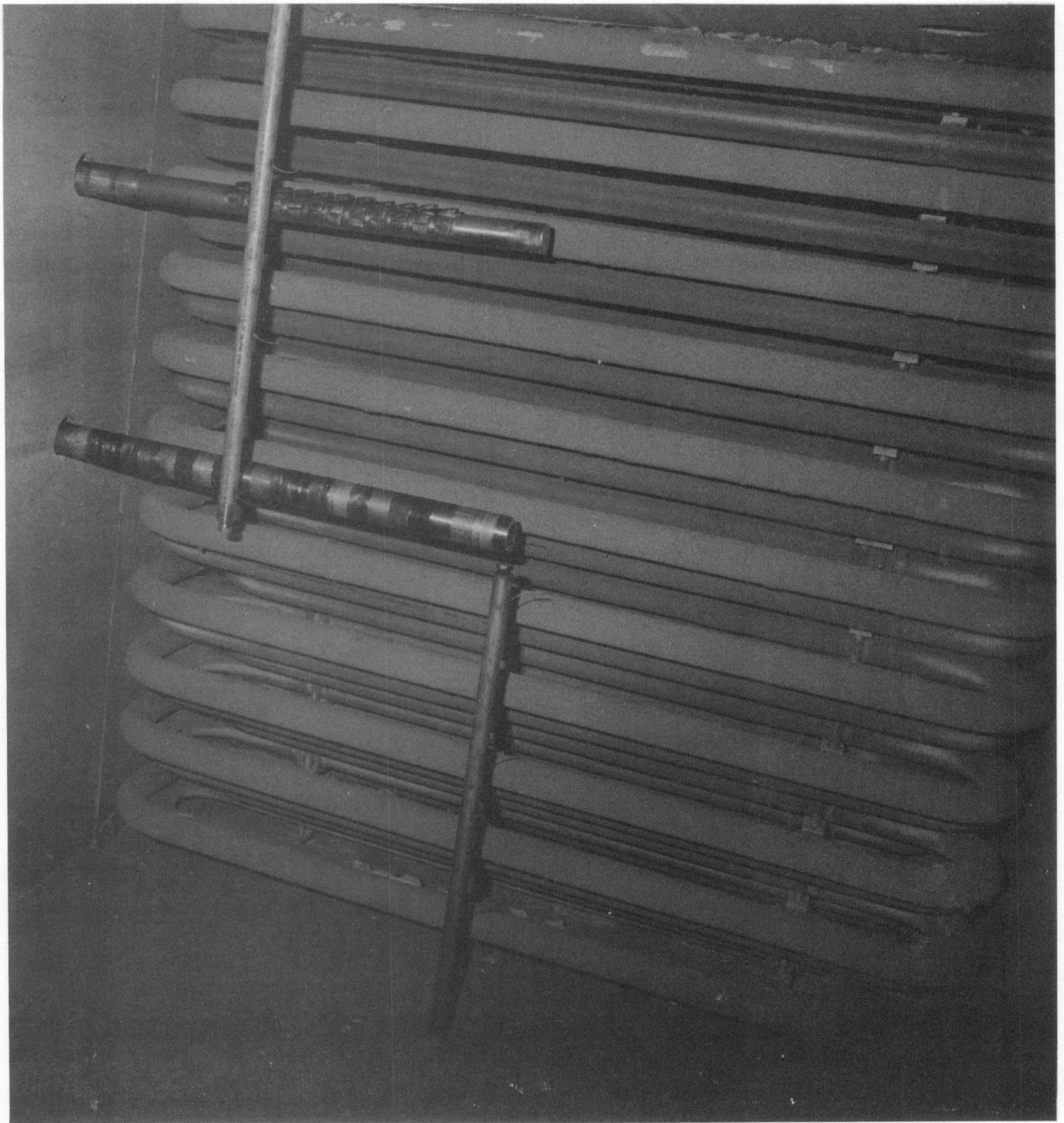
Figure C-31. View Looking Up at Material Specimen Probes Installed Below Convection Heat Exchanger (shown is a cooled ring probe, uncooled hanger specimen probe, and two temperature rake probes)
