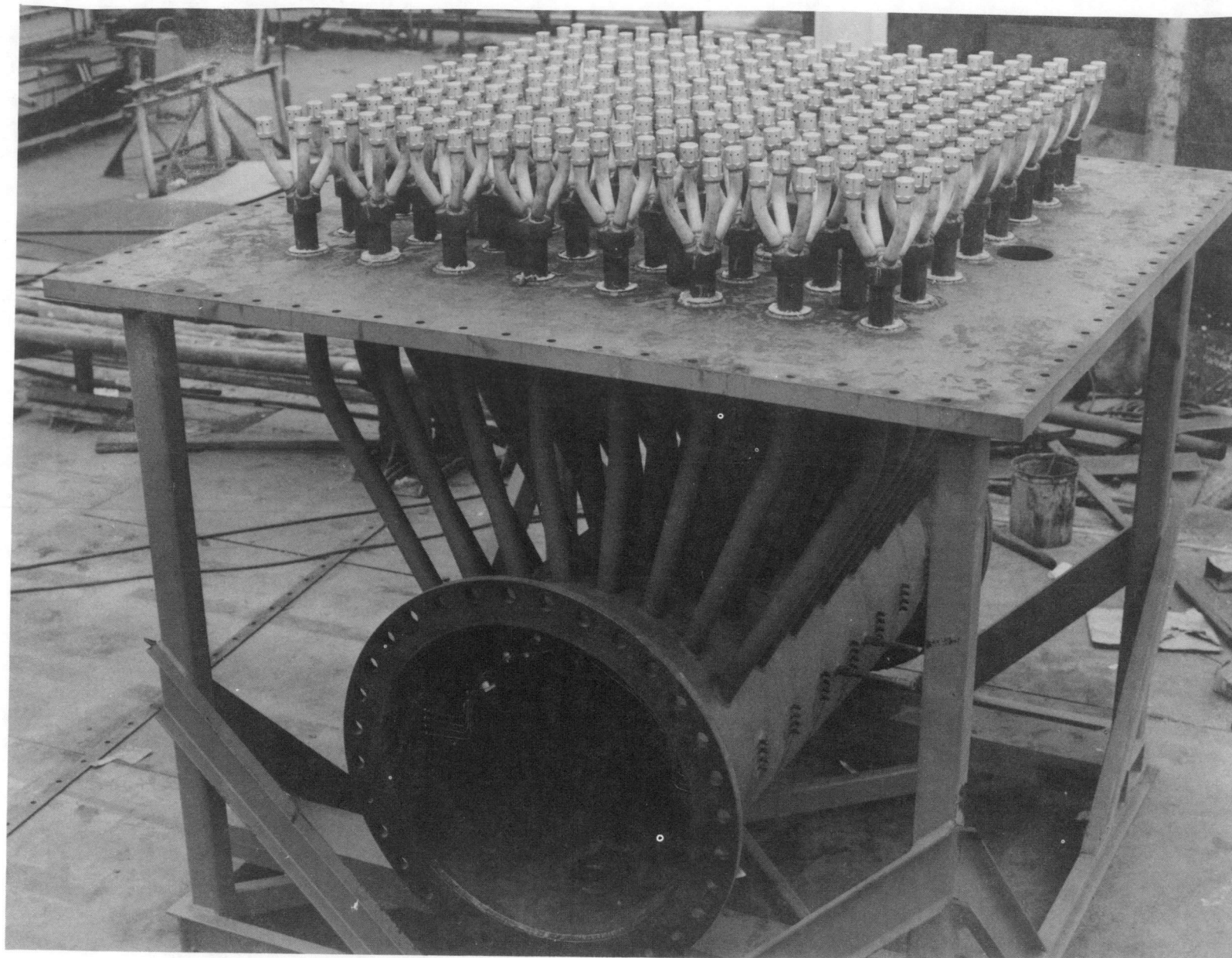
Figure C-13. Distributor Section During Fabrication (small lines in the windbox are for measuring flow in each feedline)
