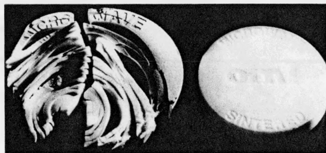
Figure 5. Zirconia-3 mole percent yttria discs sintered at 2.45 GHz (left) and 28 GHz (right). Right disc is 6.4 mm thick by 44.5 mm diameter.
