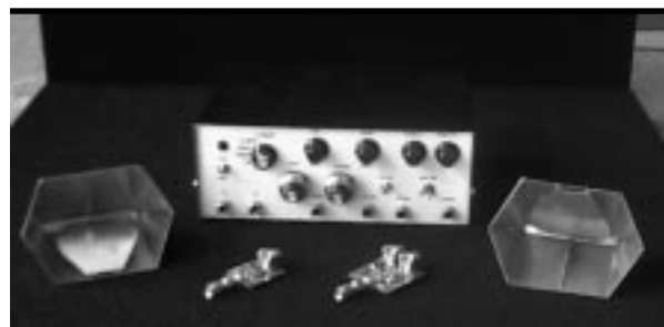
Figure 3. The modular MIR system: transmitter module, receiver module (front), two antennas (sides), and the timing and control unit (back).
