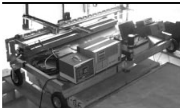
Figure 1. Calibrated Autonomous Radar Testbed (CART) for data acquisition using the MIR.
