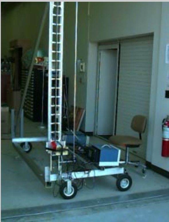
Figure 2. The CART in vertical mode, used for scanning large objects such as crates or containers, walls and other vertical objects. This mode also provides side-scanning SAR capability. The 3-D rendered images on the right are from cinder-block walls backfilled with pebbles (top) and reinforced concrete (bottom).
