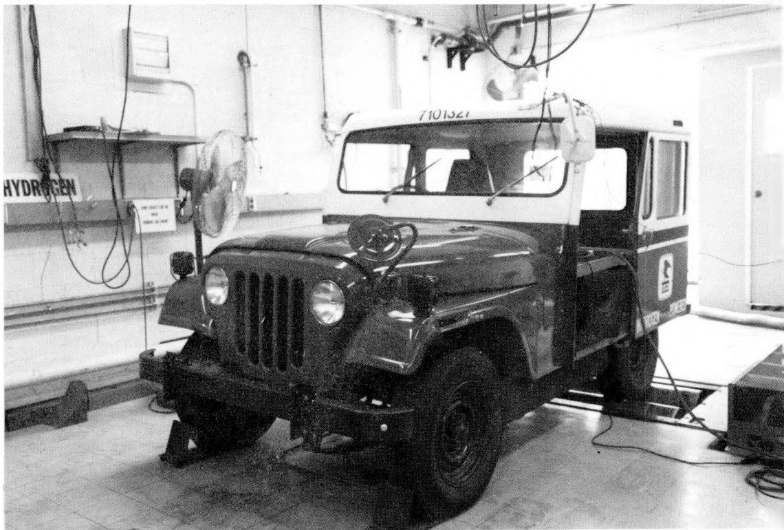
Figure 1. USPS Hydrogen-Fueled Jeep Delivery Vehicle on JPL Chassis Dynamometer
