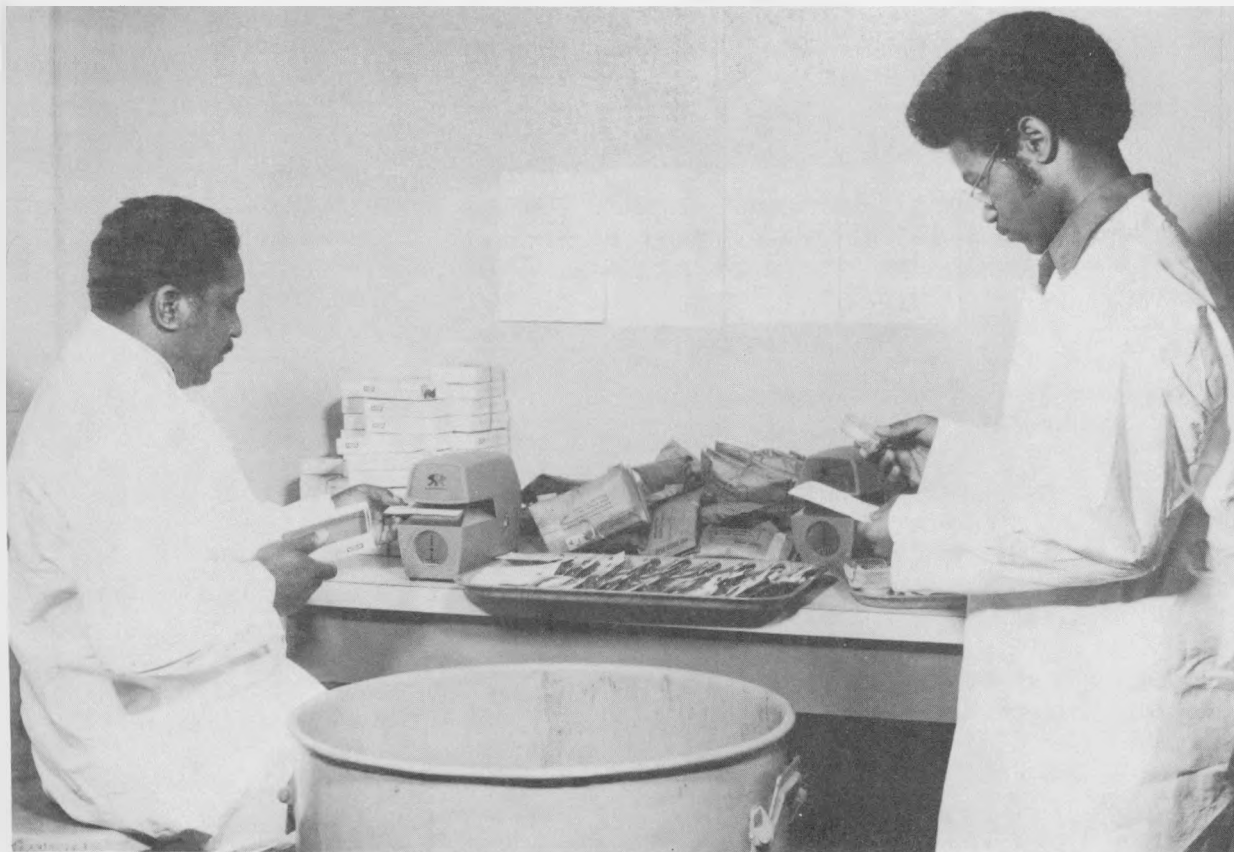
FIGURE 6. - Initial processing and marking of respirable coal mine dust samples.
