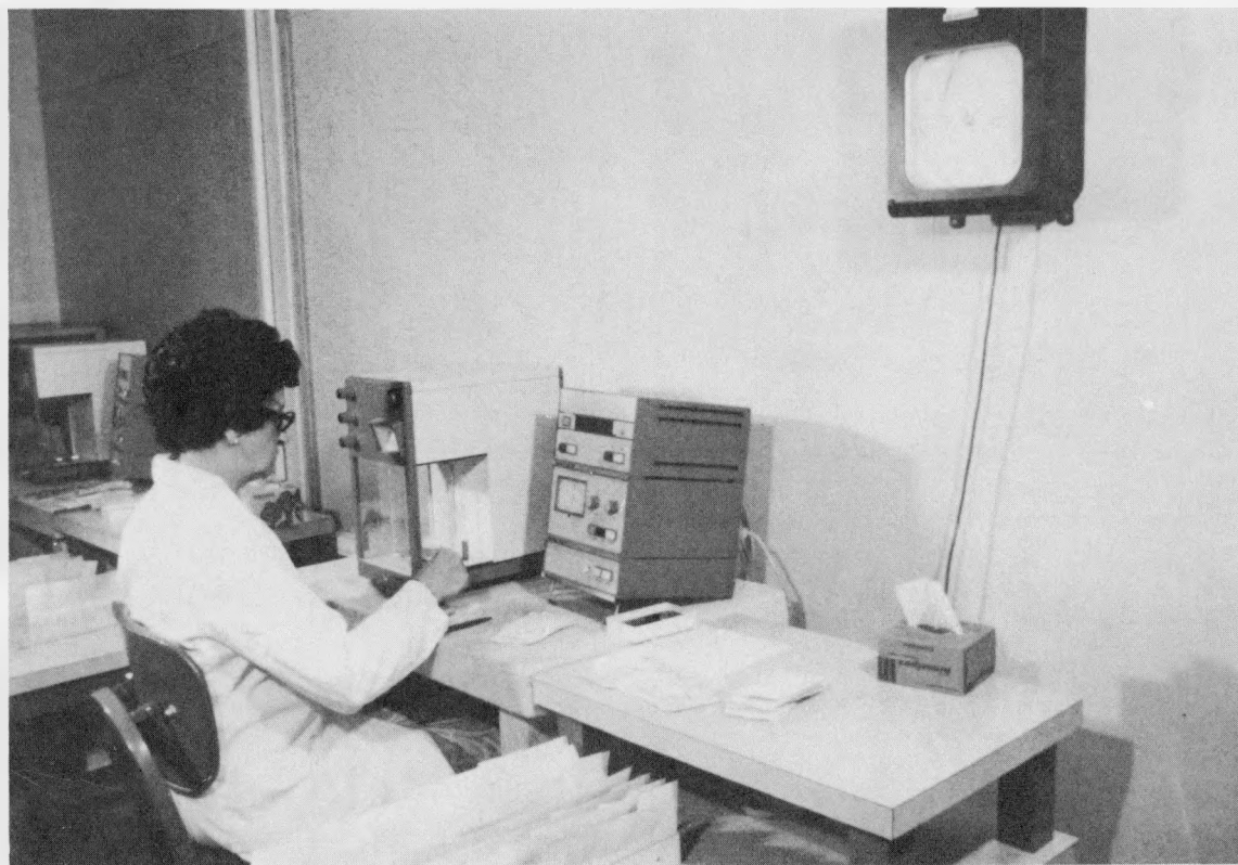
FIGURE 3. - Electronic semiautomatic balance with digital voltmeter readout (Mettler HE20).
