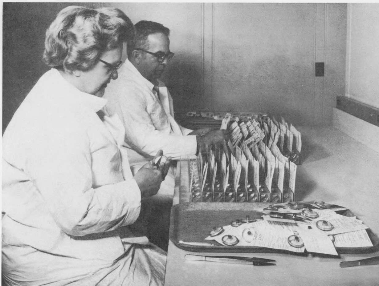
FIGURE 7. - Removal of filter capsules and filling of compartment trays.
