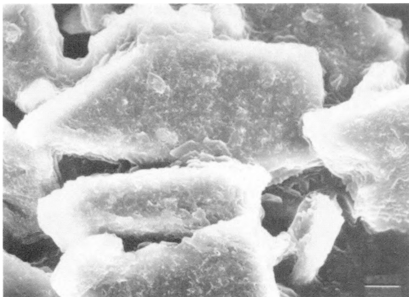
Figure 4(a): ZnO-SiC, from nitrate solution, after 15 minutes. Bar = 3.3 \mu\text{m} .
