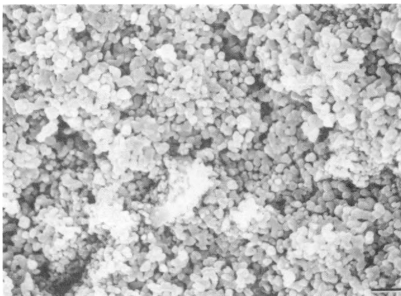
Doped matrix, 5 vol% SiC, heated to 900 °C.
