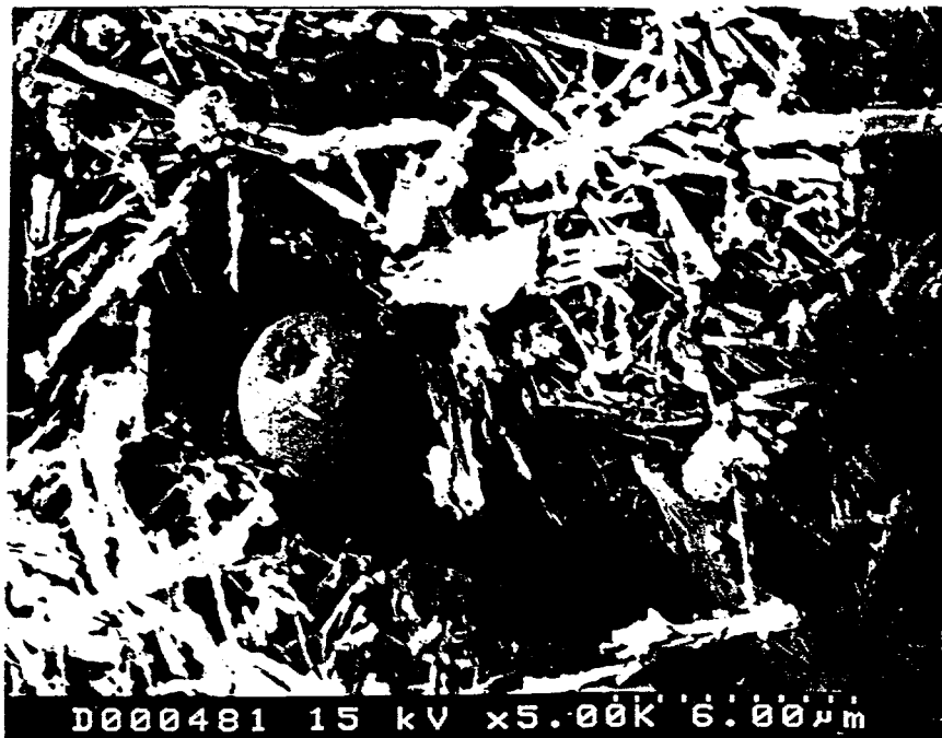
Figure 2-5b. Dense crystal growth of ettringite needles with only minimal pore space.
