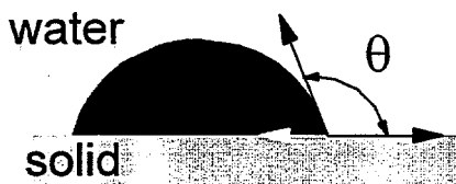
Figure 7. Contact angle is the angle between the tangent to the droplet at the three-phase line and the solid surface, measured here through the water phase.
