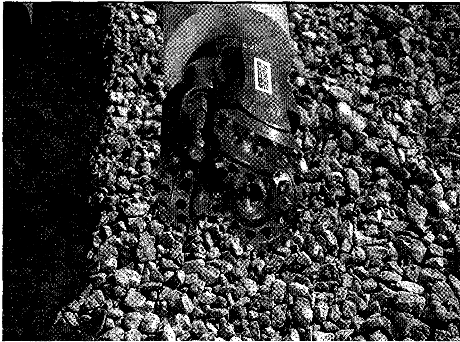
Figure 9. Smith F2 8-3/4 Inch Drill Bit with Extended UHP Nozzle used during First Field Experiment under GRI Program
