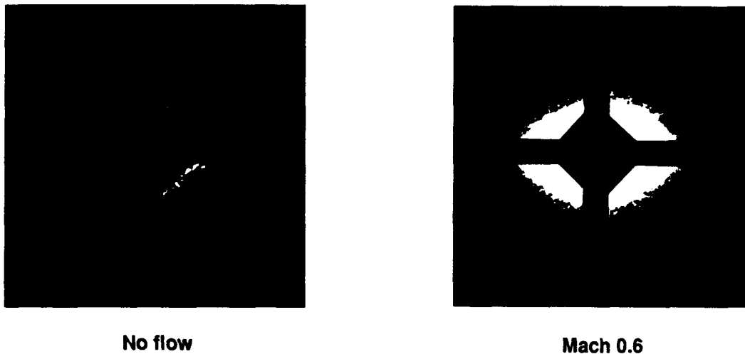
Figure 9. The intensity distribution in the focal spot. On the left is the background, on the right a flow at Mach 0.6 with no heat removal.
