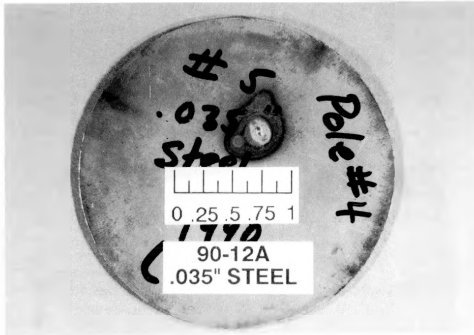
Figure 31. Back Side of Steel Sample Exposed on Flash 90-02
