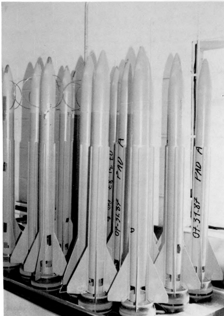
Figure 10. CENG Rocket Assemblies Prior to Installation of Propellant Cartridges (Specifications are presented in Appendix A.)
