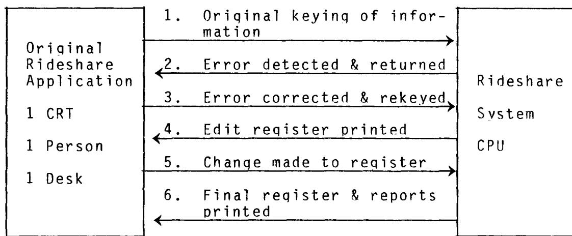
Figure 4: EXAMPLE OF CENTRALIZED DATA PROCESSING INFORMATION FLOW
