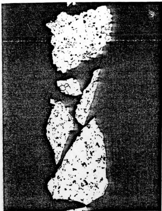
Fig. 5. As-polished cross-section of the pulverized fuel oxidized in +14.5°C dew point air at 225°C for 356 hours. Note the grain boundaries are usually seen only in etched UO 2 (250X).
