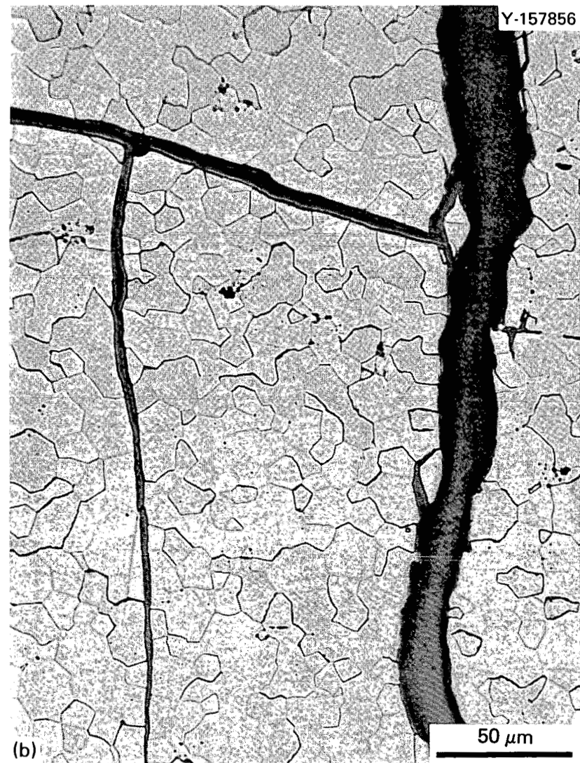
Fig. 15. Representative Microstructure of a \text{UO}_2 Pellet with High Density Matrix (Batch FGT-8, About 50- \mu\text{m} Spheres, 450°C Calcine). (a) Polished section. (b) Etched ( \text{H}_2\text{SO}_4:2\text{H}_2\text{O}_2:7\text{H}_2\text{O} ).
