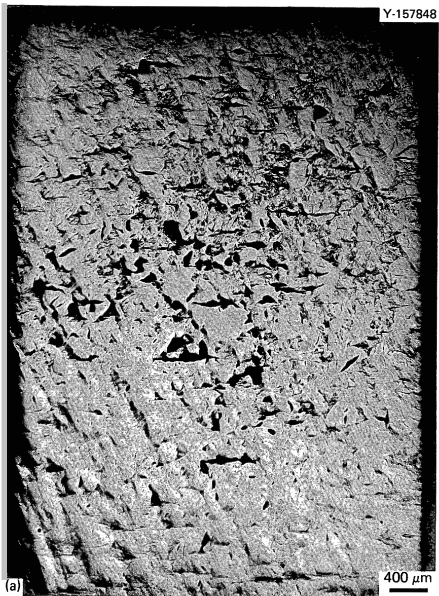
Fig. 20. A (\text{Th,U})\text{O}_2 Pellet Fabricated from SNAM-Type Microspheres (Batch MGT-104, About 700\text{-}\mu\text{m} Spheres, External Gelation-SNAM Process, \text{Th/U} = 4 ). (a) As polished. (b) Etched ( 30\text{H}_3\text{PO}_4:1\text{HF} ).
