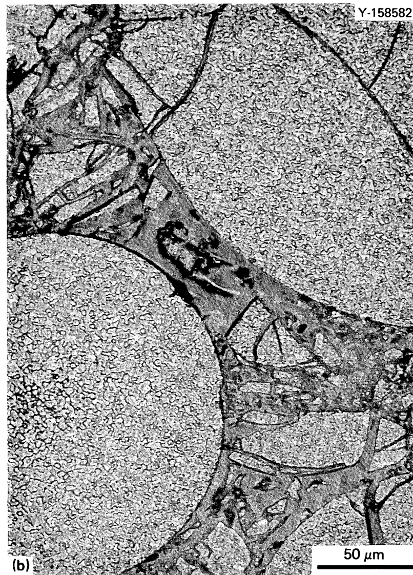
Fig. 9. A (\text{Th,U})\text{O}_2 Pellet with Remnant Microsphere Structure (Batch GT-484, About 300- \mu\text{m} Spheres, Internal Gelation, \text{Th/U} = 3 ). (a) As polished. (b) Etched (30 \text{H}_3\text{PO}_4 :1 \text{HF} ).
