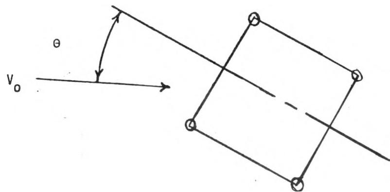
FIGURE 5 - Definition of Wind Direction
