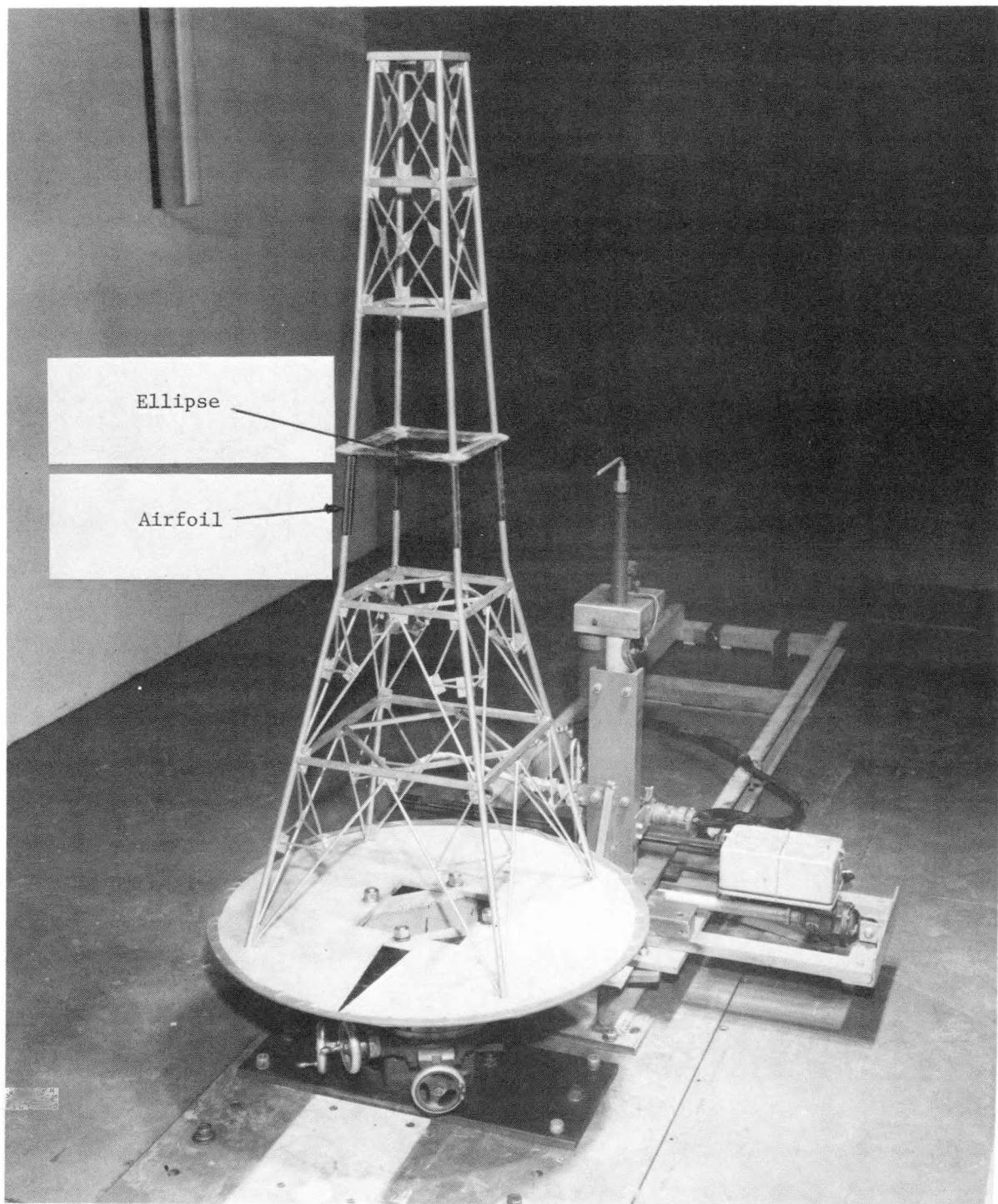
FIGURE 13 - Tower Configuration With Ellipses
