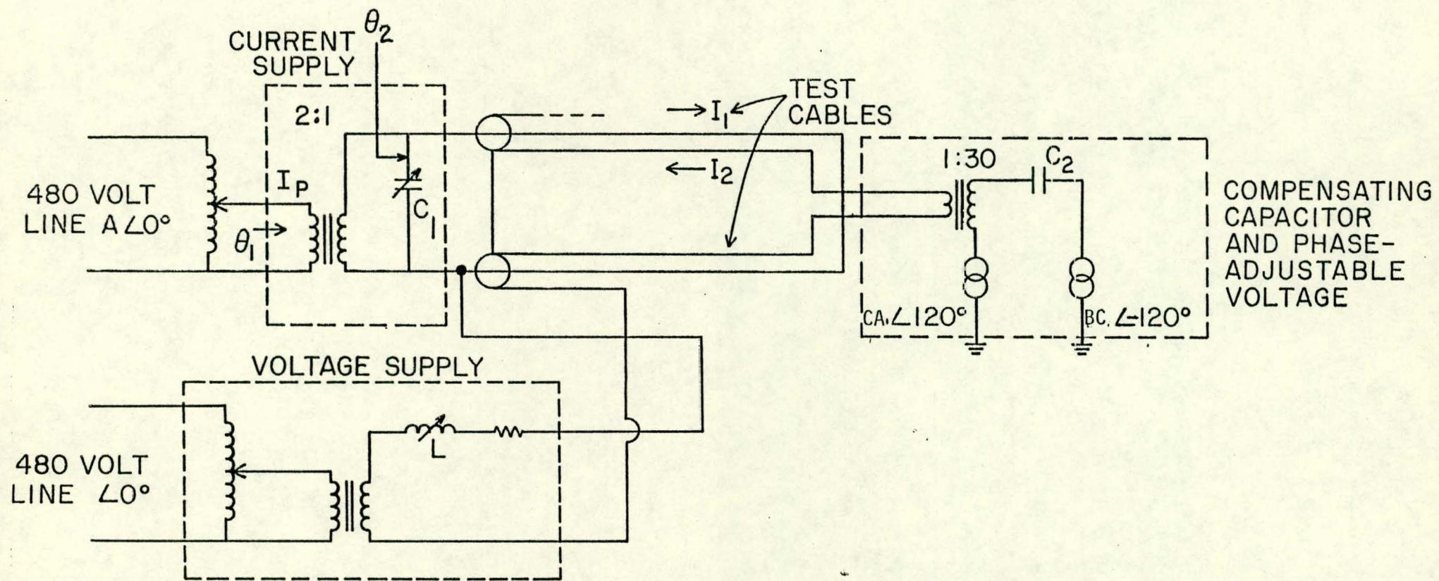
Fig. 2. Simplified model of cables and power supplies at the Test Facility.
