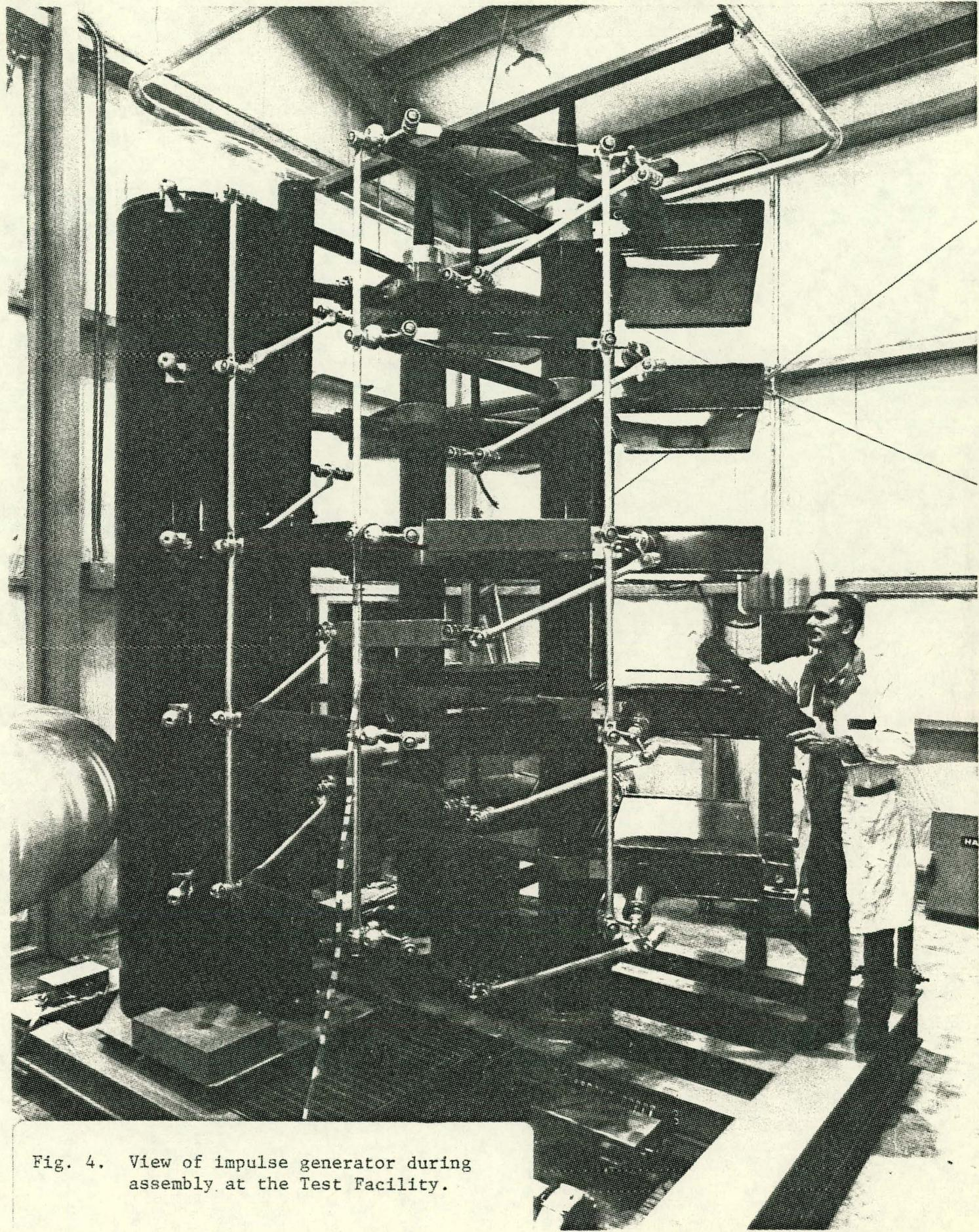
Fig. 4. View of impulse generator during assembly at the Test Facility.
