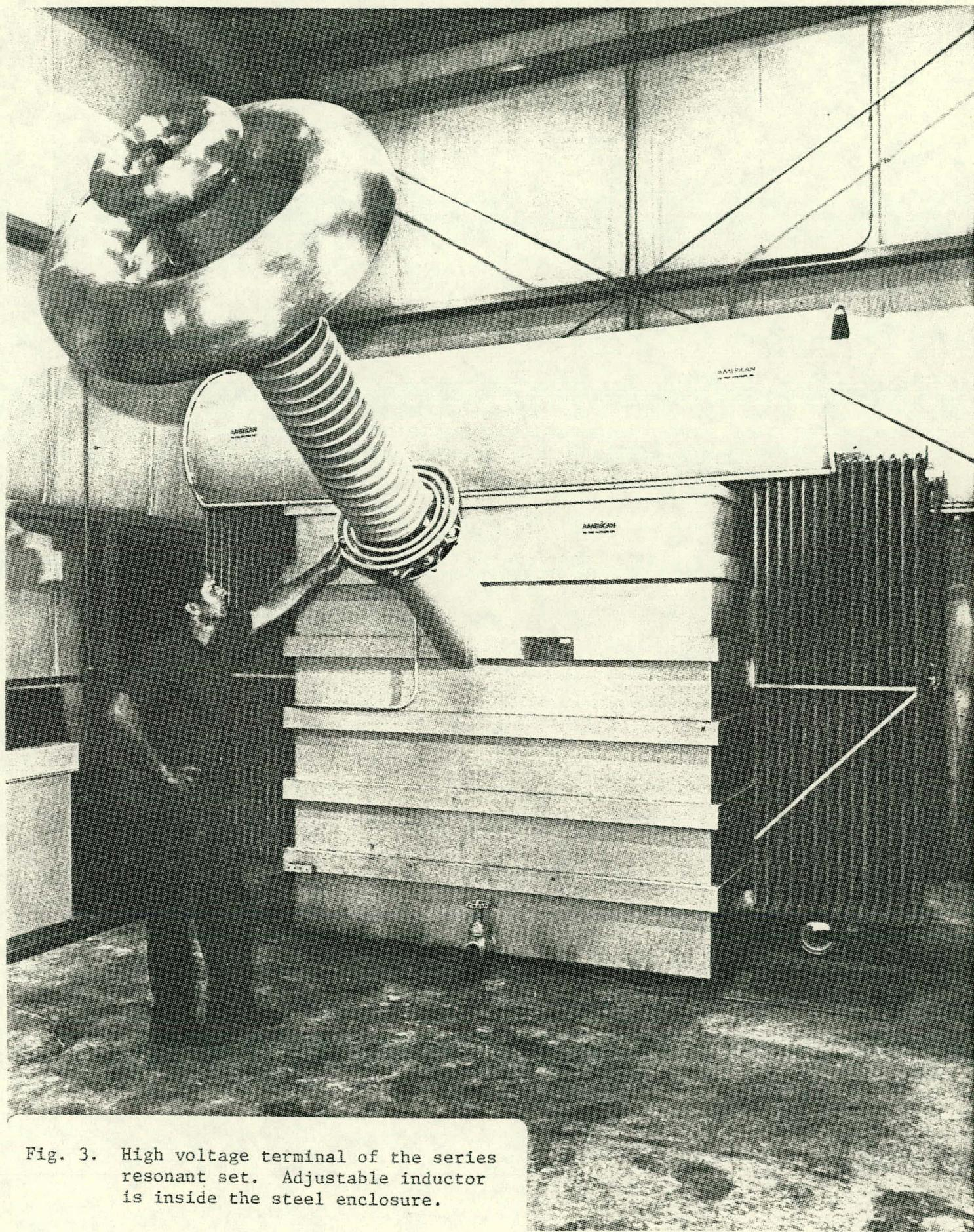
Fig. 3. High voltage terminal of the series resonant set. Adjustable inductor is inside the steel enclosure.
