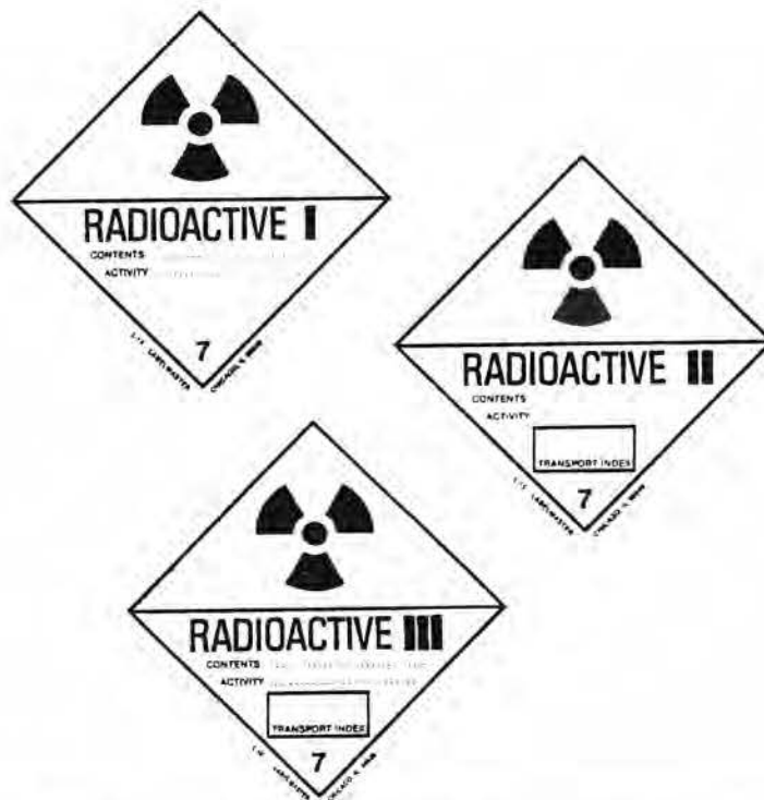
FIGURE 9.2. Warning Labels for Packages Containing Radioactive Materials
